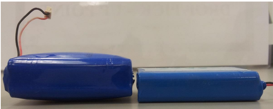
Figure 4.2 Example of battery bloat for an outdoor sensor network after 6 months (the battery is a 2.3Ah single cell Li Ion, and the average operating temperature is 118 °F).
