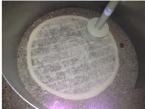
*Figure 3.2: Sand patch test on transversely tined pavement (pre-grinding)*
