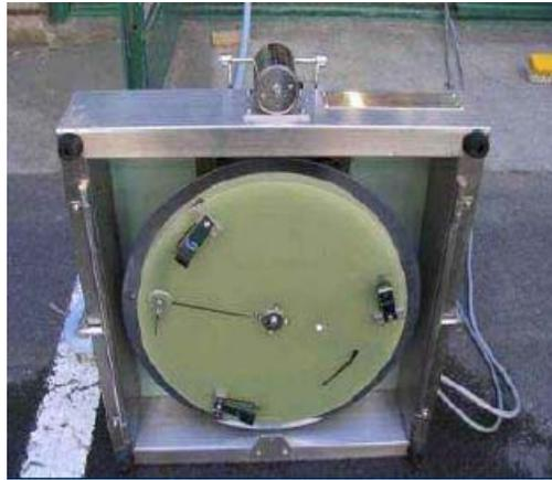
*Figure 3.4: Dynamic friction tester*
