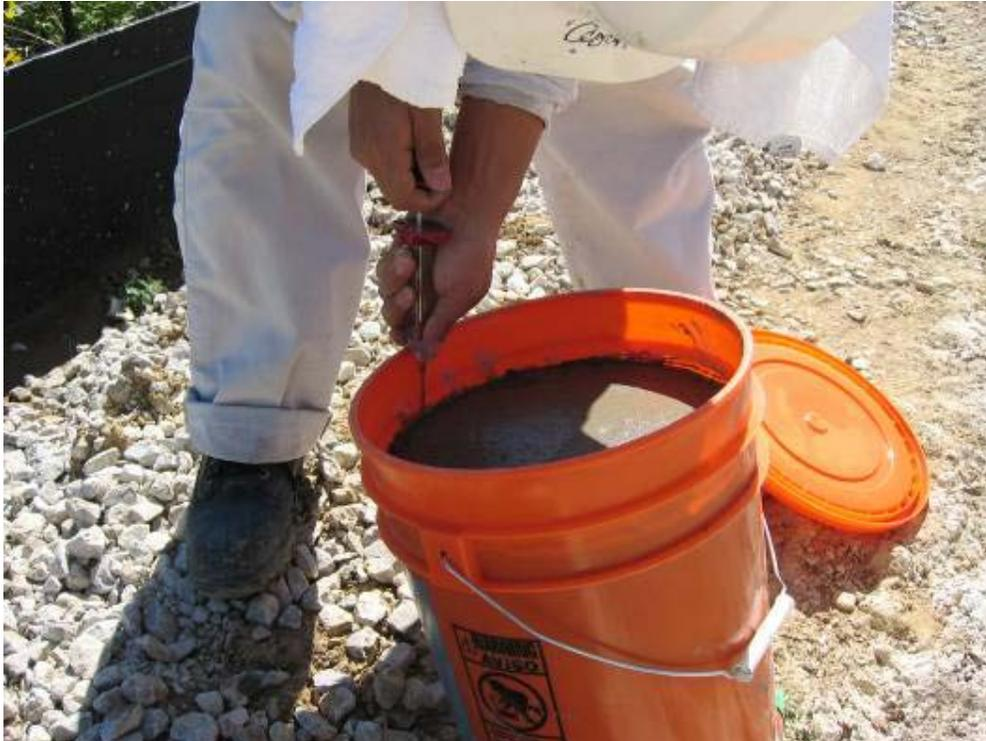
Figure 3.5: Bleeding Test of Concrete
