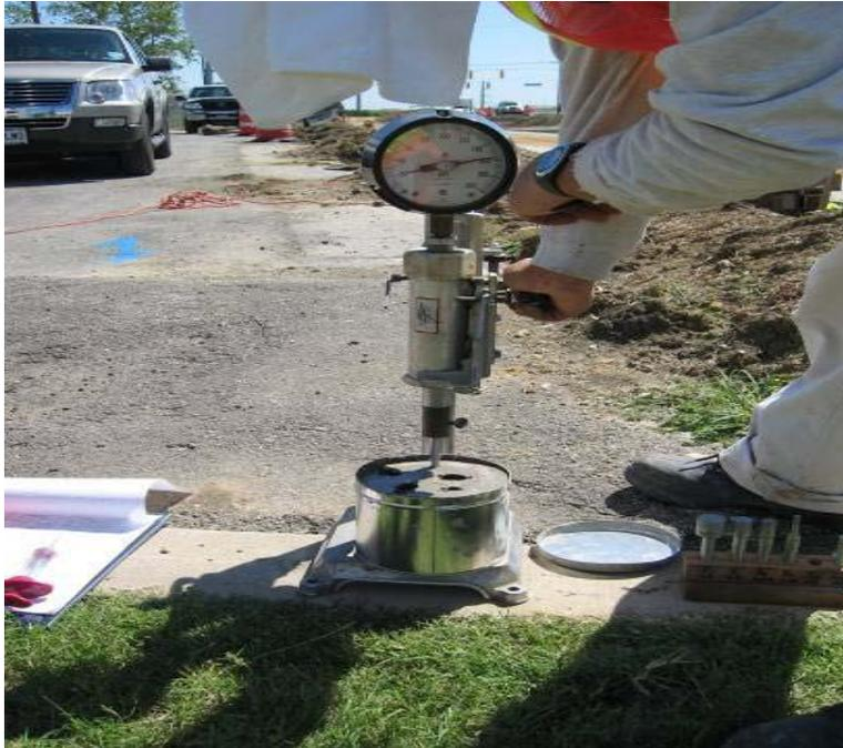
Figure 3.9: Testing for Setting Time
