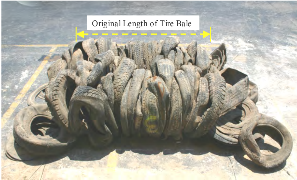
Figure 3.8 Expansion of tire bale after breakage of all wires
