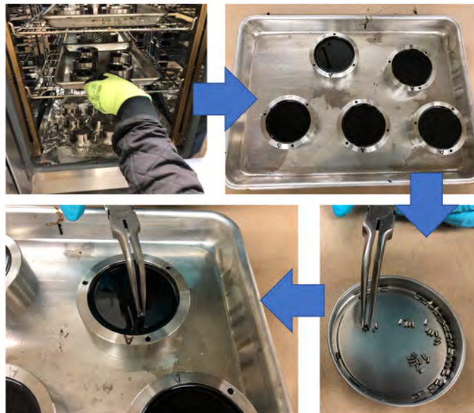
Figure A.3. Placement of dowels for film thickness control on liquid binder in the heated bottom plate of the poker chip assembly.
