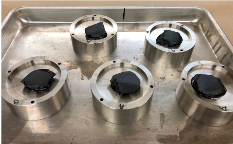
Figure A.2. Binder samples from the silicone mold placed into heated bottom plate of the poker chip assembly.
