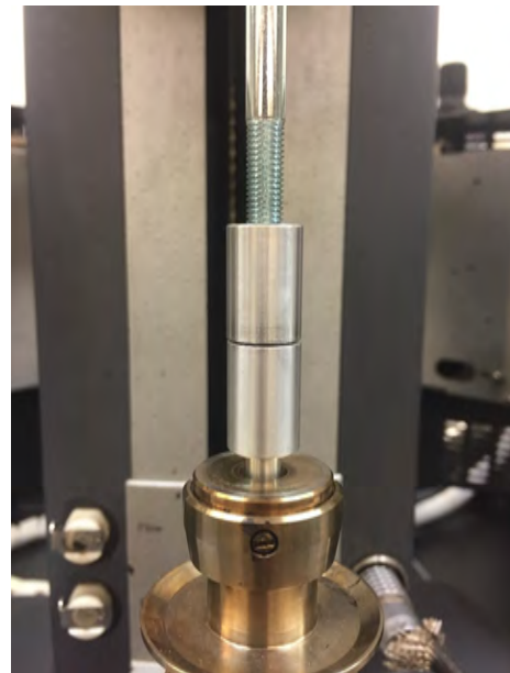
Figure 3.6. Sixth iteration that required the use of DSR to achieve temperature control, maintain alignment and precise film thickness in the sample.
