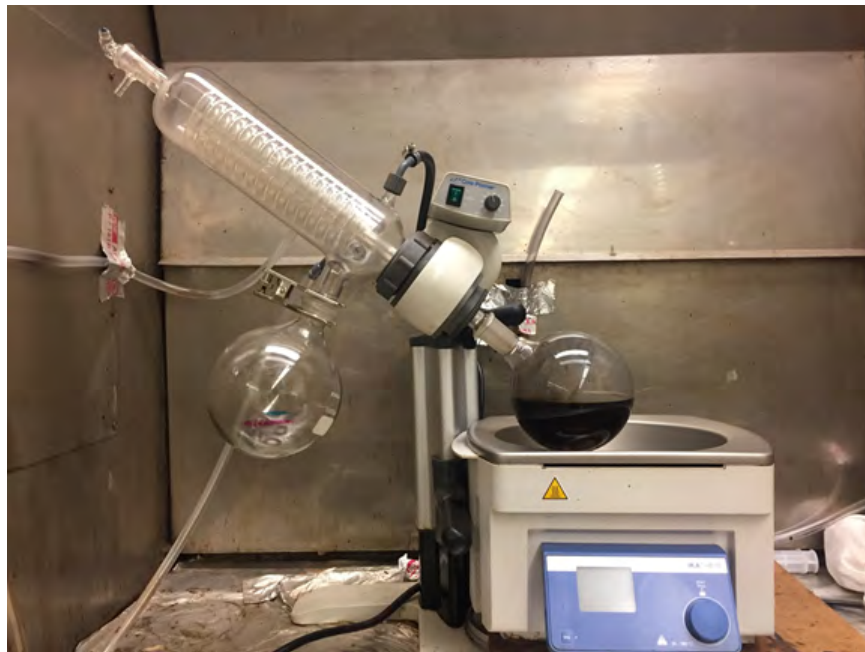
Figure 2.6. Rotary evaporator used to recover the asphalt binder.
