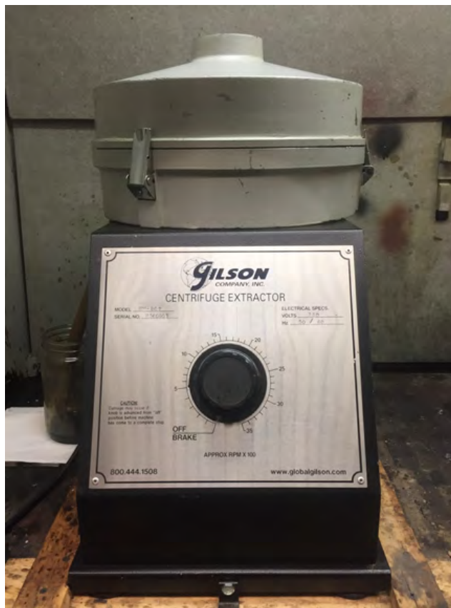
Figure 2.5. Centrifuge extractor used with toluene as the solvent to recover the asphalt binder.
