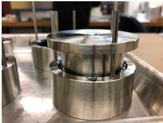
Figure A.6. Side of the poker chip assembly after placing the top plate and alignment pins.
