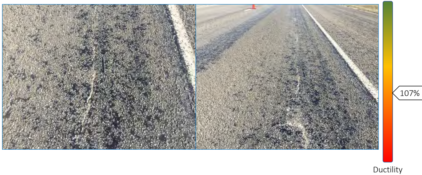
Section #8: 7 years Photo and coring from Dec. 2019, a seal coat was placed prior to coring but cracks bleeding through are visible
