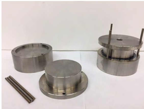
Figure 4 – Poker chip stainless-steel mold and laboratory-molded specimen between the top and bottom pieces that are aligned using three alignment pins (top and bottom of the mold with the three alignment rods are shown to the left and an assembled mold with the binder sample is shown to the right).
