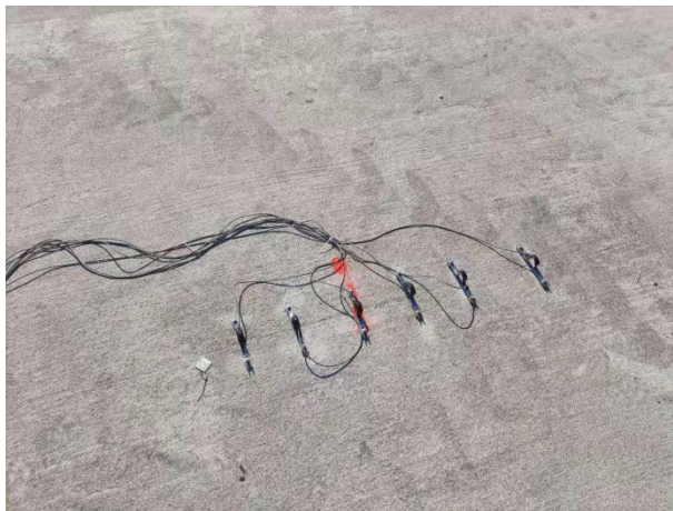
(a) Pi-gage on Deck Surface
