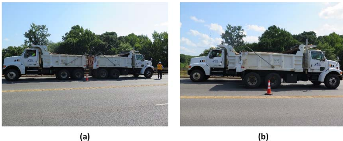
Figure 6.15 Photographs of (a) Back-to-Back Loading Configurations and (b) Side-by-Side Loading Configurations
