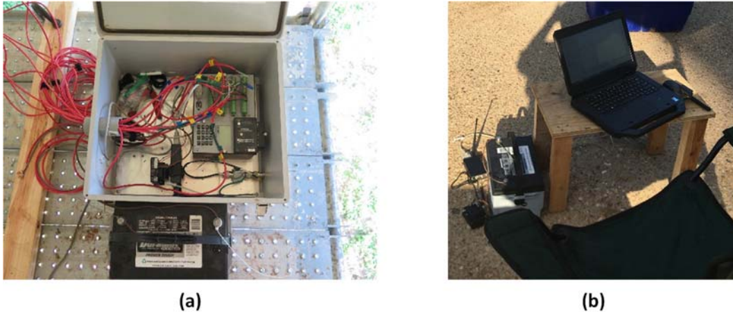
Figure 6.6 Data Acquisition System – (a) Datalogger and (b) Laptop Computer
