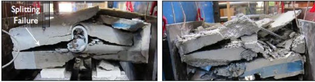
Figure 4.19 Splitting and Crushing Failure Mechanisms of Panel-Based Specimens (Wald et al., 2017)
