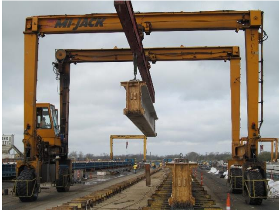
Taking off girders from prestressing bed
