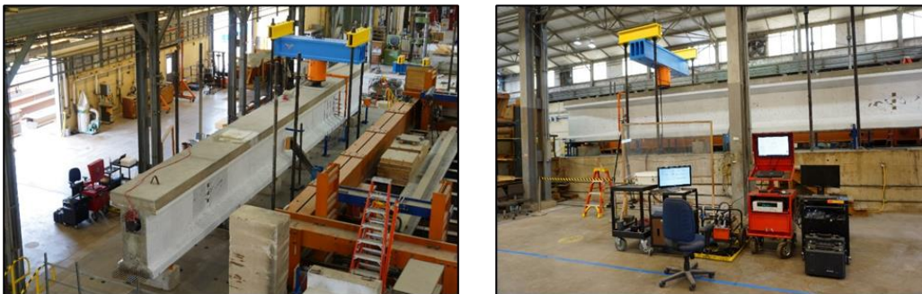
Figure 4.2 As-Built Structural Schematic: (a) Overall Structural Setup with the Test Specimen and (b) Designed Monitoring and Controlling Area during the Test
