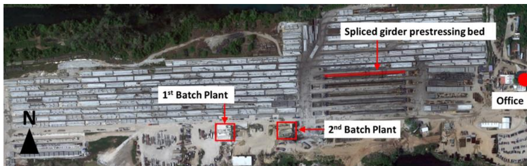
Figure 3.5 Precast Plant with the Location of Prestressing Beds and Batch Plants
