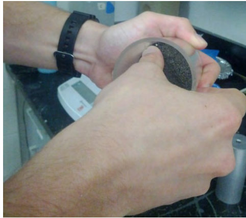
Figure 3: Densification of Soil Using Thumb
