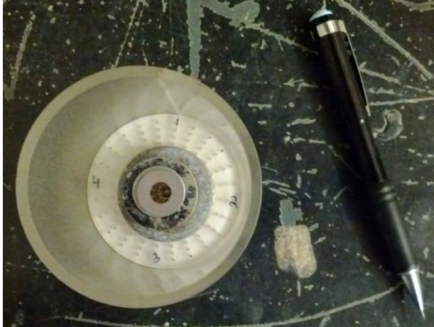
Figure 7: Assembled Permeameter Cup with Overburden Washers and Washers Simulating 51.3 Grams of Overburden from the Ponded Water
