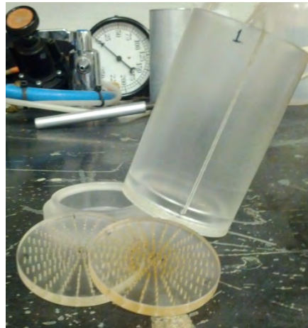
Figure 1: Components of Plastic Permeameter Cup: Top Cup, Cup Base, and Porous Disks
