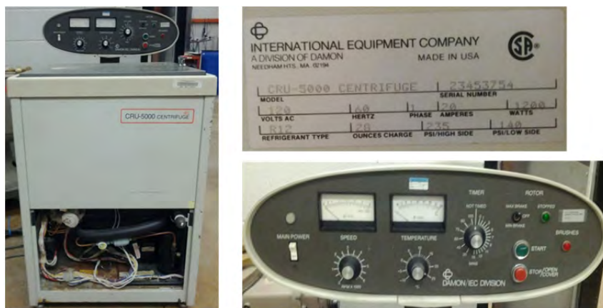
Figure 3.1: Damon IEC CRU-5000 Centrifuge and Control Board
