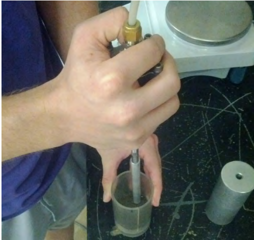
Figure 4: Compaction of Soil Specimen Using Small Diameter Kneading Compactor
