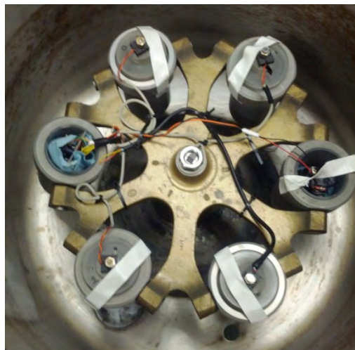
Figure 8: Assembled Testing Setup within the Centrifuge
