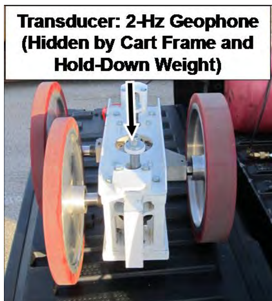
(b) Photograph of Rolling-Sensor Three-Wheel Cart
