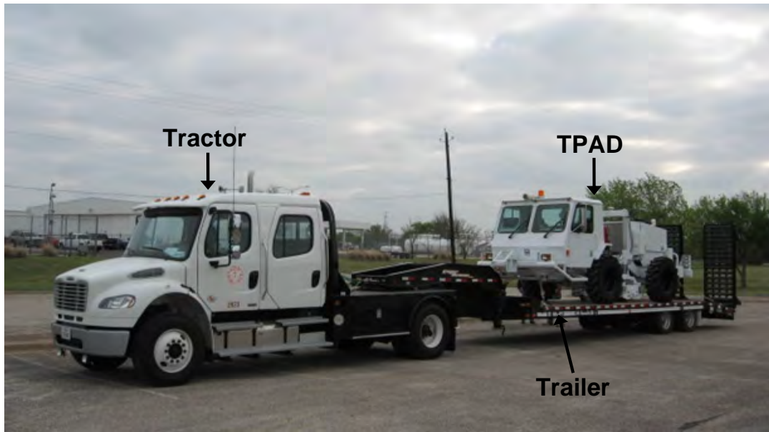
(a) Photograph of the TPAD on the Tractor-Trailer Rig
