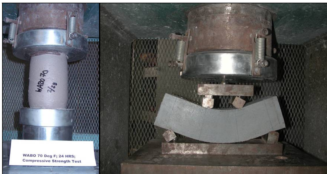
Figure A14. Flexible materials are typically too easily deformed to test under concrete test methods. This material is still within elastic limits.
