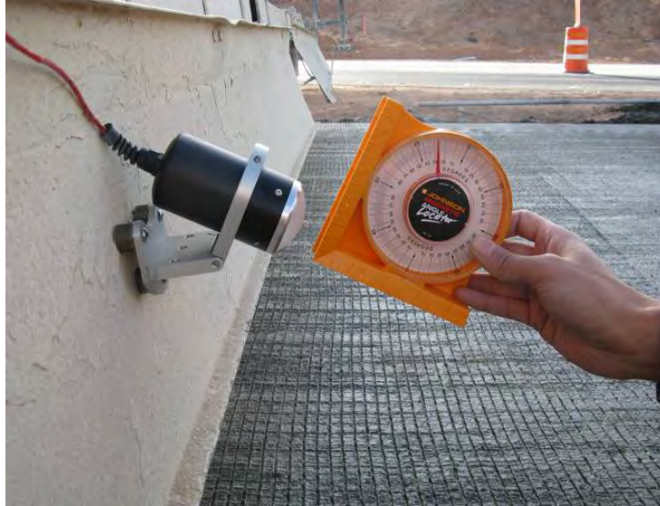
Figure 2.1: NDRSS retrofitted in curing machine
