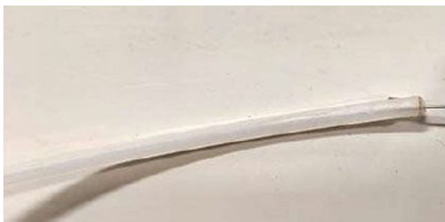
Figure 46. Stainless steel tell-tale wire and white nylon plastic tubing
