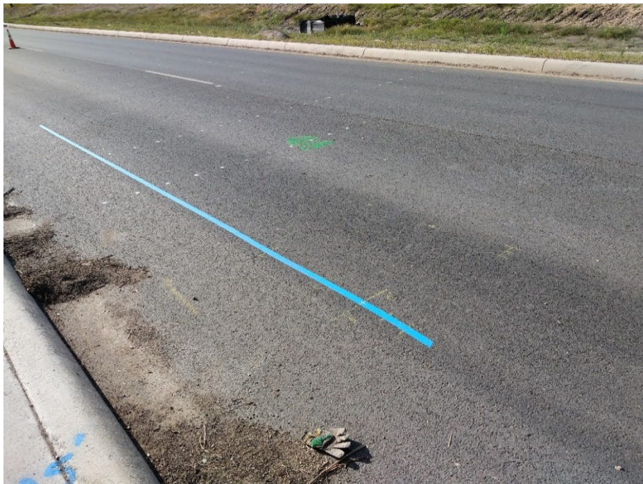
Figure 75. Photo showing location of sensors marked in yellow and wheel path highlighted in blue to facilitate accurate trafficking of instrumented sections
