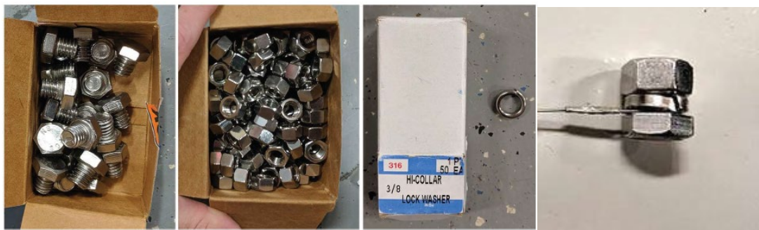
Figure 45. Components of gravel D50 simulant (from left bolt, nut, washer, assembled simulant)
