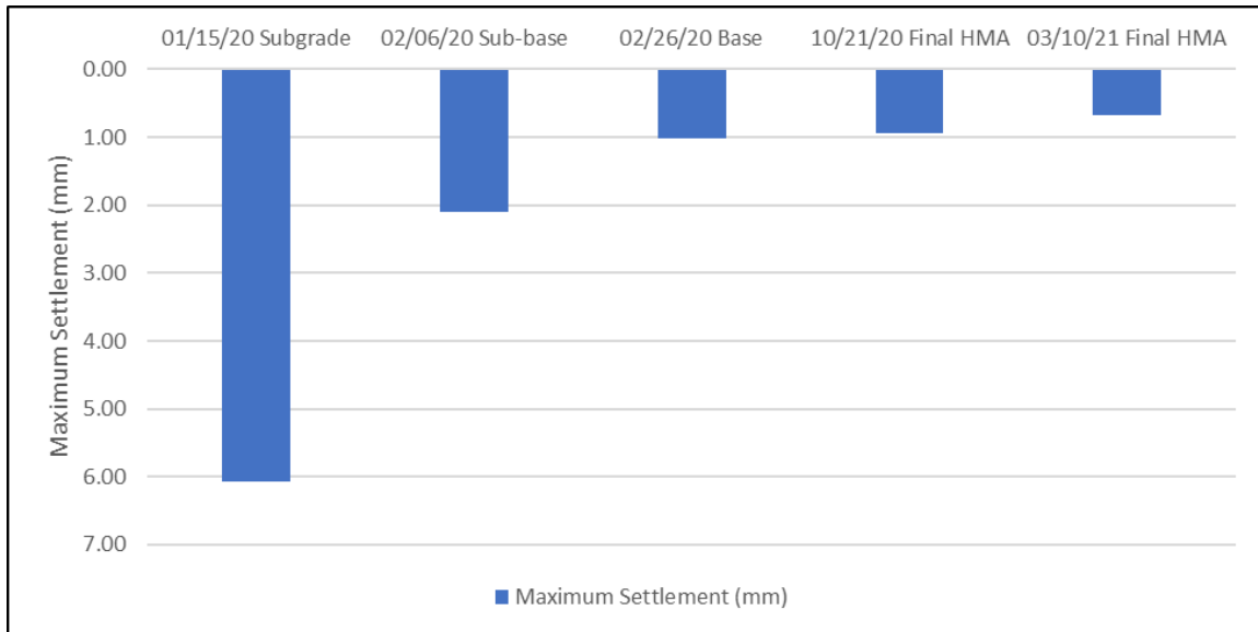
Figure 104. Maximum settlement under sPLT
