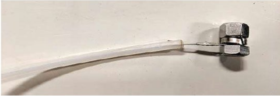
Figure 58. Tell-tale attached to gravel simulant
