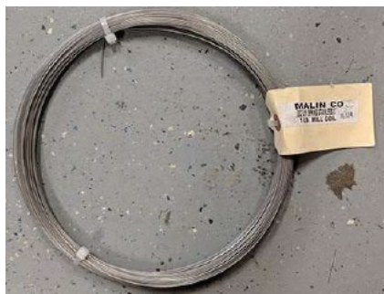
Figure 46. Stainless steel tell-tale wire and white nylon plastic tubing
