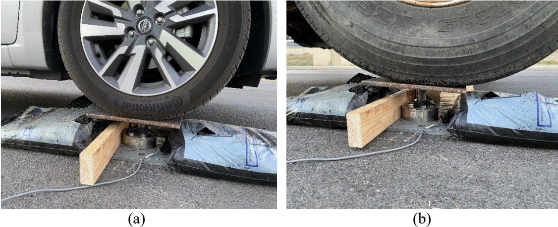
Figure 76. Custom scale used to weigh wheel load of: (a) light car; and (b) heavy truck
