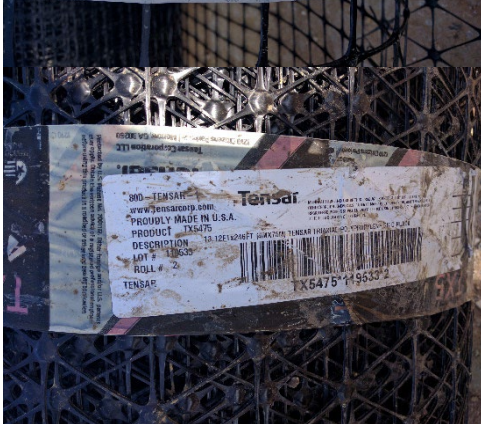
Figure 27. Geosynthetic samples collected from various IH10 test sections: a) geogrid type II from WBFR test section; b) geogrid type I from EBFR test sections; c) geogrid type II from EBFR test sections; and d) geogrid type III from EBFR test sections
