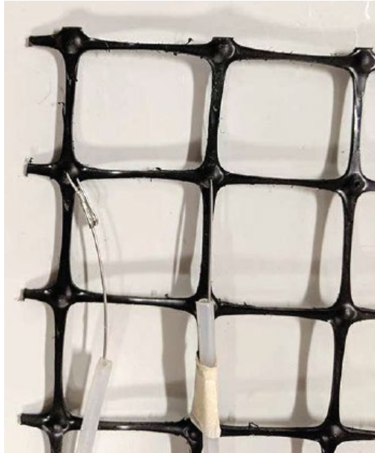
Figure 57. Tell-tale installed on a geogrid node
