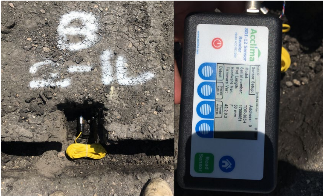
Figure 159. TDR installed in section 2 and connected to data logger
