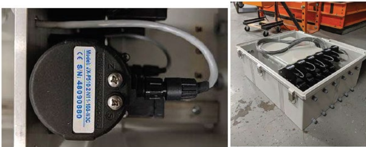
Figure 59. LP mounted on a vertical aluminum plate installed inside the enclosure box
