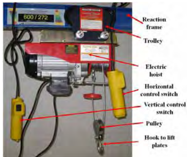
Figure 2.3: Automated hoist system used to assemble the reaction frame.
