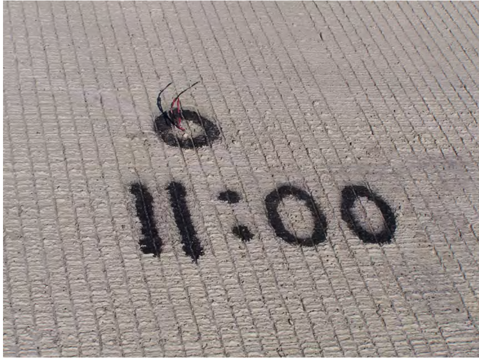
Figure 3.3 Wires from Installed I-Button Assembly
