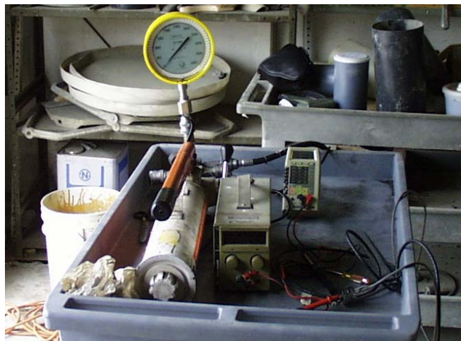
Figure 4.19: Hand Pump and Load Cell Output
