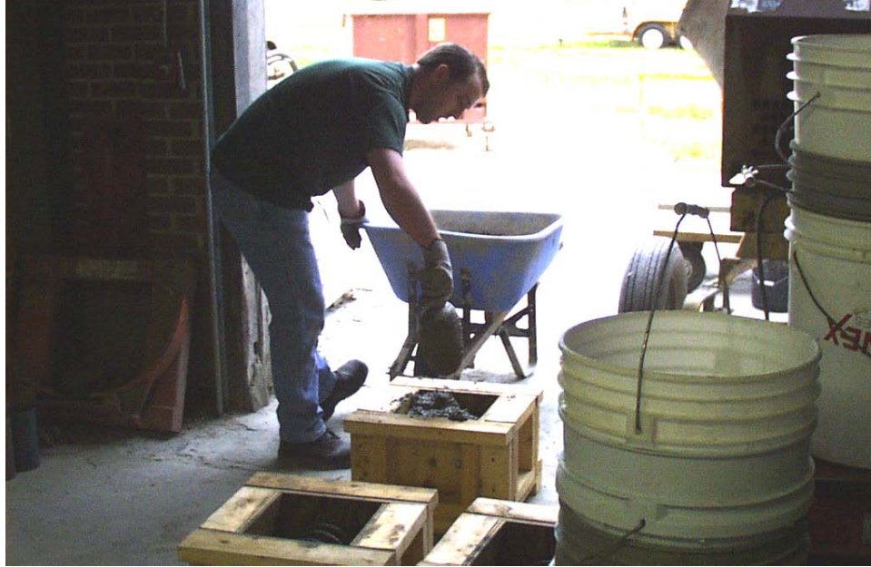
Figure 4.11: Concrete Placement for Pullout Specimens
