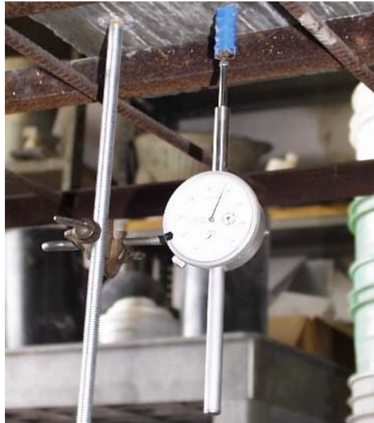
Figure 4.20: Slip Measured by Linear Displacement Gauge
