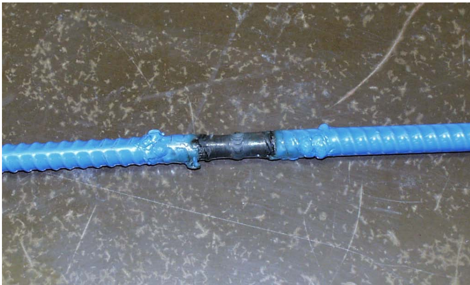
Figure 4.7: Typical Nylon-Coated Bar Weld
