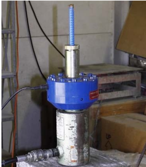
Figure 4.18: Hydraulic Ram, Load Cell, and Grips
