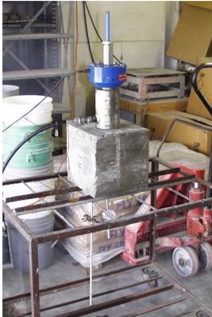
Figure 4.21: Complete Pullout Test Loading Setup
