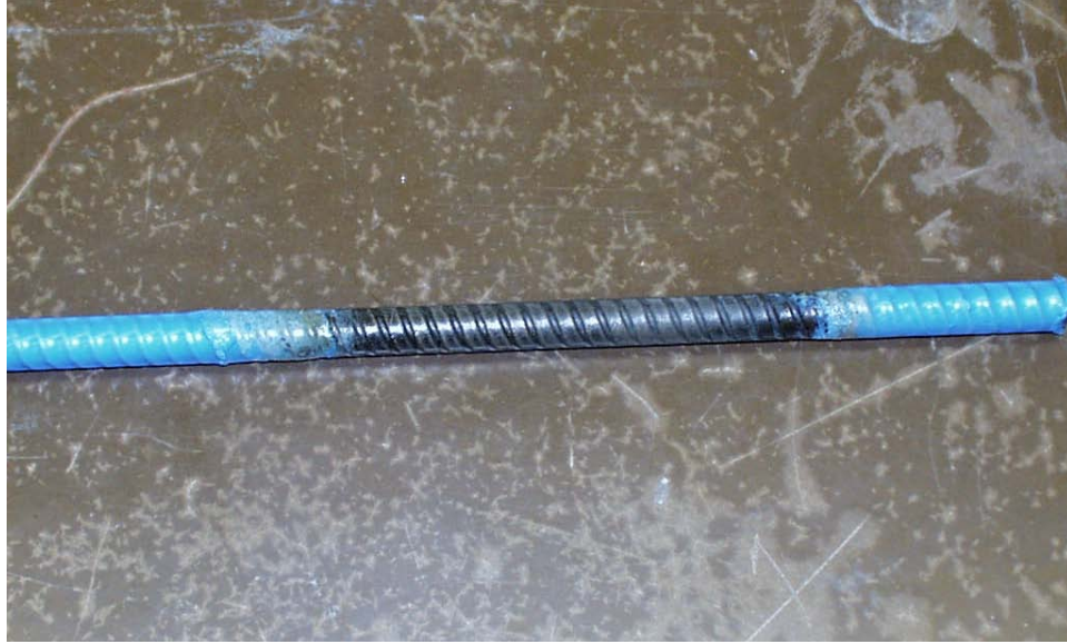
Figure 4.8: Nylon Coating Removed for Control Specimens
