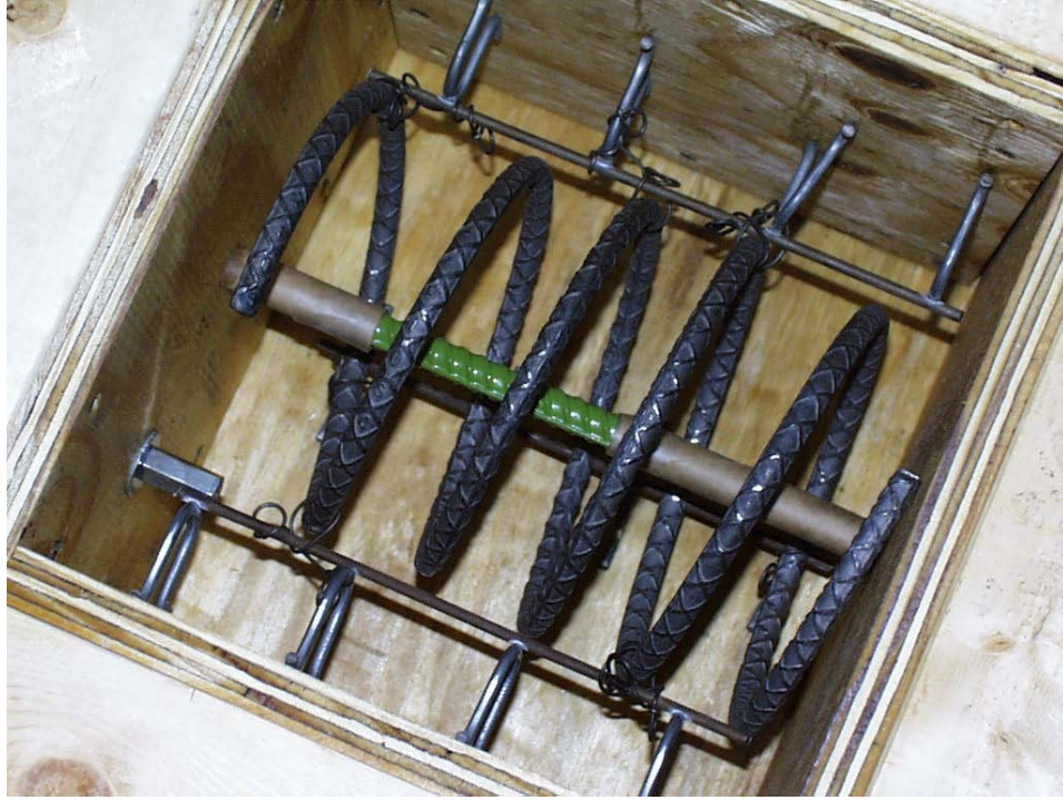
Figure 4.10: Typical Reinforcing Steel and Test Bar Setup
