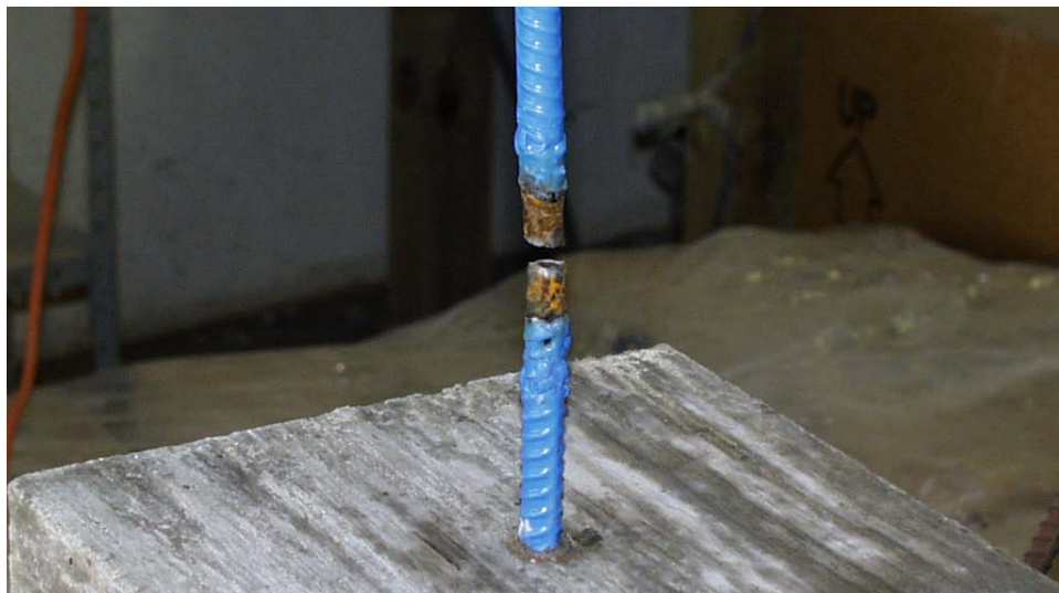
Figure 5.6: Typical Nylon Weld Fracture
