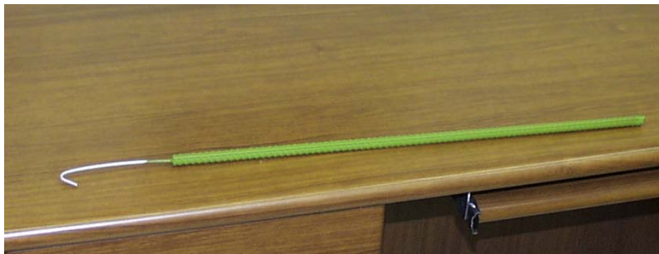
Figure 4.5: Typical PVC-Coated Bar
