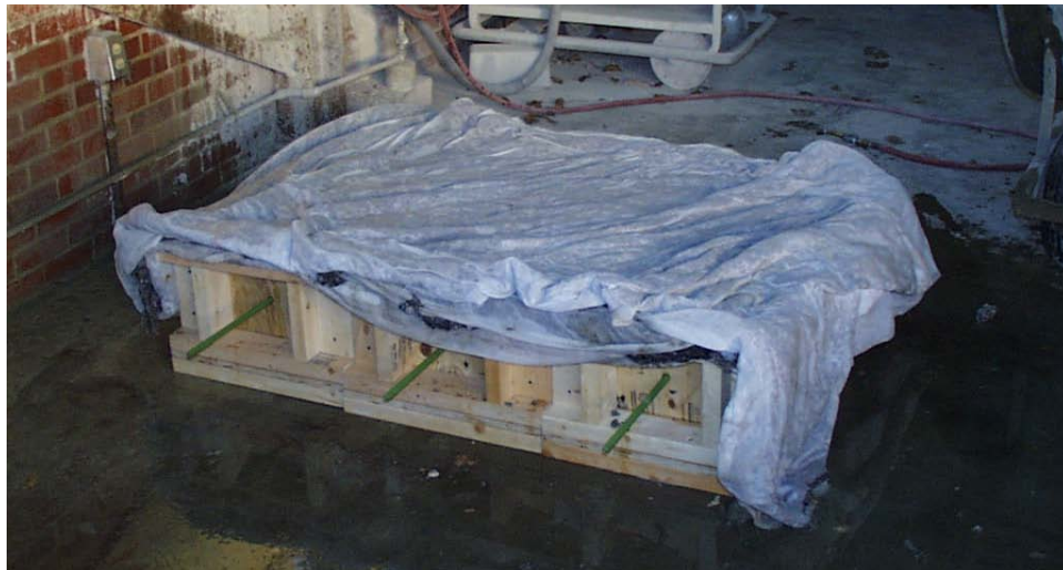
Figure 4.13: Curing of Pullout Specimens
