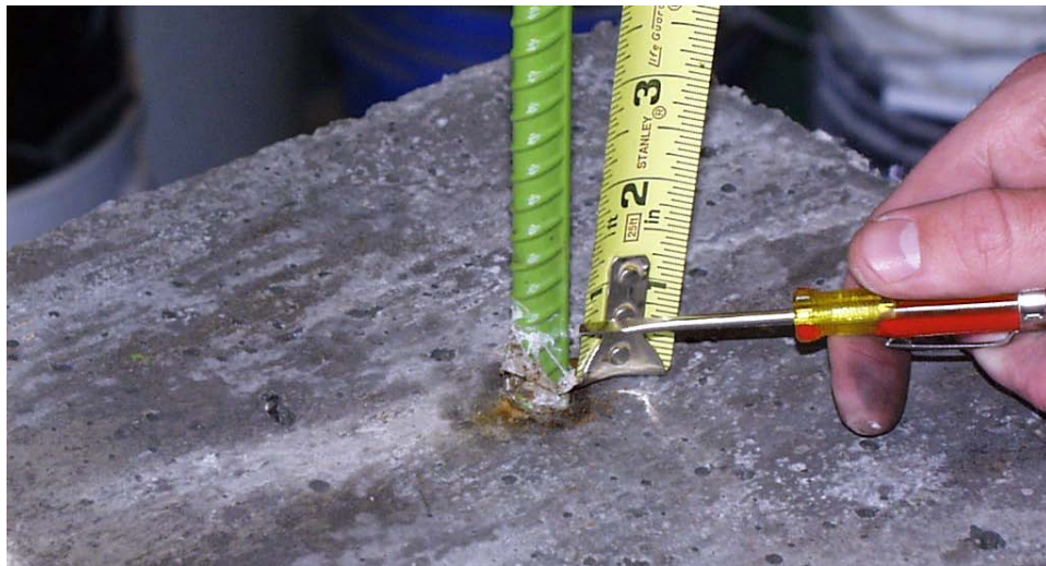
Figure 5.4: Typical PVC Pullout Failure
