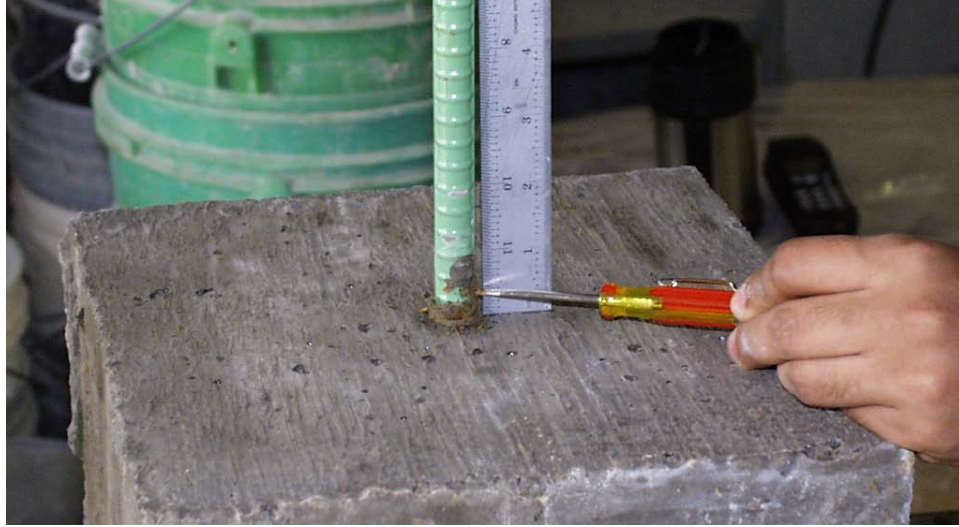
Figure 5.5: Typical Epoxy Pullout Failure
