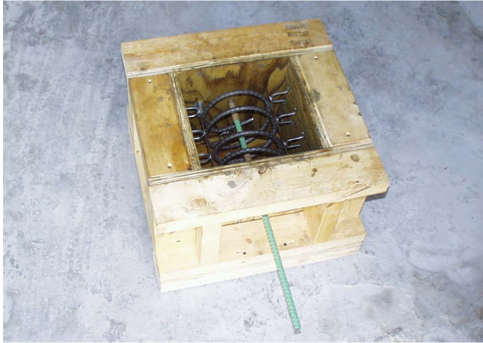
Figure 4.9: Typical Form for Pullout Specimens
