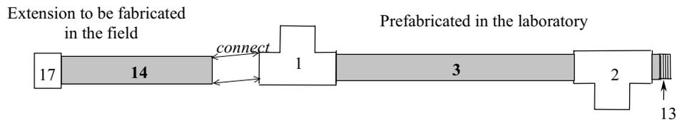
*Figure 2.13 External assembly for the bubbler orifice*
