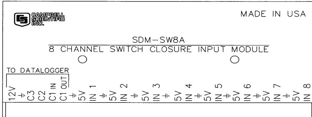
Figure 3.22 Connection panel of the SDM-SW8A switch closure module
