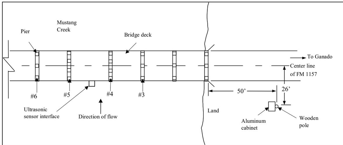
*Figure 1.1 Plan view of the proposed installation*
