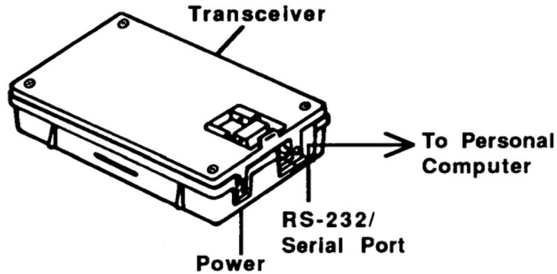
*Figure 2.25 Connection between transceiver/modem combination and computer*
