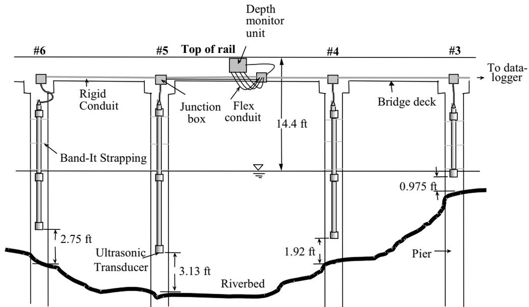
Figure 2.14 Layout of the completed installation
