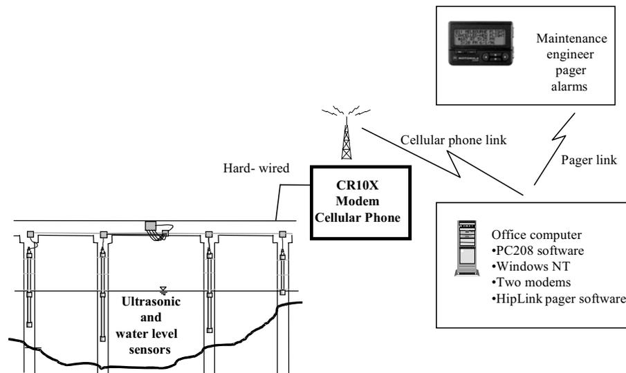
*Figure 3.14 Communications schematics for the Phase II installation*
