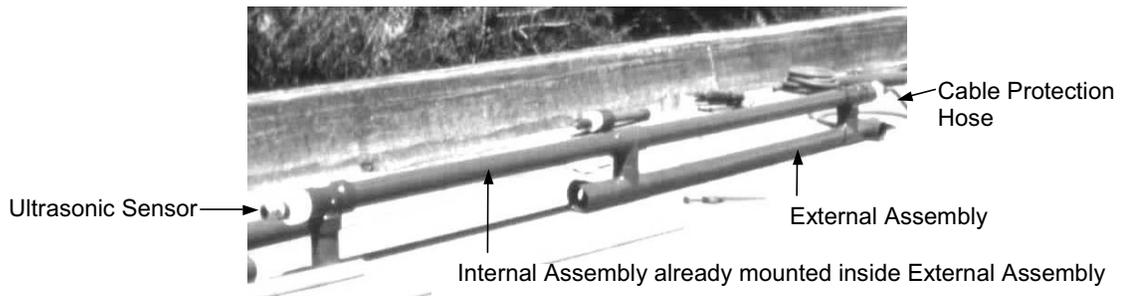
*Figure 2.14 Sensor assembly ready for strapping to piers*
