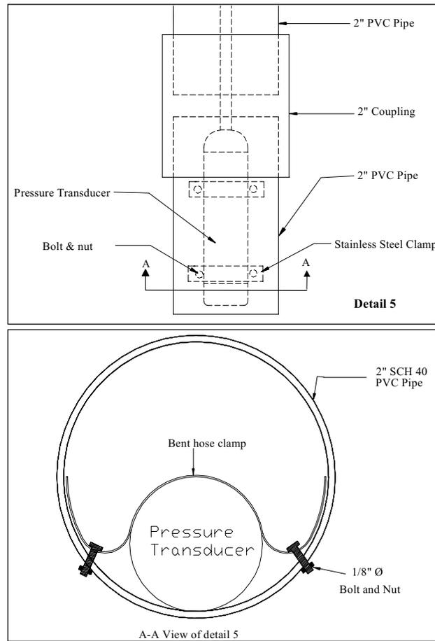
Figure 3.8 Schematics of the pressure transducer assembly (Detail 5)
