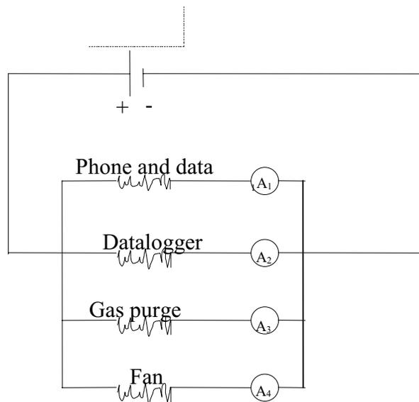
*Figure A.1 Schematics for measuring amperage consumption of equipment*
