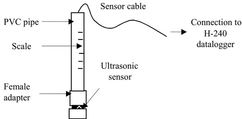
*Figure 2.2 Temporary ultrasonic sensor assembly*
