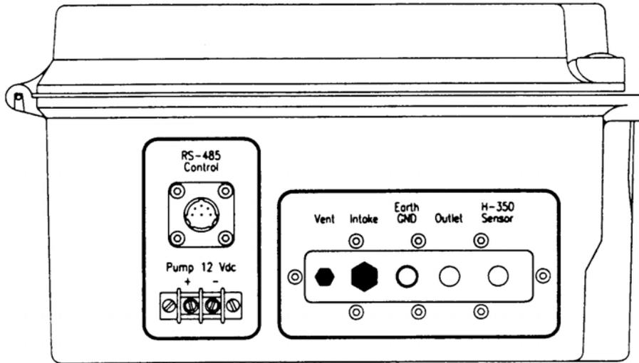
Figure 2.20 H-355 Connector panel
