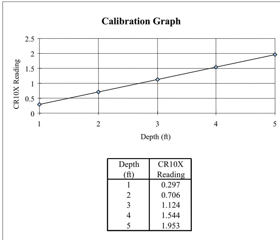
*Figure 3.10 Calibration curve for the pressure transducer*
