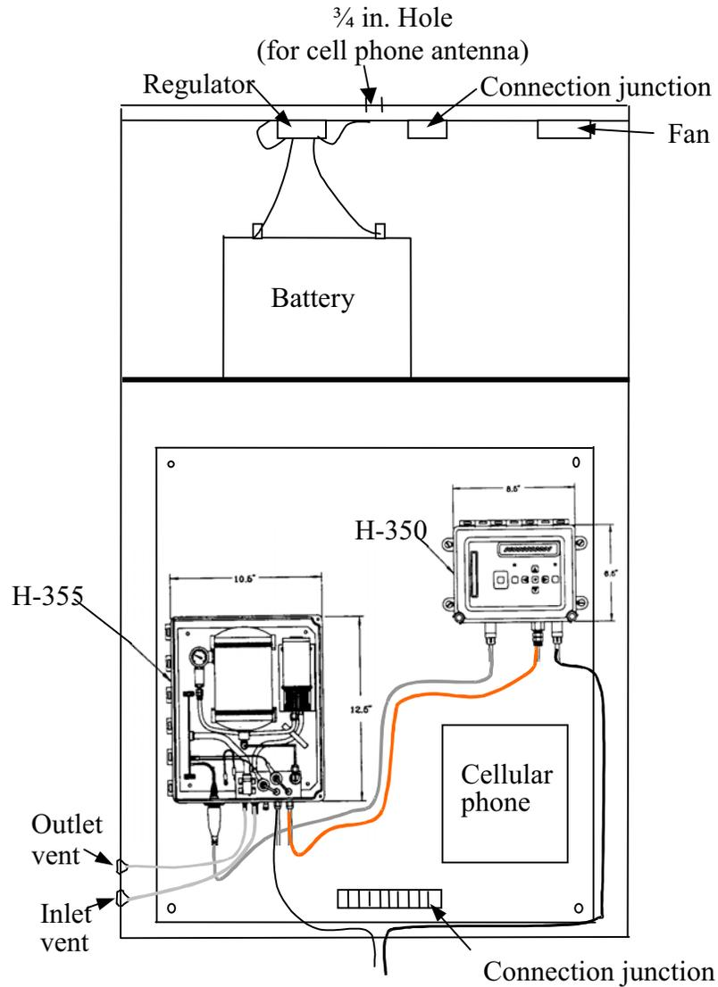
*Figure 2.5 Plan view for the main electronics box with units layout*
