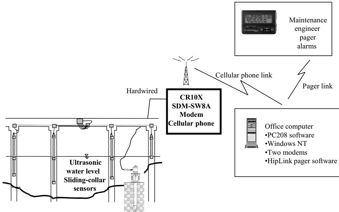
*Figure 3.24 Schematics of a hybrid magnetic sliding-collar ultrasonic installation*
