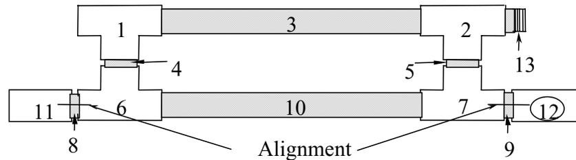
*Figure 2.7 Schematics of prefabrication of transducer external assembly*
