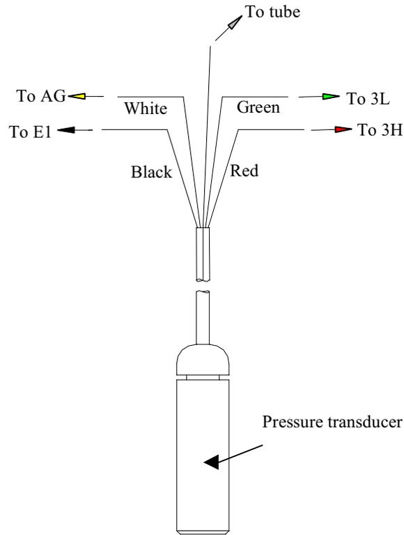
Figure 3.9 Wiring schematics for the pressure transducer
