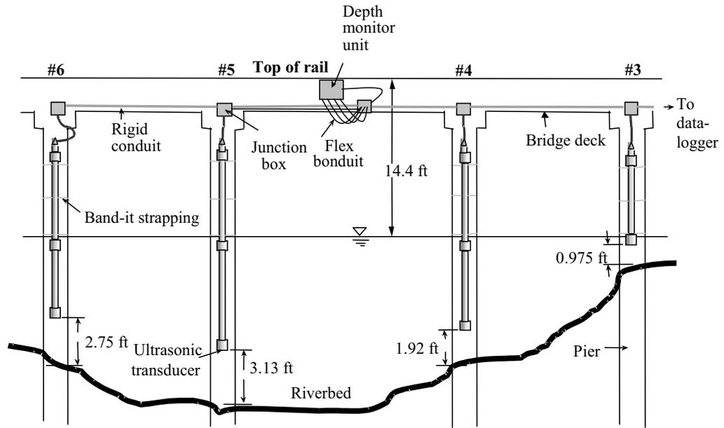
*Figure 1.2 Elevation of the proposed installation viewed from upstream.*
