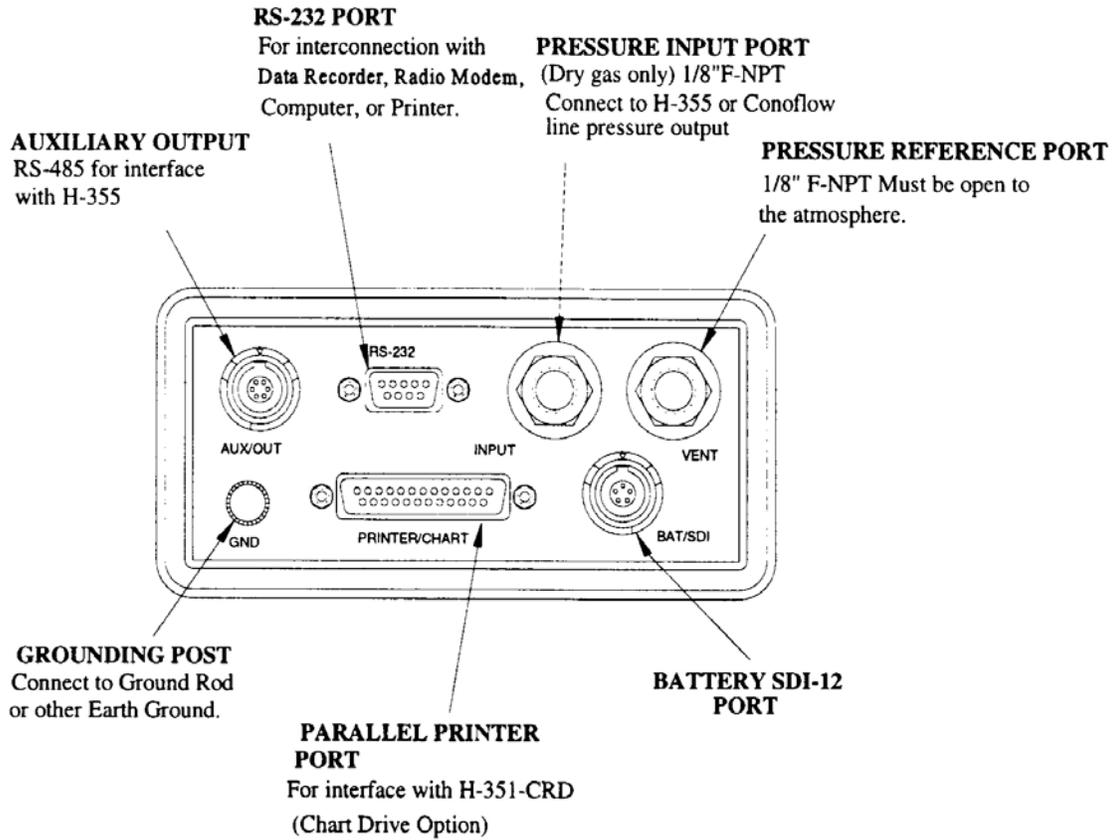
Figure 2.19 H-350 Connector panel
