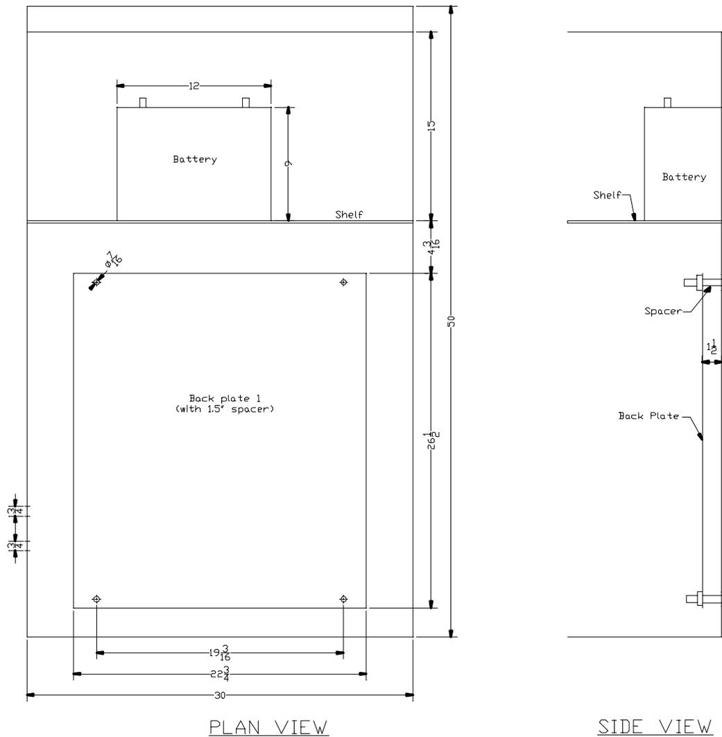
*Figure 2.4 Plan and side views for the main electronics box (dimensions in inches)*
