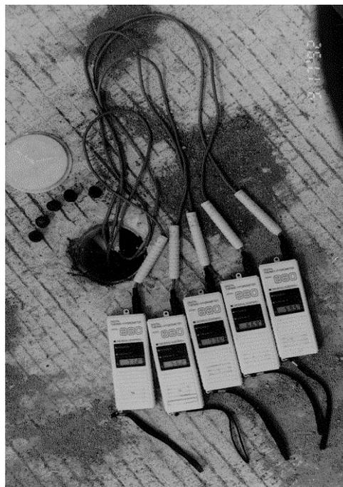
*Figure 3.24 Measurement of RH in the field*
