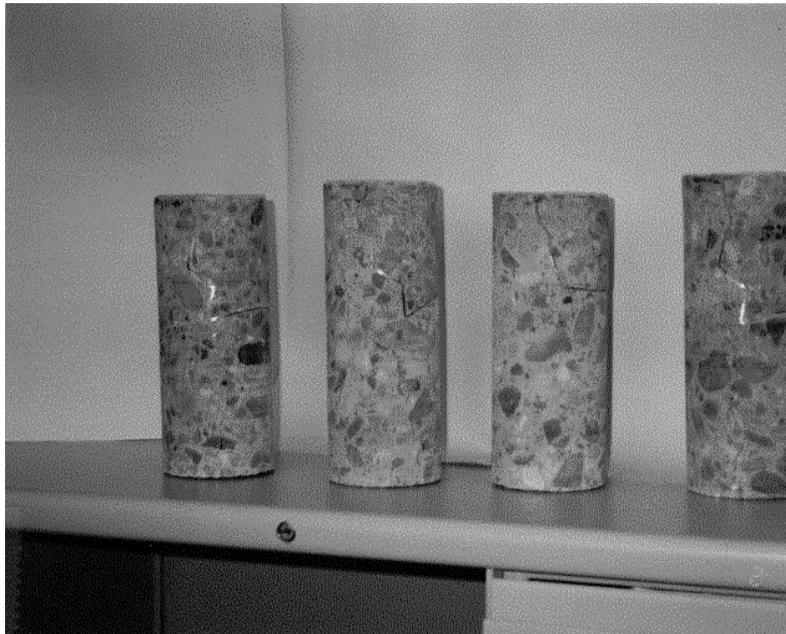
***Figure 3.3 Cores from nonsawcut part in TS3 where Type III crack inducer was located***
