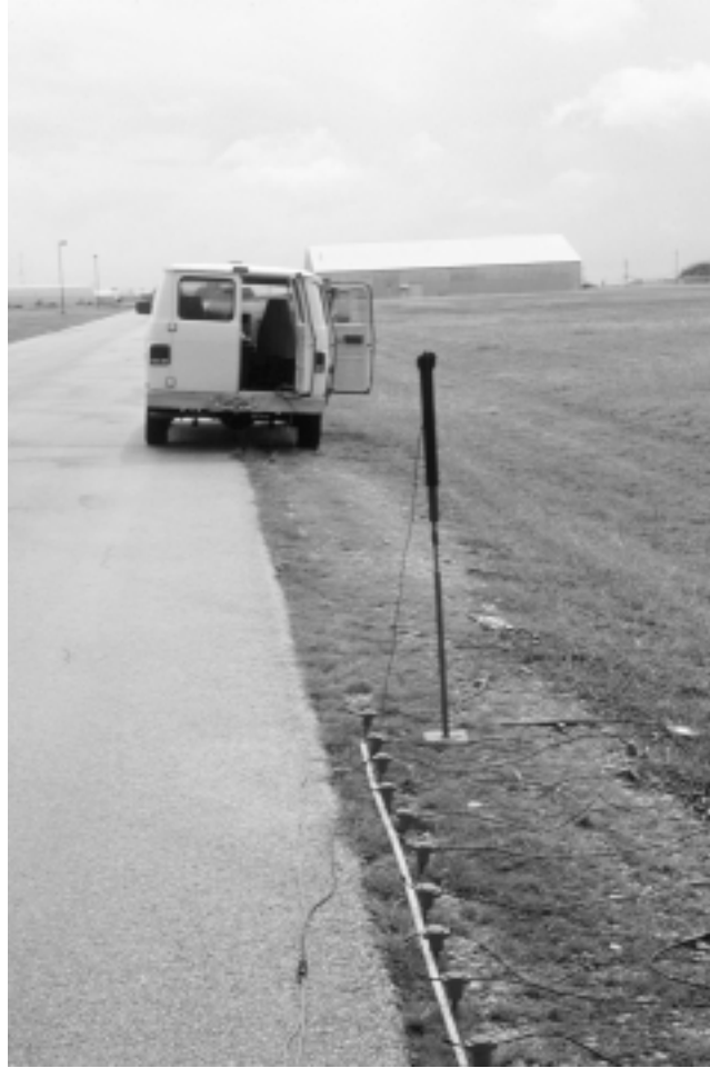
Figure 5. Soil-probe hammer and spike-mounted geophones on the shoulder of Road D at the J. J. Pickle Research Campus, The University of Texas at Austin.
