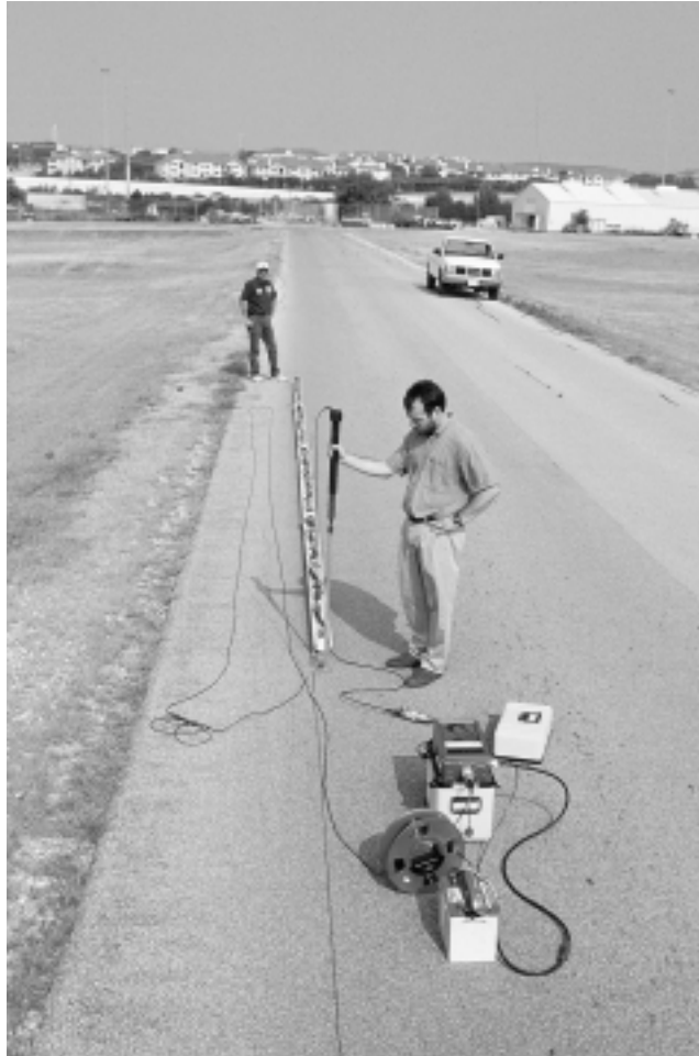
Figure 54. Photograph of Seismic Refraction Bedrock Analyzer deployed on pavement. The battery and seismograph are in the foreground. The soil-probe hammer is at the front end of the recording spread containing 24 geophones.
