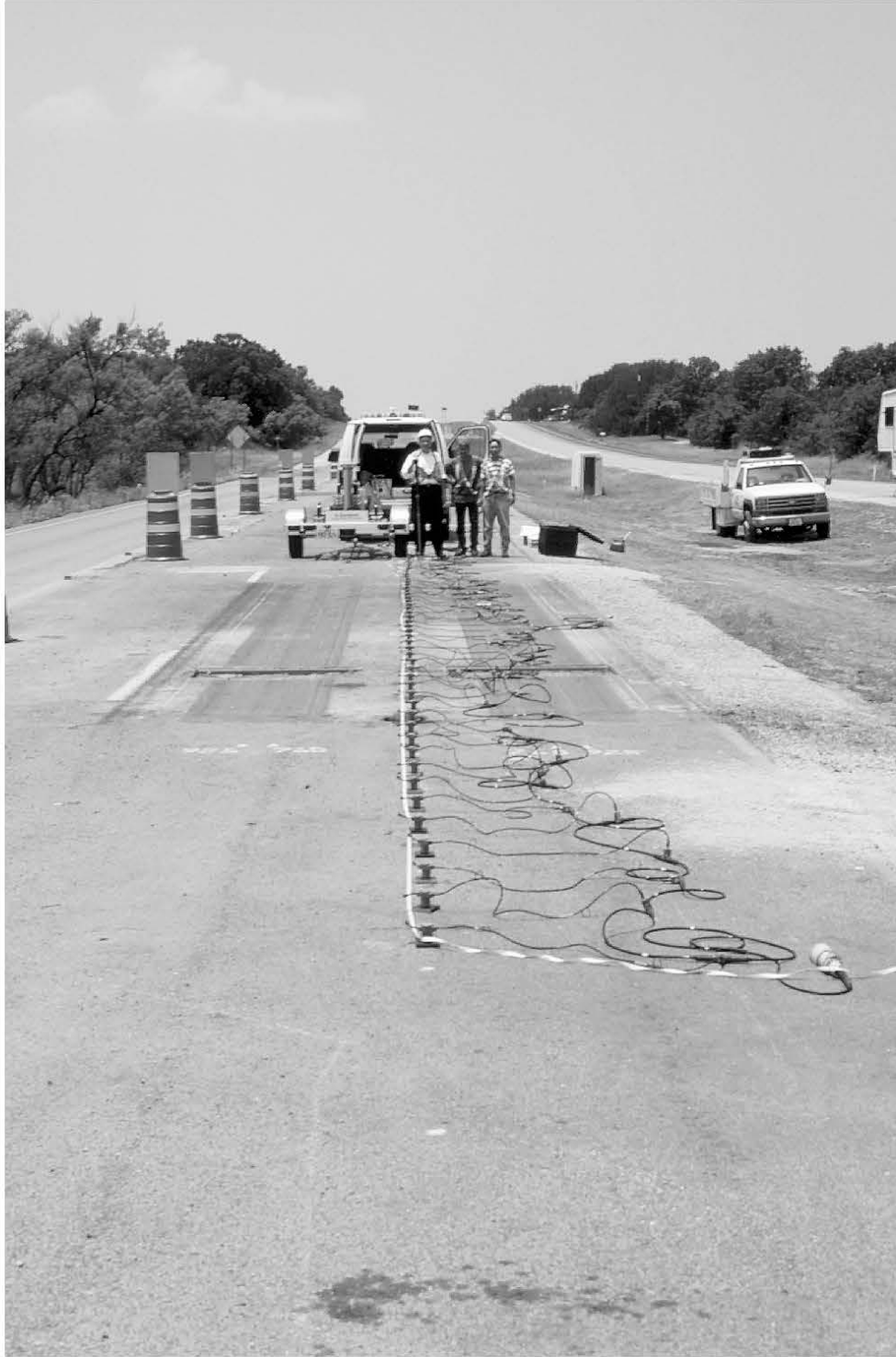
Figure 7. Geophones mounted on threaded steel plates and placed on the pavement of southbound U.S. Highway 281 at the Texas Department of Transportation's Mobile Load Simulator site south of Jacksboro, Texas.
