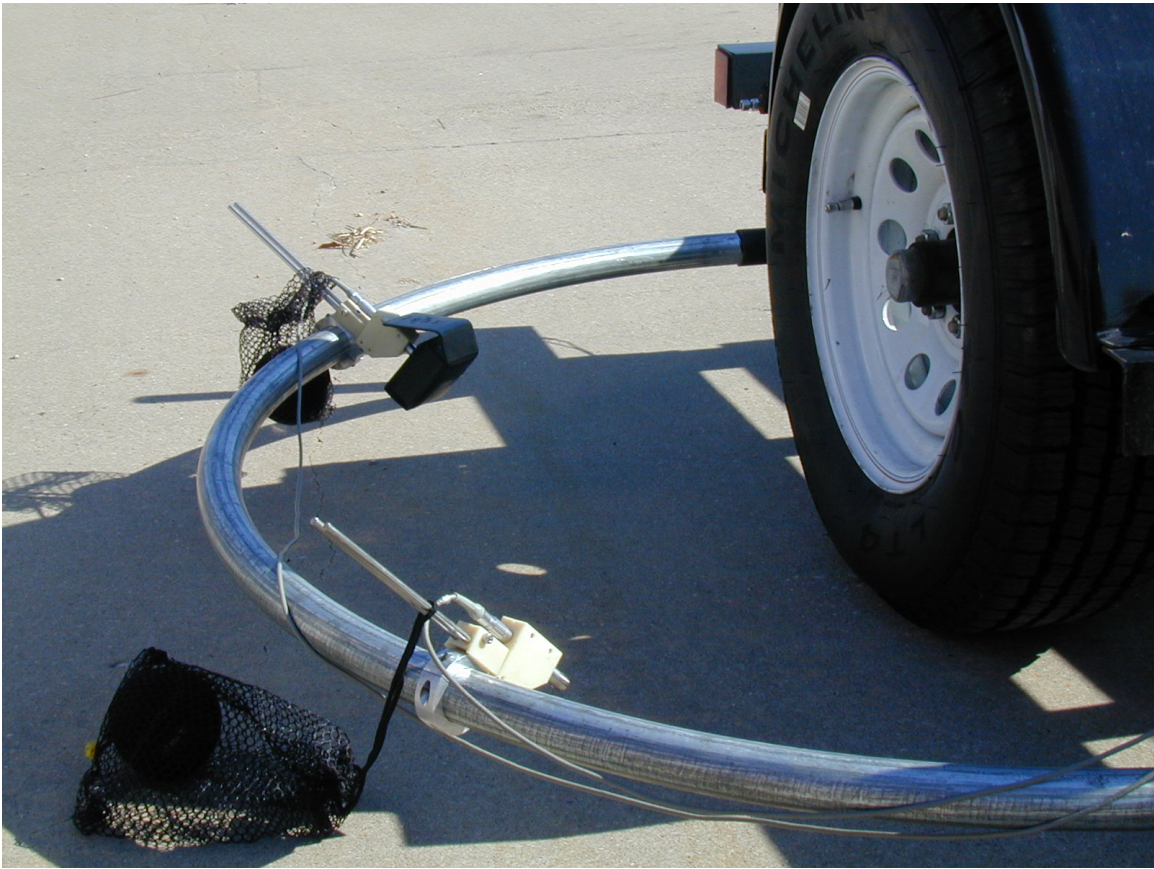
Figure 1-3: Microphone Locations on Second-Generation Trailer
