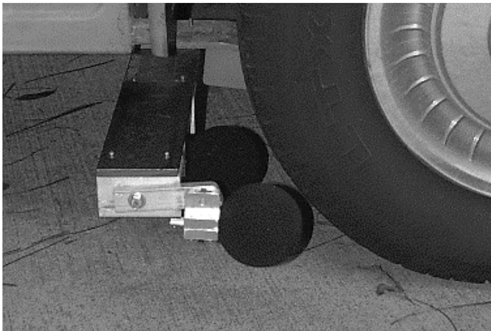
FIGURE 3. Photo of the onboard microphones with the windscreens in place
