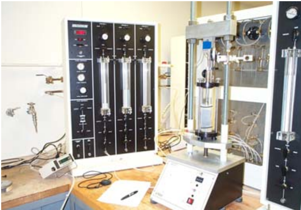
Figure 5-3. Apparatus used for conducting the unconsolidated-undrained triaxial compression tests
