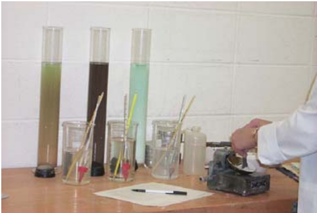
Figure 5-2. Determination of grain size distribution using the hydrometer test method, and determination of liquid limits using a hand-operated liquid limit device
