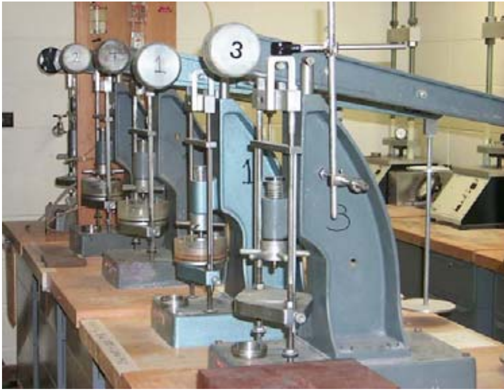
Figure 5-4. Apparatus used for conducting the one-dimensional free swell tests
