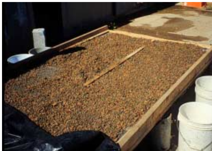
Figure 3.20 Drying of Aggregate on Screened Bed
