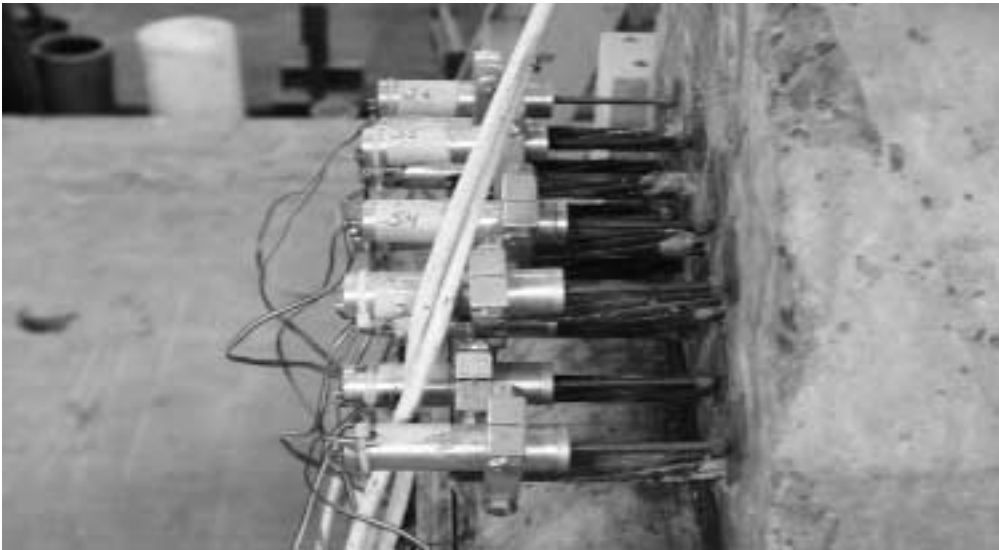
Figure 10.17 Strand Slip Measurement
