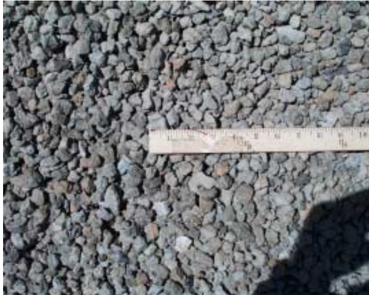
Figure 3.18 Appearance and Maximum Size of Western Aggregate
