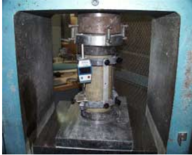
Figure 3.7 Test Setup for Modulus of Elasticity
