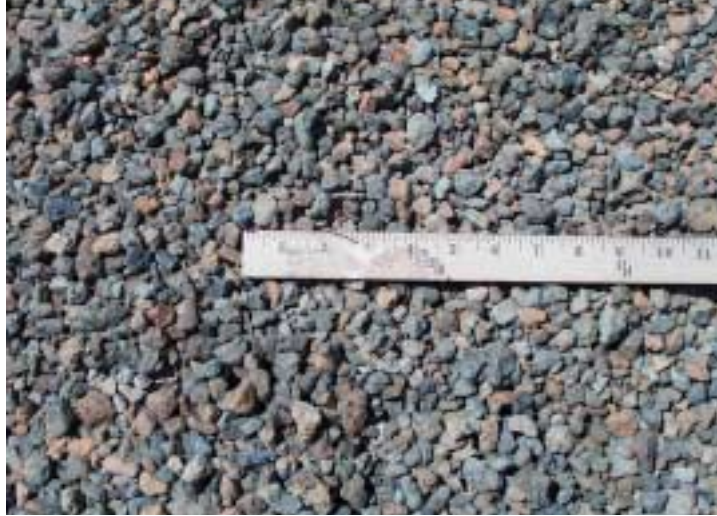
Figure 3.14 Appearance and Maximum Size of Clodine Aggregate
