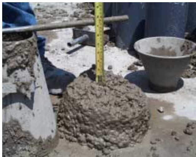
Figure 5.8 Slump for Second Batch of 8000 psi Concrete
