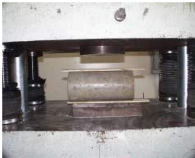
Figure 3.10 Test Setup for Splitting Tensile Test
