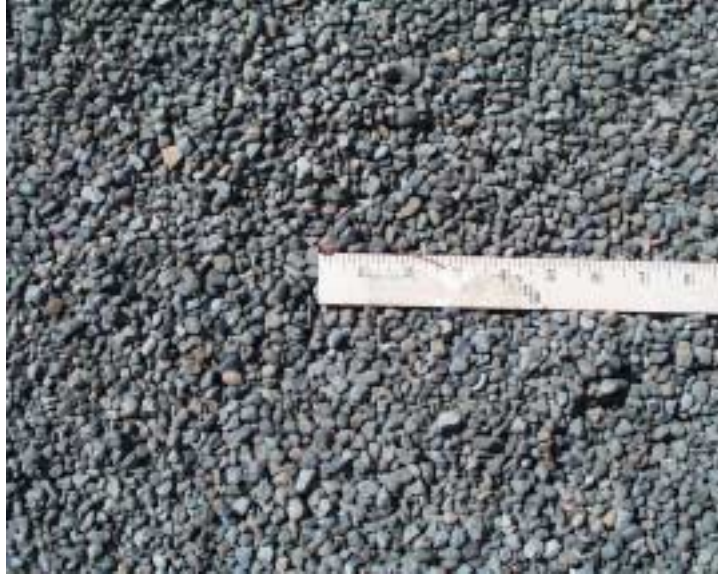
Figure 3.16 Appearance and Maximum Size of Streetman Aggregate
