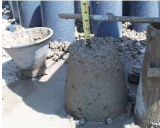
Figure 5.7 Slump for First Batch of 8000 psi Concrete
