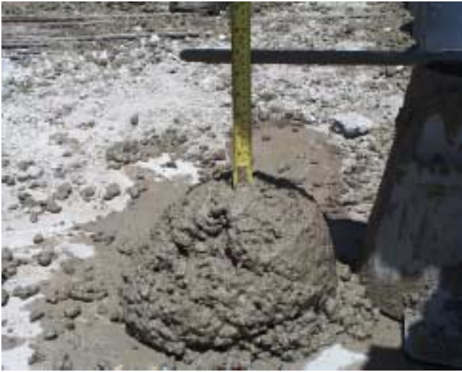
Figure 4.9 Slump of Second Batch of 6000 psi Concrete
