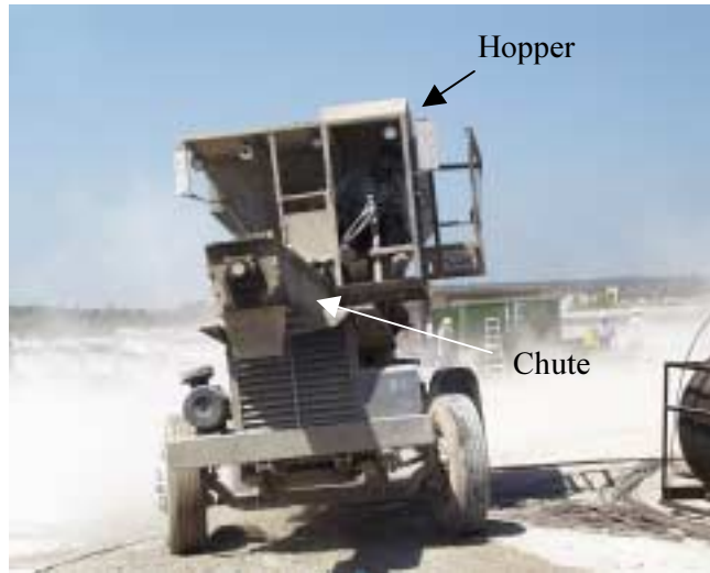
Figure 4.1 Sidewinder at Heldenfels Precast Plant
