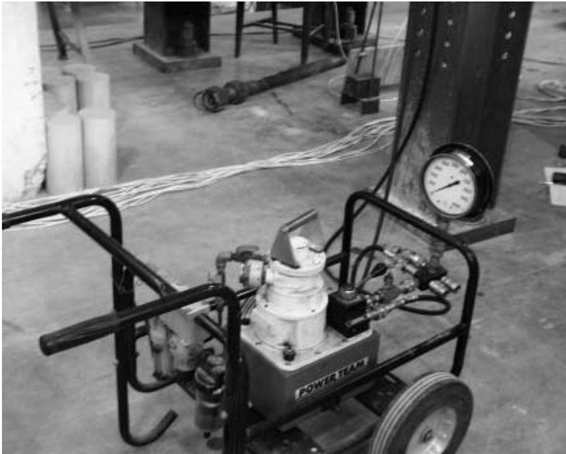
Figure 10.13 Hydraulic Pump and Pressure Gauge
