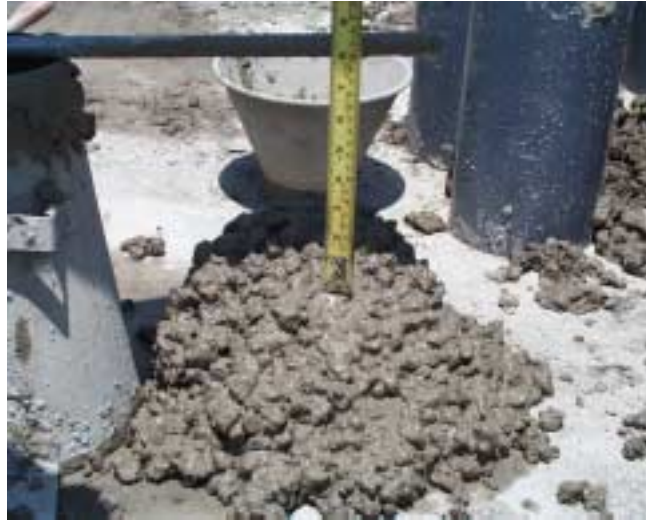
Figure 5.9 Slump for Third Batch of 8000 psi Concrete
