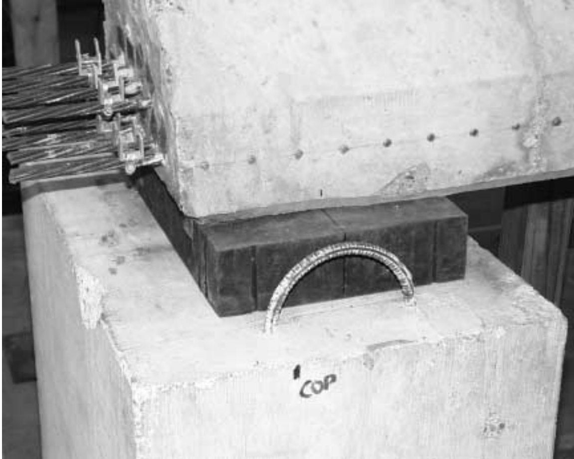
Figure 10.9 Beam on Pad and Concrete Block
