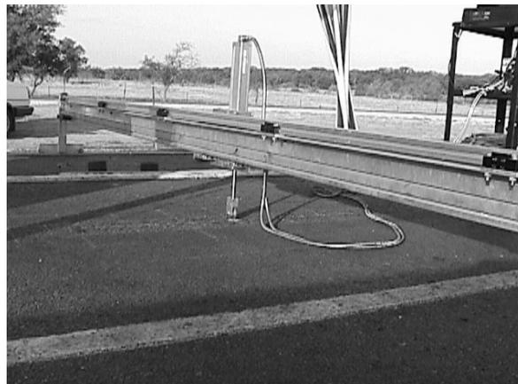
Figure 7. Profilometer measurements on MMLS3 test grid
