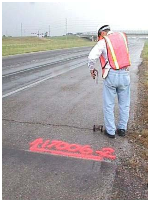
Figure 4.15 Beginning of Section 17006-2 with a transverse crack on southbound SH 6
