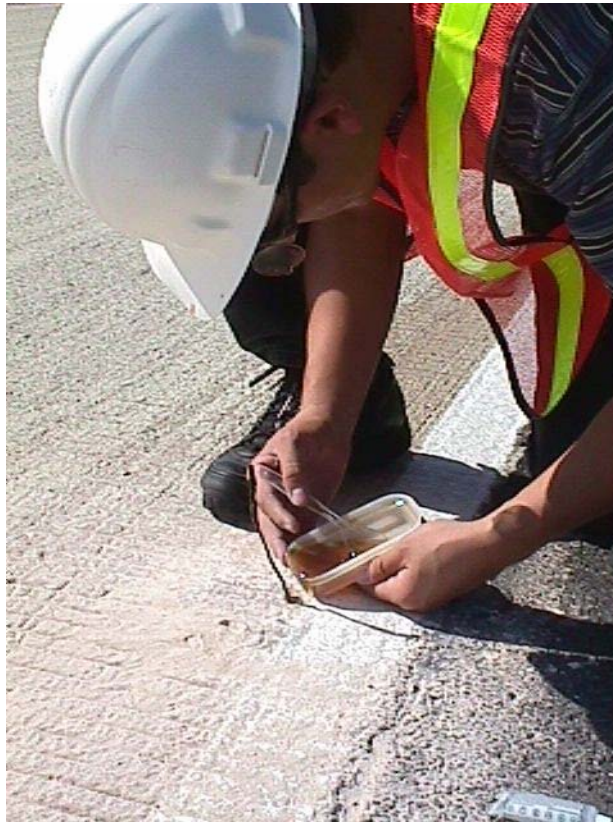
Figure 4.5 Liquid fiberglass being poured into hole containing I-Buttons
