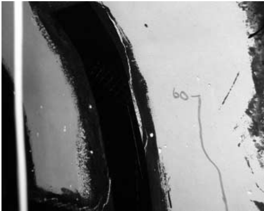
Figure 4.12 Crack Propagation Behind Strap Caused Debonding
