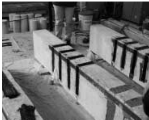
e) Final configuration of full-scale joist after strengthening
