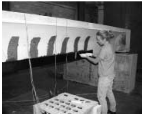
f) Coating placed sheets with epoxy
