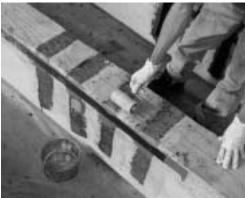
e) Final configuration of full-scale joist after strengthening
