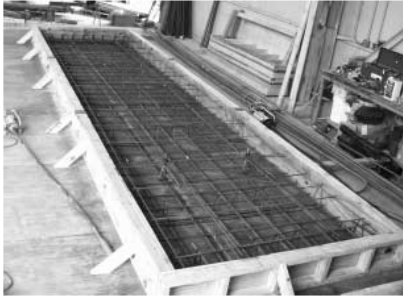
Figure 6.3 Reinforcement in a Typical Flat-Slab Specimen
