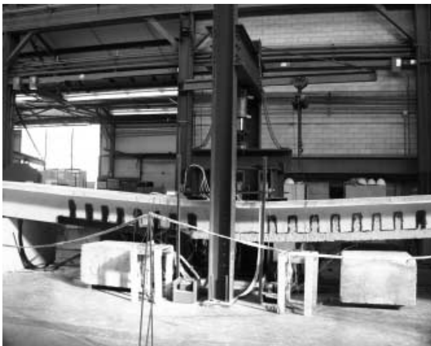
Figure 4.13 View of West Joist in Specimen J-2 at Failure
