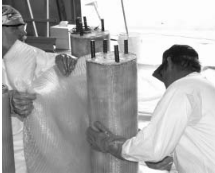
Figure 8.4 Applying FRP wrap to the concrete specimen
