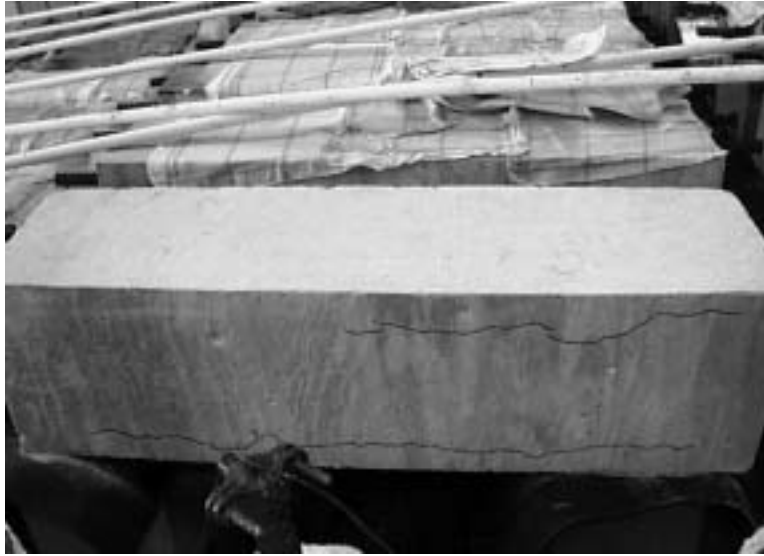
Figure 6.2 Longitudinal cracks forming on an uncracked specimen
