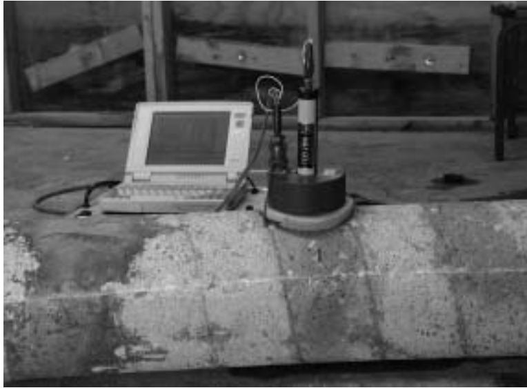
Figure 6.8 PR-Monitor test setup on specimen CC5
