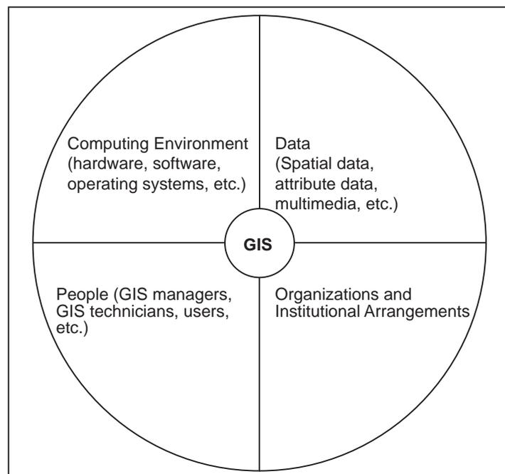
**Figure 2.1 The components of a geographic information system (GIS)**
