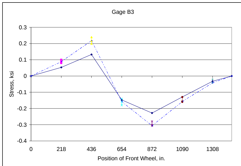
Fig. D.28: Field Test No. 1 - Member L2U2 of upstream truss
