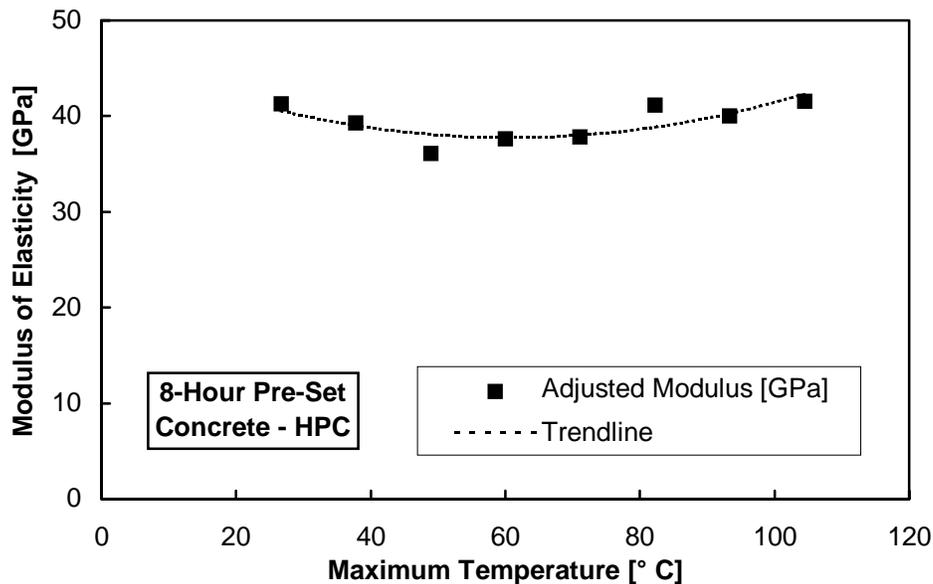
Figure 5.12 Typical variation of design modulus with curing temperature
