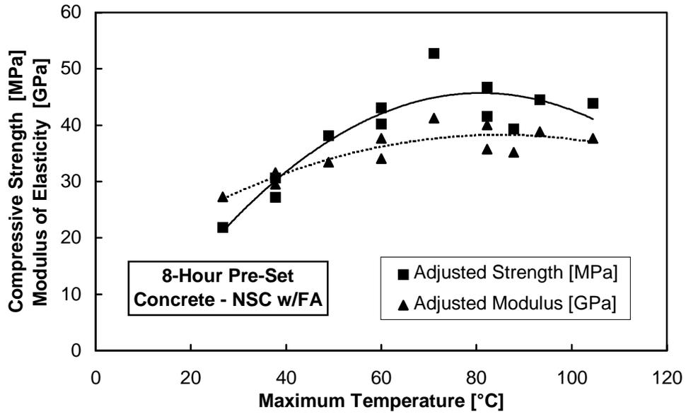
Figure 4.8 Release data for NSC with fly ash cured with an 8-hour pre-set period
