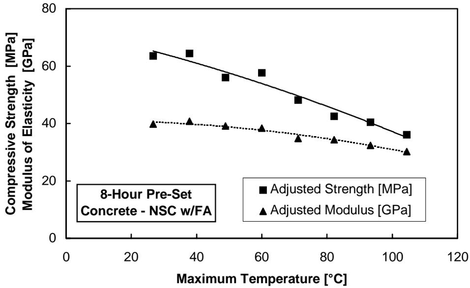
Figure 4.16 Twenty-eight-day data for NSC with fly ash match/air cured cylinders
