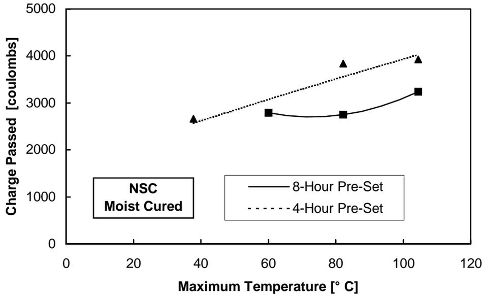
Figure 5.16 Permeability data for moist cured NSC without fly ash
