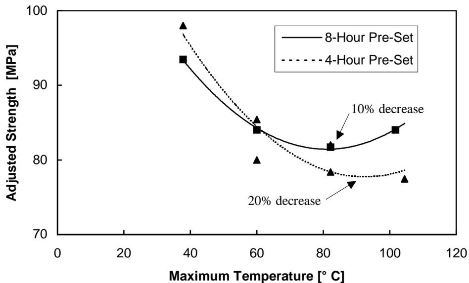
Figure 5.7 Compressive strength decrease of 8-hour and 4-hour pre-set specimens for the HPC mix
