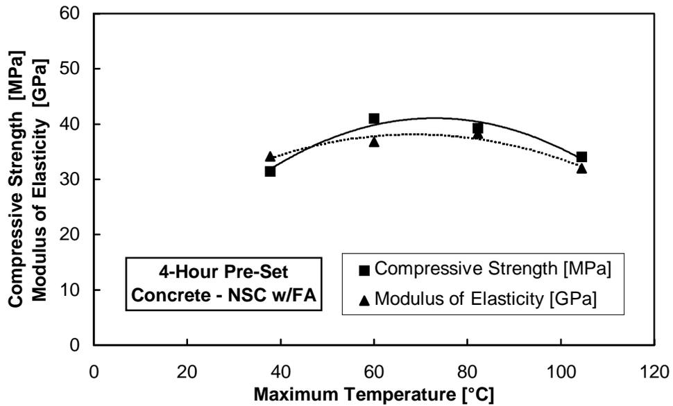
Figure 4.9 Release data for NSC with fly ash cured with a 4-hour pre-set period
