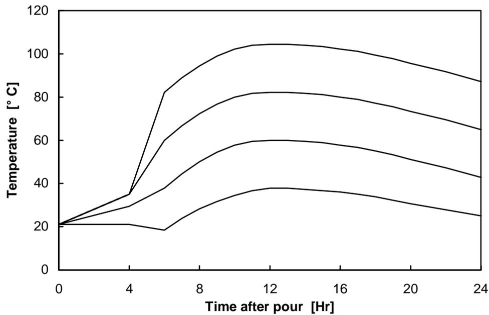
*Figure 3.2 Four-hour pre-set temperature profile model*
