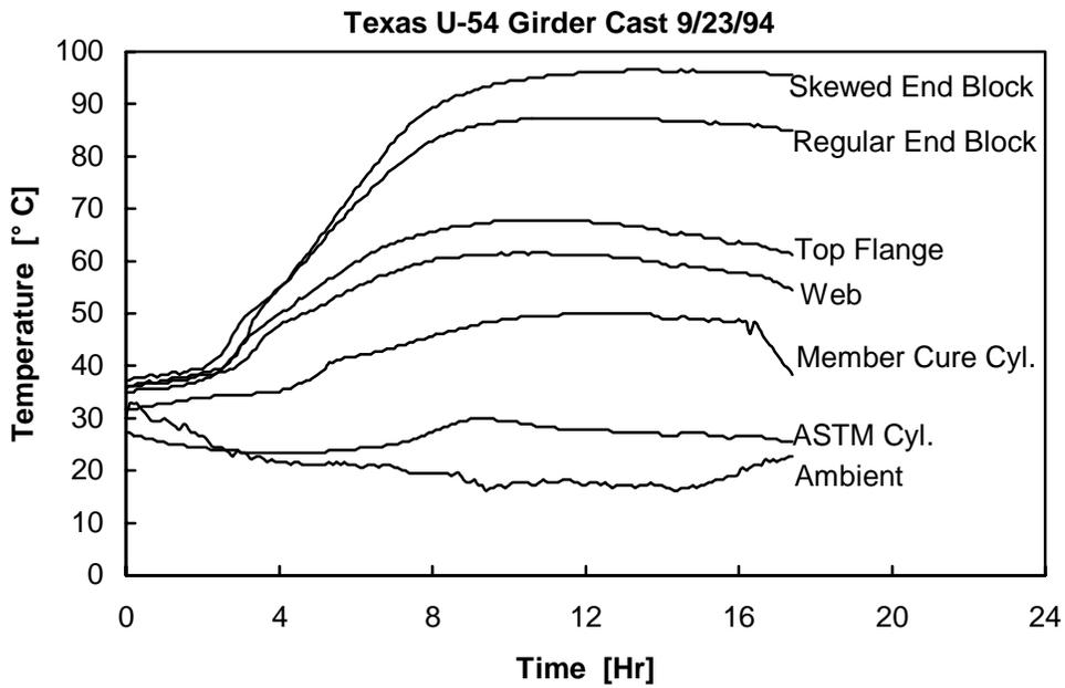
Figure 4.3 HPC temperature profile with 4-hour pre-set
