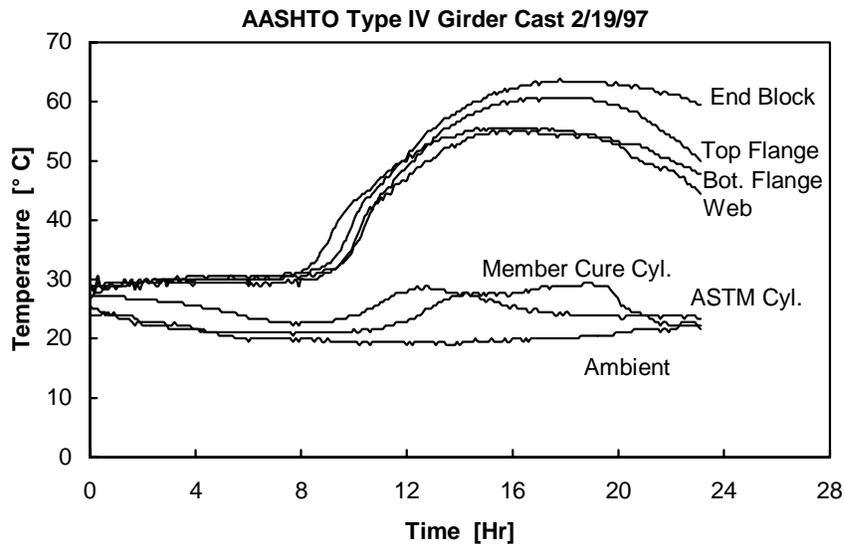
Figure 4.1 HPC temperature profile
