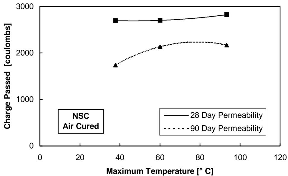
Figure 5.14 Permeability data for air cured NSC without fly ash
