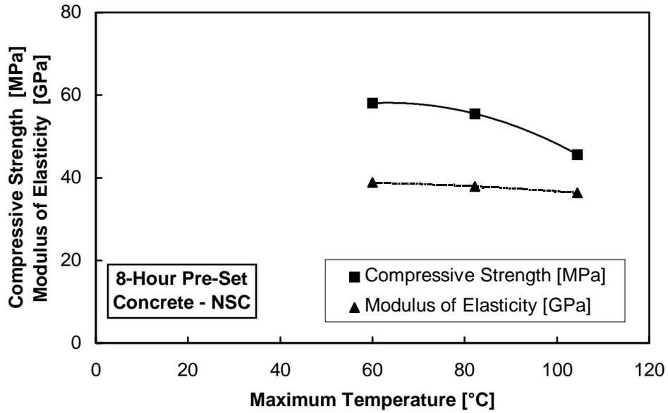
Figure 4.14 Twenty-eight-day data for NSC match/moist cured cylinders
