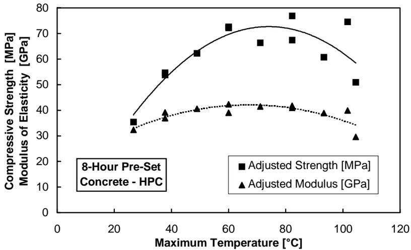
Figure 4.4 Release data for HPC cured with an 8-hour pre-set period
