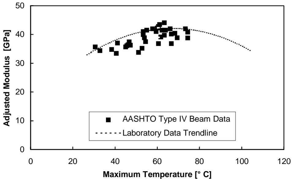
Figure 5.6 Comparison of modulus of elasticity data for laboratory and field specimens
