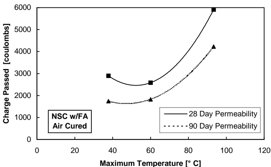
Figure 5.15 Permeability data for air cured NSC with fly ash
