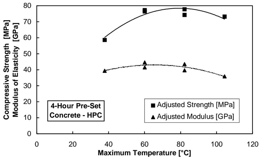
Figure 4.5 Release data for HPC cured with a 4-hour pre-set period
