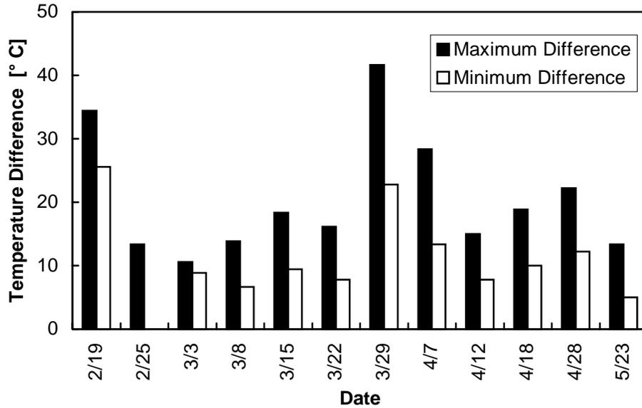
Figure 5.1 Difference between member concrete temperature and member cured cylinder for AASHTO Type IV girders
