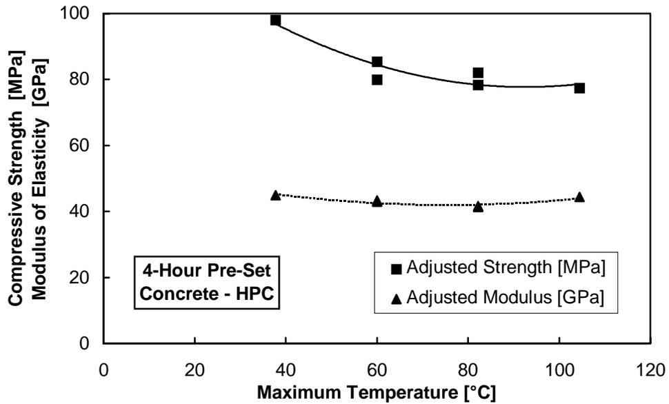
Figure 4.12 Fifty-six-day data for HPC match/moist cured cylinders with a 4-hour pre-set period
