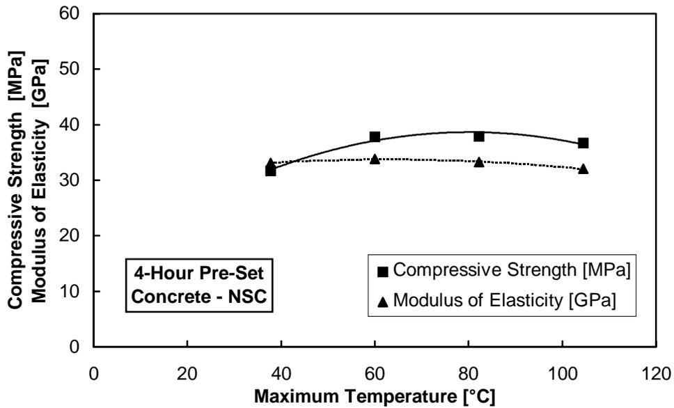
Figure 4.7 Release data for NSC cured with a 4-hour pre-set period
