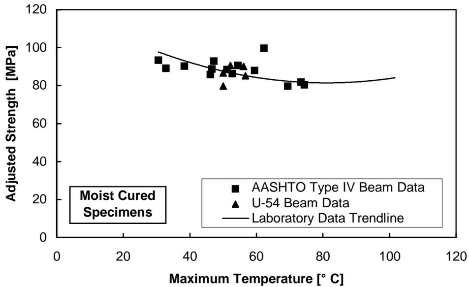
Figure 5.11 Comparison of moist cured design strength data from the laboratory and field
