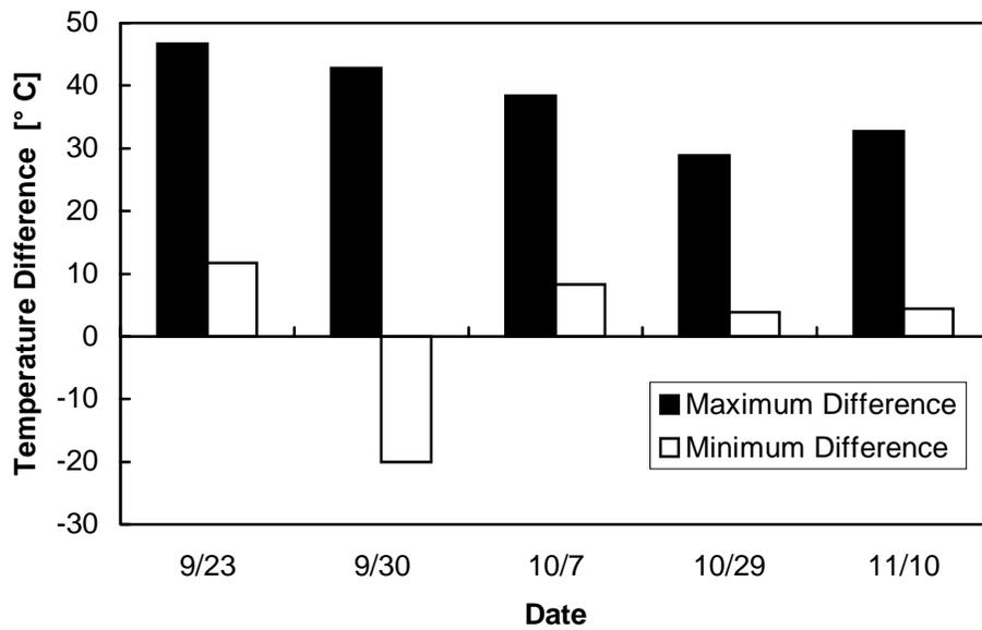
Figure 5.2 Difference between member concrete temperature and member cured cylinder for Texas U-54 girders
