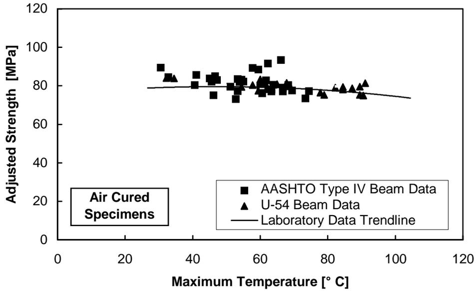
Figure 5.10 Comparison of air cured design strength data from the laboratory and field
