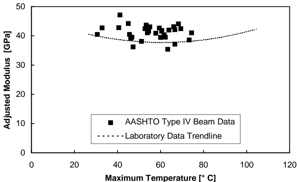
Figure 5.13 Comparison of modulus of elasticity data from the laboratory and field
