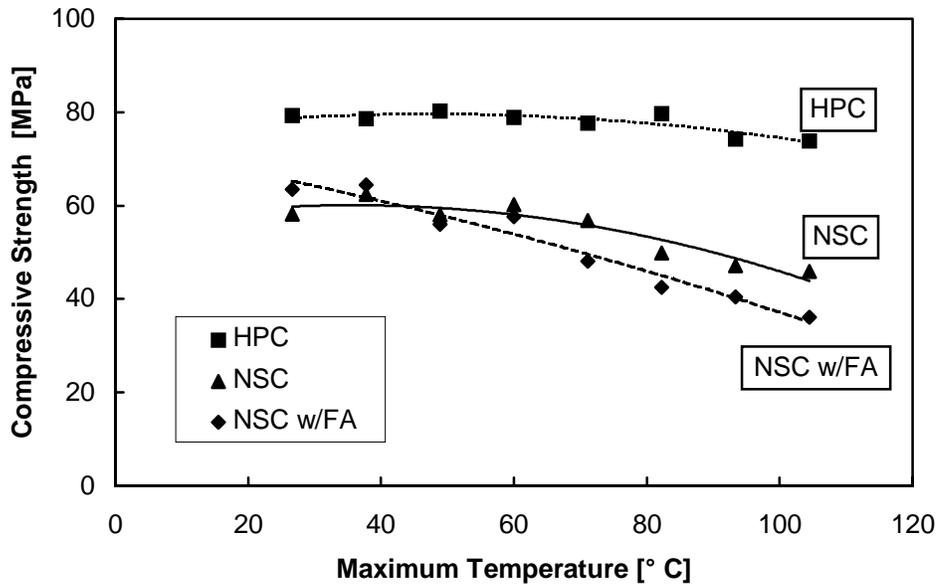
Figure 5.9 Compressive strength decrease for the three mixes evaluated
