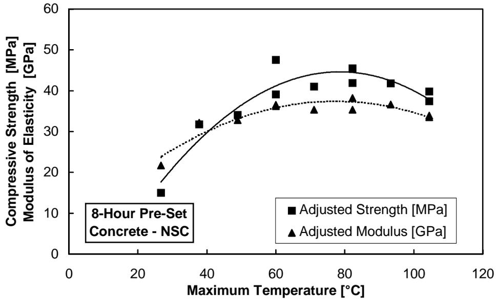
Figure 4.6 Release data for NSC cured with an 8-hour pre-set period
