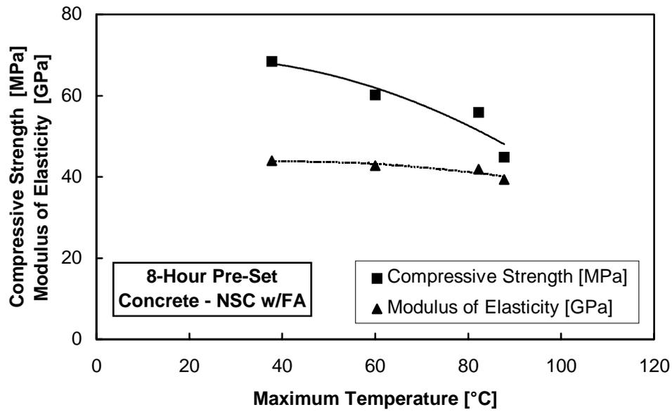
Figure 4.17 Twenty-eight-day data for NSC with fly ash match/moist cured cylinders
