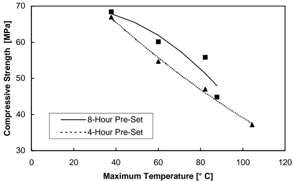
*Figure 5.8 Compressive strength decrease of 8-hour and 4-hour pre-set specimens for the NSC mix with fly ash*
