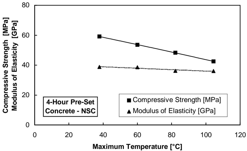
Figure 4.15 Twenty-eight-day data for NSC match/moist cured cylinders with a 4-hour pre-set period
