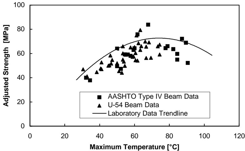
*Figure 5.5 Comparison of compressive strength data for laboratory and field specimens*
