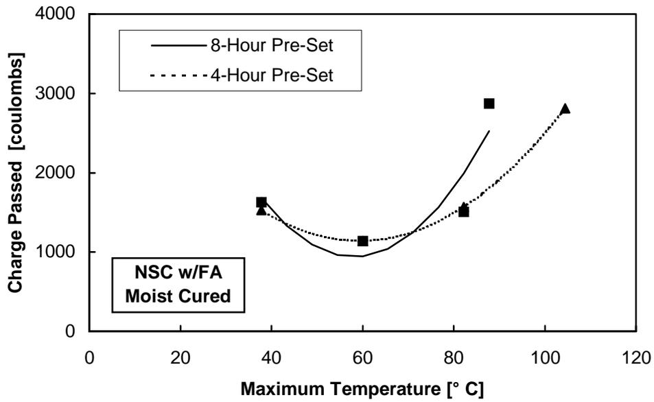
Figure 5.17 Permeability data for moist cured NSC with fly ash
