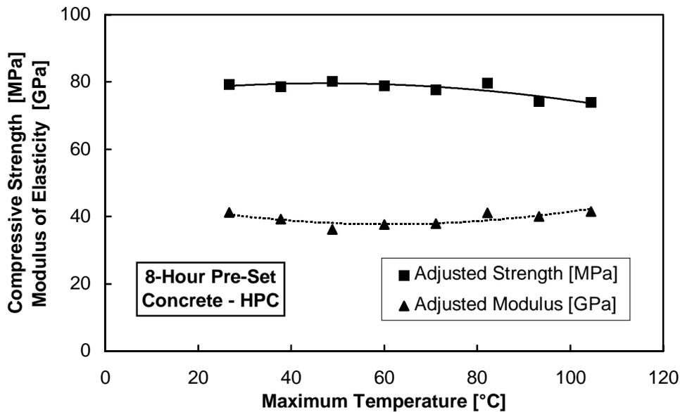
Figure 4.10 Fifty-six-day data for HPC match/air cured cylinders
