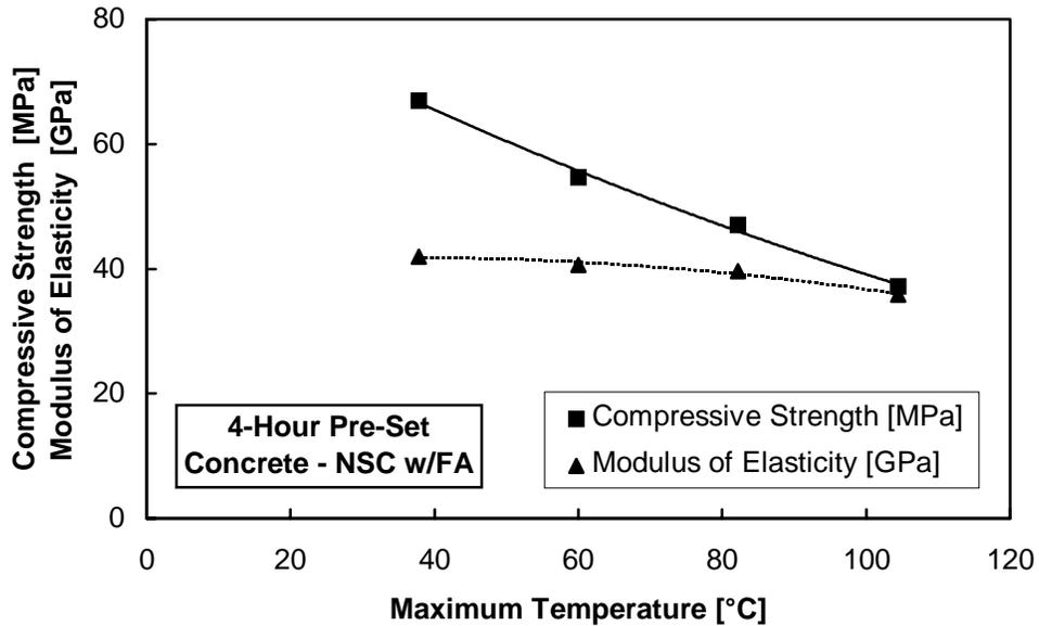
Figure 4.18 Twenty-eight-day data for NSC with fly ash match/moist cured cylinders with a 4-hour pre-set period
