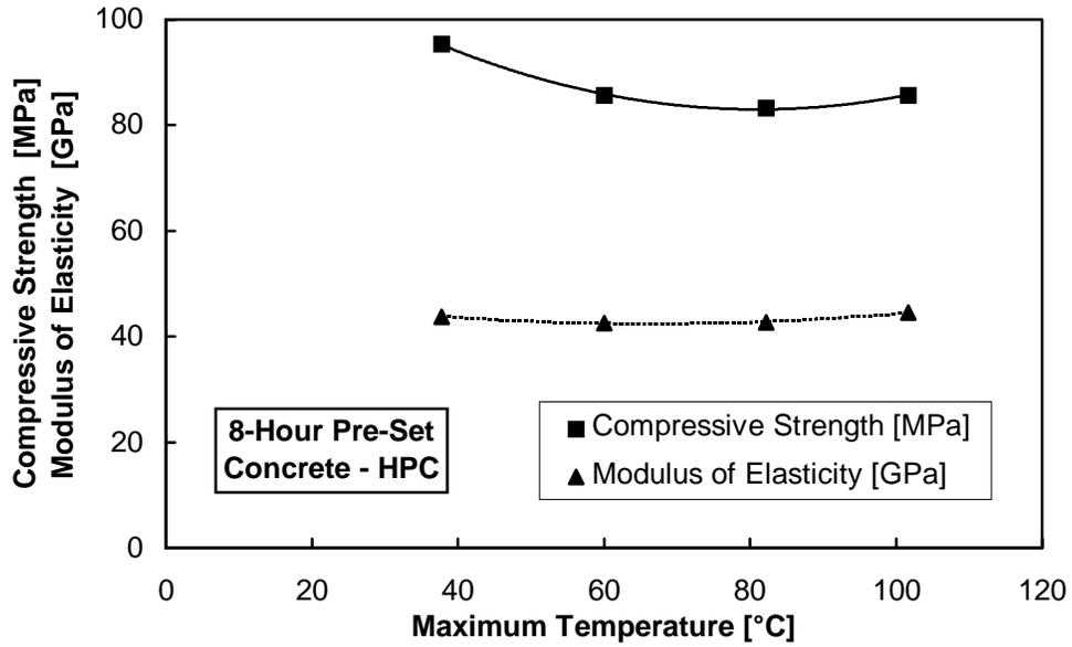
Figure 4.11 Fifty-six-day data for HPC match/moist cured cylinders
