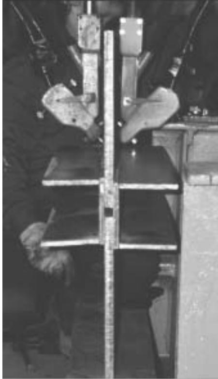
**Figure 2.4 Test plate with tacked wing plates**
