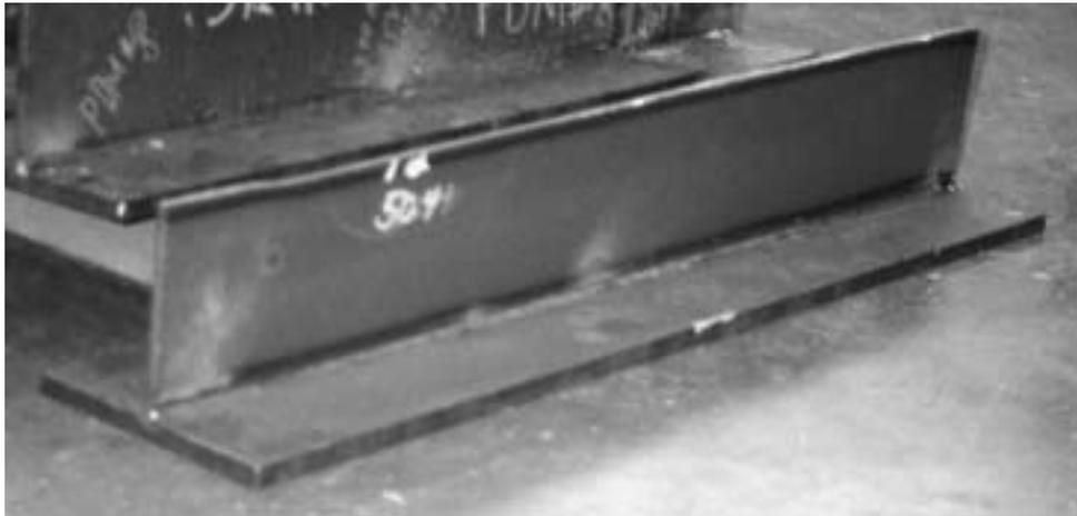
**Figure 3.1 T-bend specimens as fabricated**
