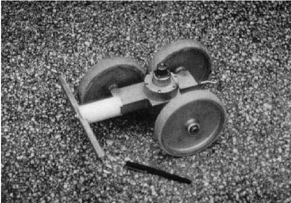
Figure 5.17 Photograph of Second-Generation RDD Rolling Sensor
