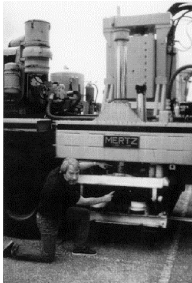
Figure 7.14 Photograph Showing Guide Rod Joint and Location of Bolts under Loading Foot
