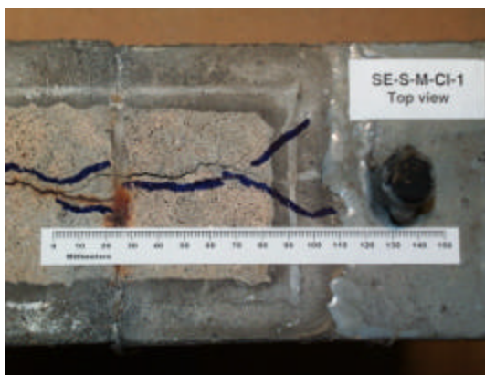
Specimen condition prior to autopsy (Top view)
