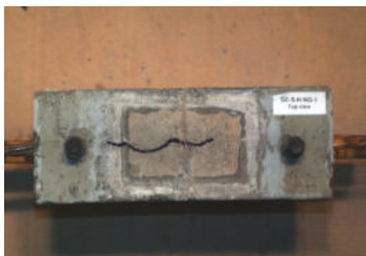
Specimen condition prior to autopsy (Top view)
