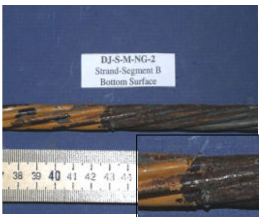
Specimen condition prior to autopsy (Top view)
