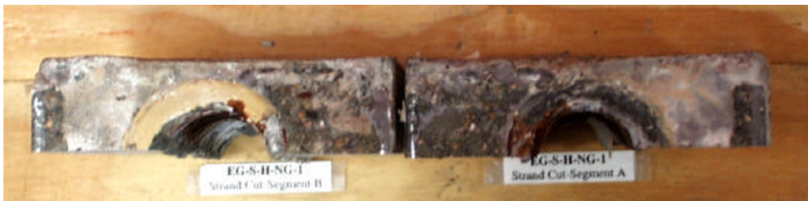
Figure 4.30 Incomplete Epoxy Coverage in Epoxy/Gasket Joint (EG-S-H-NG-1).
