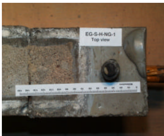
Specimen condition prior to autopsy (Top view)
