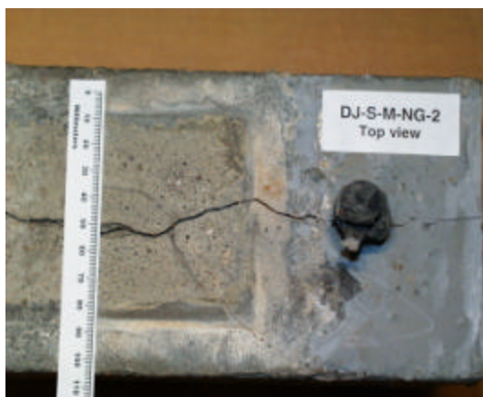
Specimen condition prior to autopsy (Top view)
