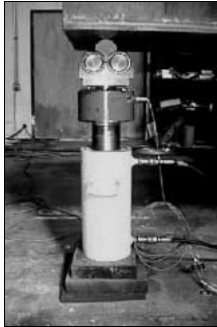
Figure 3.6 Load Ram, Load Cell, and Roller/Bearing Assembly
