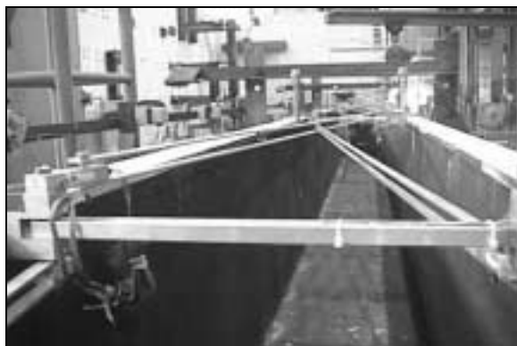
Figure 4.13 Bracing Taught before Loading
