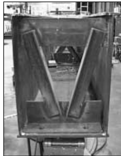
Figure 3.8 K-Brace at Location of Concentrated Load
