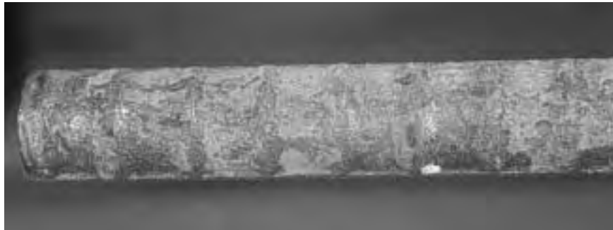
(a) Accumulation of reddish-brown rust products on side near the concrete surface
