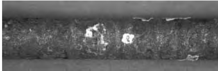
Figure 2.79 Dark corroded surface on longitudinal upper bar of beam B8 within the wetted region (zone at midspan).
