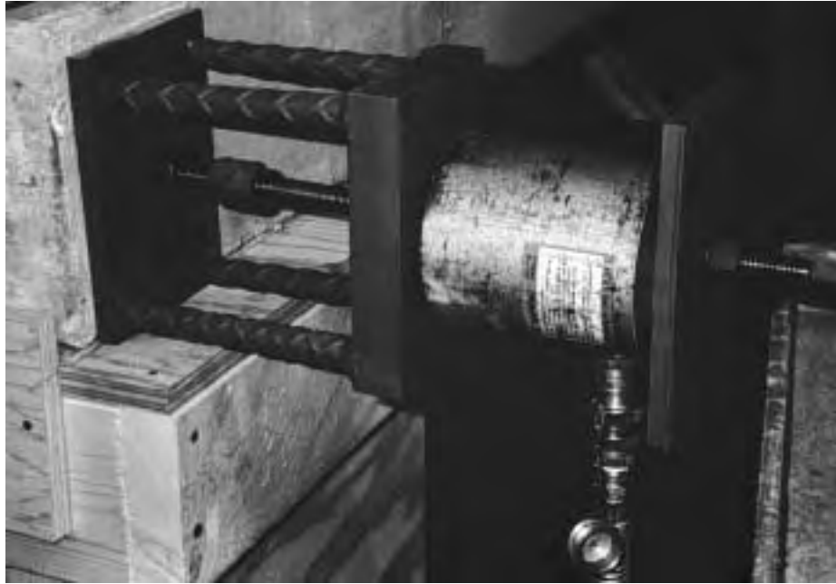
Figure A.16 Beam loading system.
