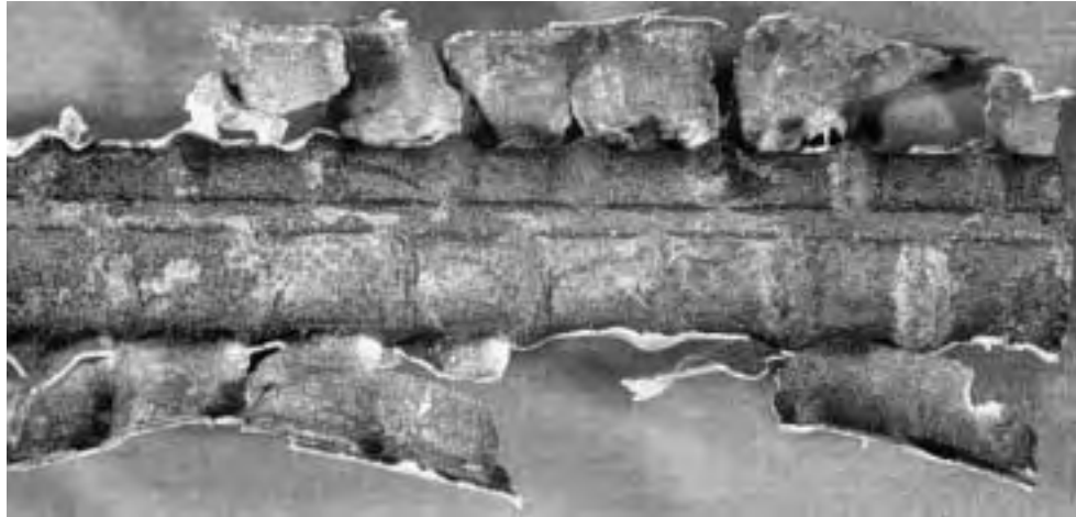
Figure 2.77 Undercutting along splice bar at patched cut end after one year of exposure.
