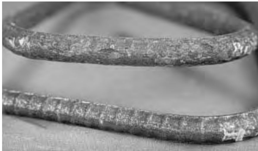
Figure 2.85 Corrosion on stirrup leg (top in photo) and mottled surface on stirrup hook (bottom in photo). Portion near the front beam surface (beam B32).
