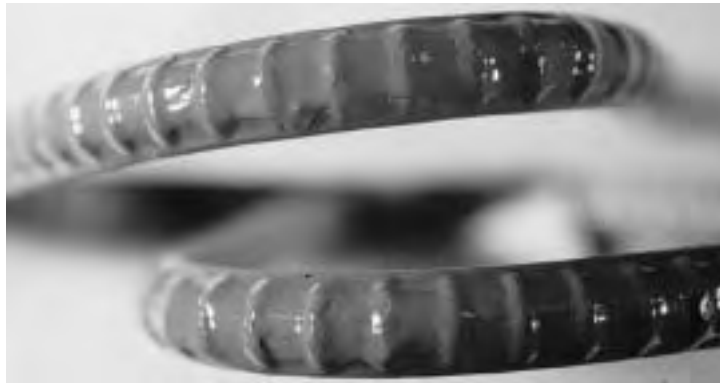
(b) 3% damaged and patched bends
