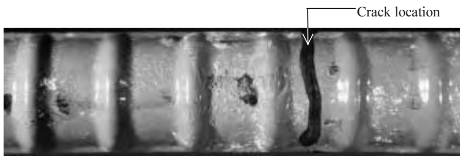
Figure 2.49 Corrosion on lower side of patched bar removed after one year of exposure.
