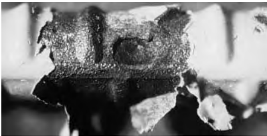
(b) Pitting on lower longitudinal bar
