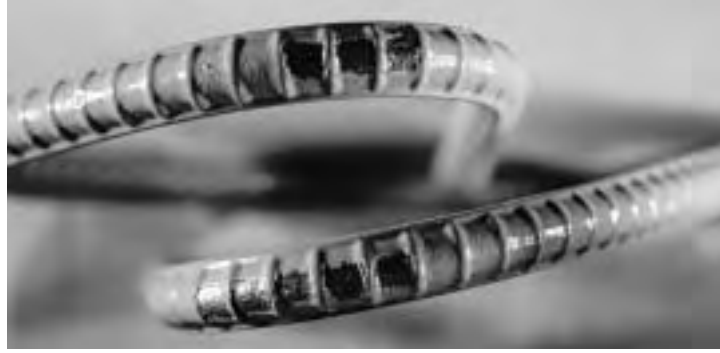
(a) 3% damaged bends
