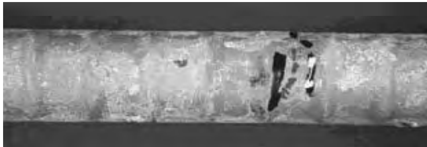
Figure 2.52 Aspect of uncorroded patched area on upper bar in beam B14, near crack location within the wetted zone after 4.3 years.
