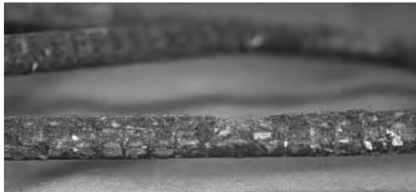
Figure 2.83 Pitting on stirrup leg near the bottom beam surface (beam B17).
