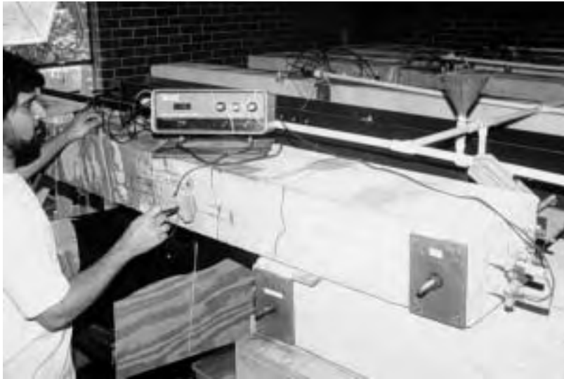
Figure 1.6 Corrosion potentials measurement.
