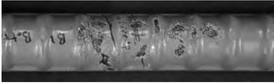
Figure 2.70 Coating adhered well throughout most portions of bars from beam B1 after 4.3 years of exposure.
