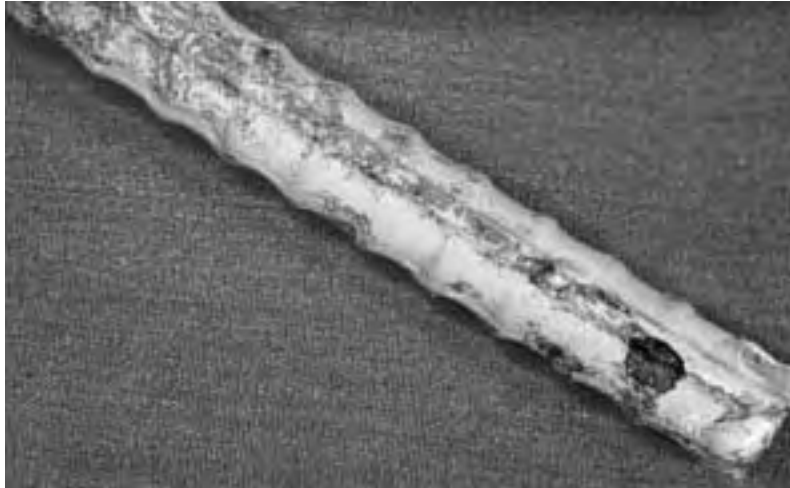
Figure 2.54 Corrosion on hook end of stirrup removed from cracked loaded beam after one year of exposure.
