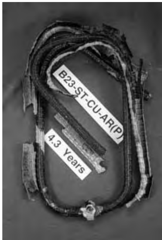
Figure 2.71 Coating extensively debonded on stirrups after 4.3 years.
