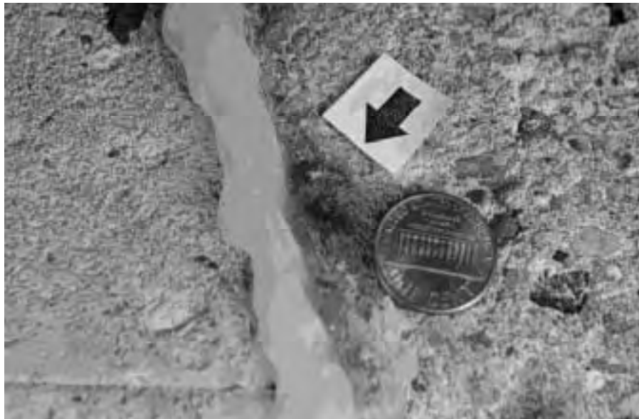
Figure 2.33 Rust spot just outside wetted region on beam B12.
