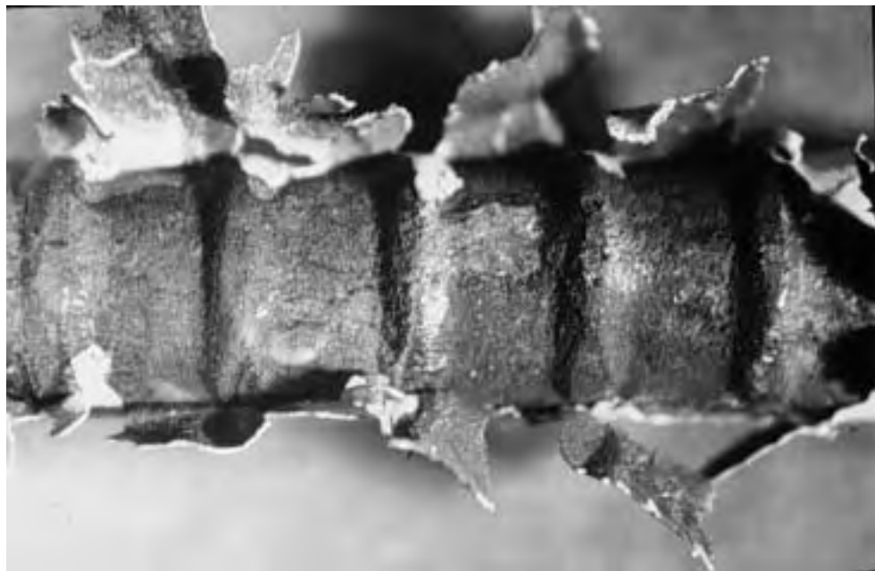
(c) Corrosion on bar from cracked loaded beam B11
