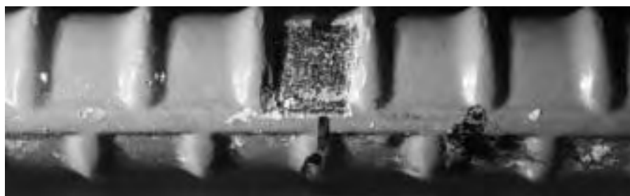
(b) No corrosion on upper side of bar
