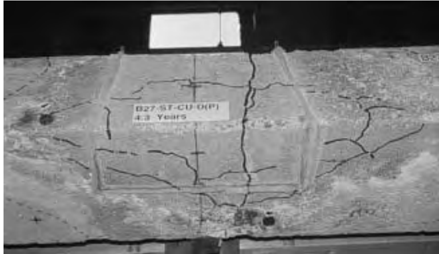
Figure 3.30 Random cracking at and around wetted region of beam B27.
