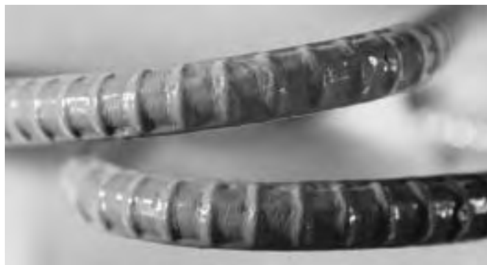
(b) As-received, patched condition of bends
