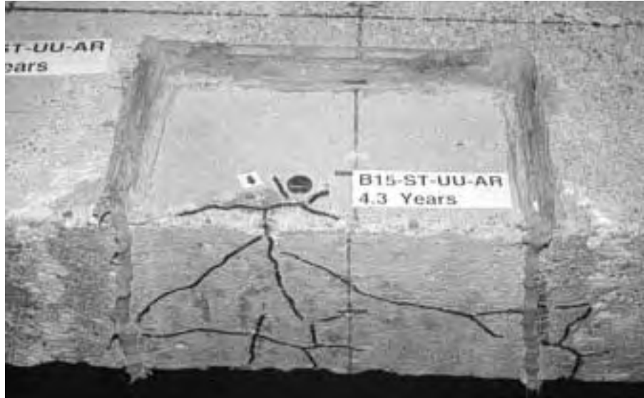
Figure 2.35 Random cracking on front surface of beam B15.
