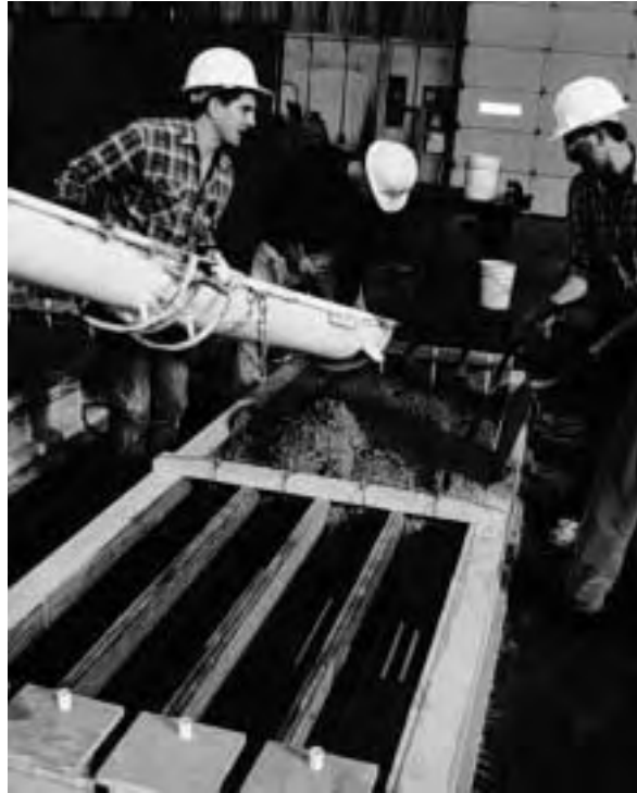
Figure A.13 Casting beam specimens.
