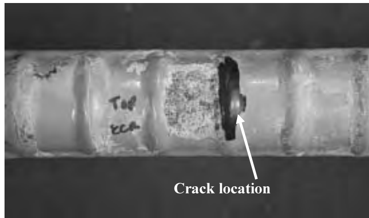
(a) Uncorroded damaged spot near a crack within the wetted region (Upper bar)
