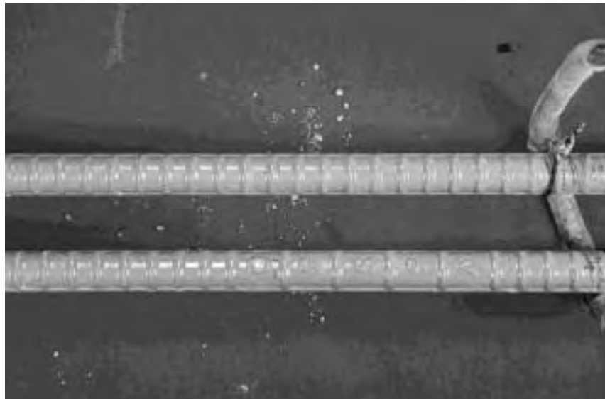
Figure 2.47 Longitudinal coated bars of beam B1 after 4.3 years of exposure.
