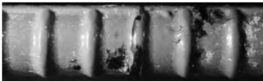
(a) Corrosion on lower side of bar (facing cover)
