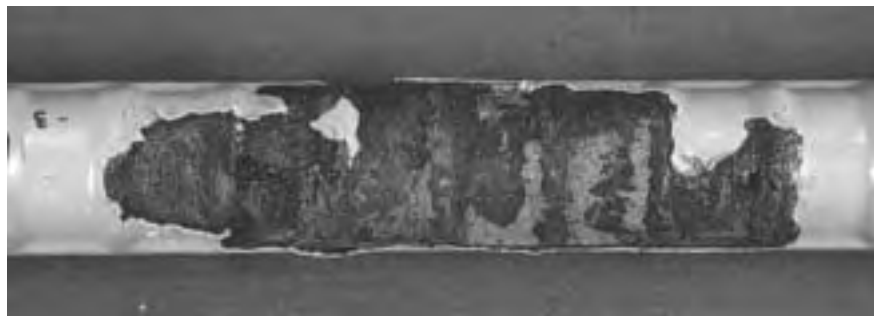
Figure 2.81 Reddish-brown rust products on lower bar of beam B8 (Zone just outside of wetted region).
