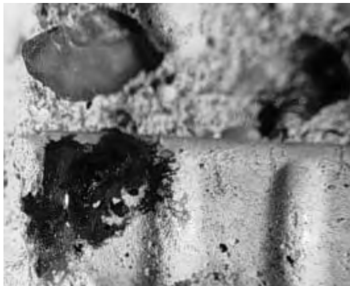
Figure 2.44 Corrosion spots coincident with voids in concrete (specimen removed after one year).
