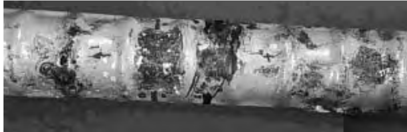
(b) Bar of beam B10, portion at midspan (wetted zone)
