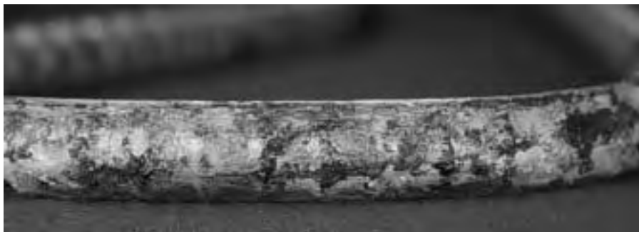
Figure 2.59 Rust staining on a stirrup leg near the front beam surface (beam B32) after 4.3 years.
