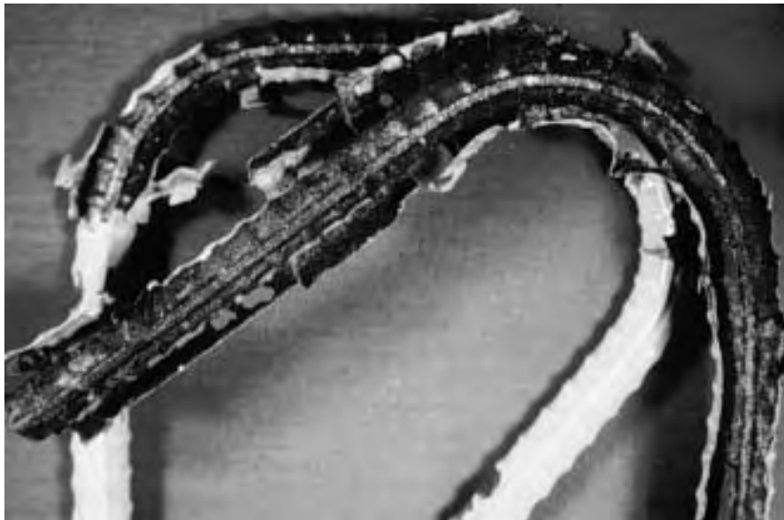
Figure 2.76 Example of undercutting on stirrup with 3% patched damage after one year of exposure.
