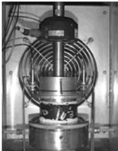
Figure 3.5: Static Creep Test Setup
