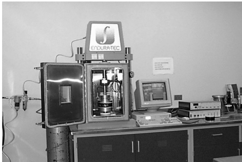
Figure 3.1: Static Creep Testing Apparatus
