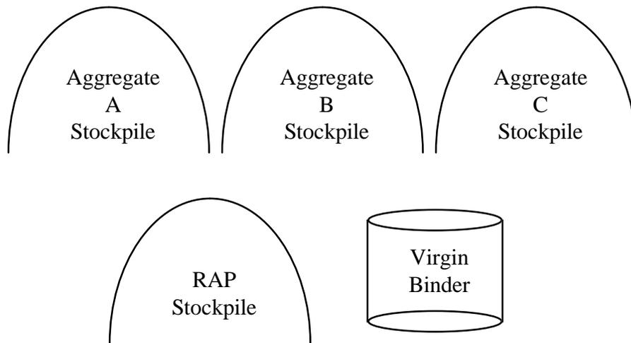
*Figure 4.6 Component material in a mix containing RAP*
