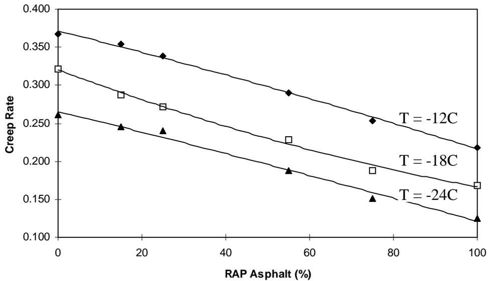
Figure 3.9 Creep rate trend for RTFOT and PAV-aged DG blend
