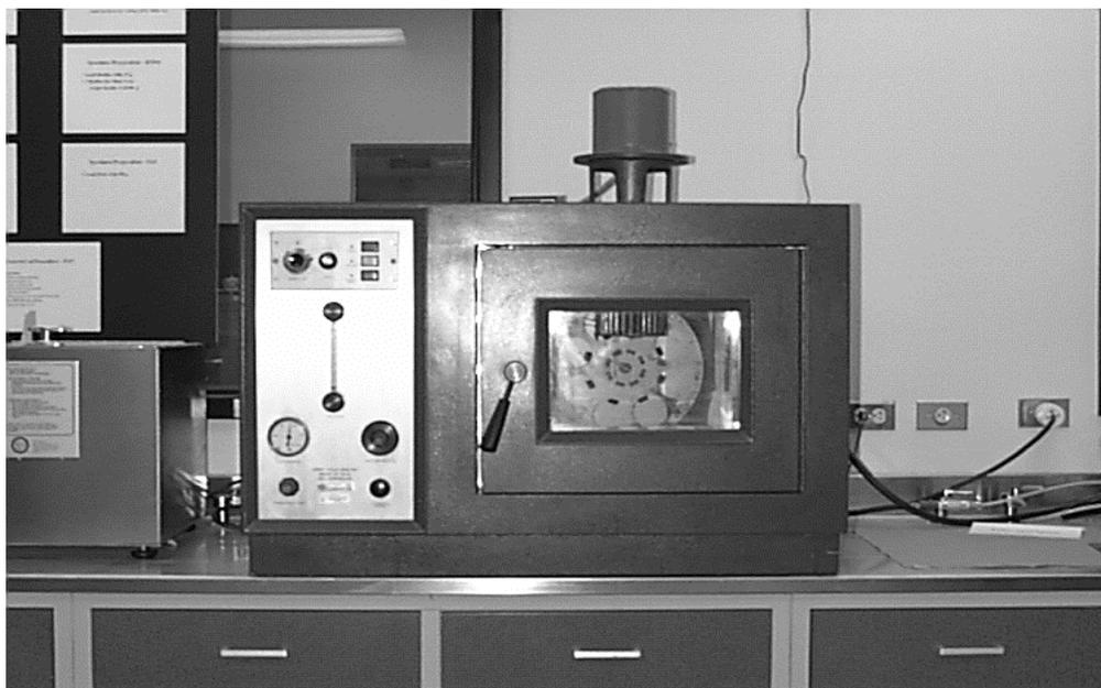
*Figure 2.1 Rolling thin film oven*
