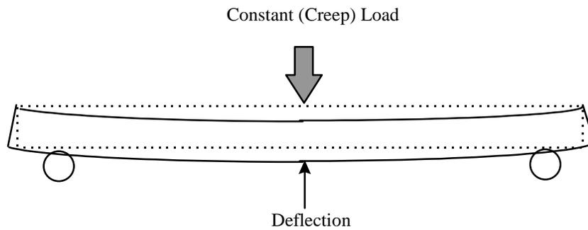
*Figure 2.6 Bending beam rheometer loading geometry*
