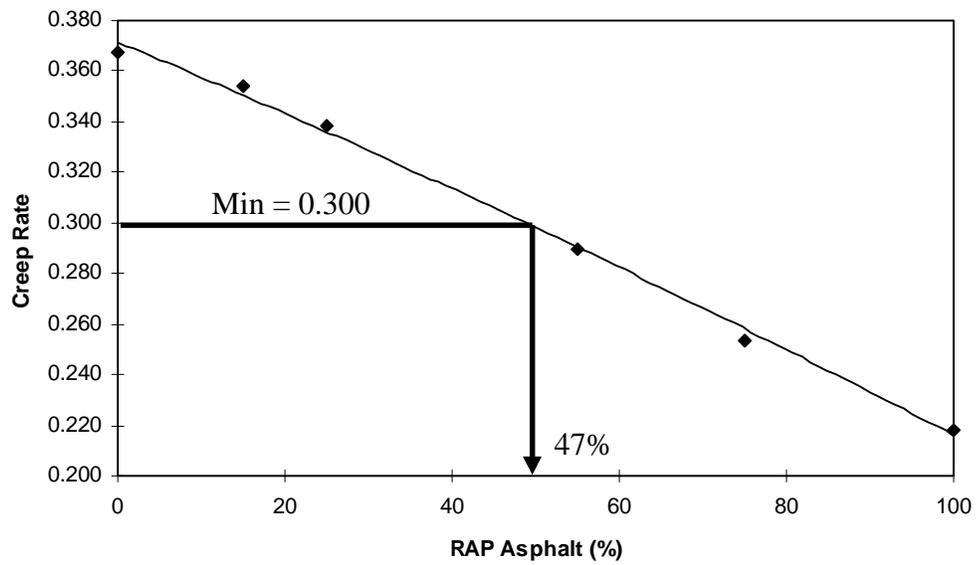
Figure 4.4 Creep rate trend for RTFO and PAV-aged DG blend at  $-12^{\circ}\text{C}$
