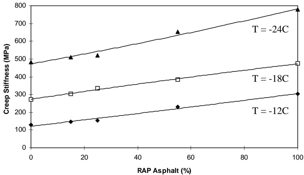
Figure 3.8 Creep stiffness trend for RTFOT and PAV-aged CF blend
