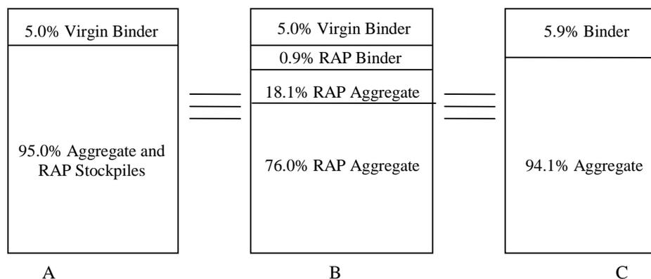
*Figure 4.7 Schematic view of material components in the mix*
