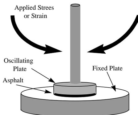
*Figure 2.4 Dynamic shear rheometer loading geometry*
