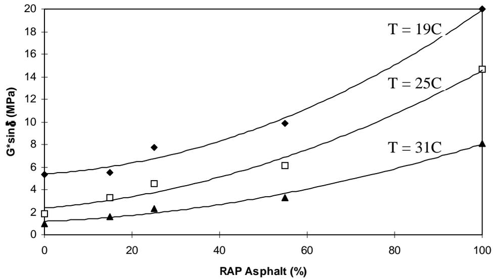
Figure 3.5  $G^* \sin \delta$  trend for RTFOT and PAV-aged MG blend
