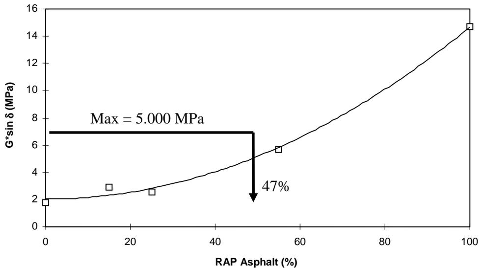
Figure 4.5  $G^*\sin\delta$  trend for RTFO and PAV-aged DG blend at 25°C
