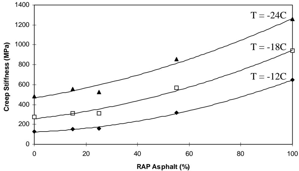
Figure 3.7 Creep stiffness trend for RTFOT and PAV-aged CG blend
