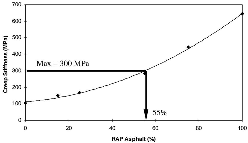
Figure 4.3 Creep stiffness trend for RTFO and PAV-aged DG blend at  $-12^{\circ}\text{C}$
