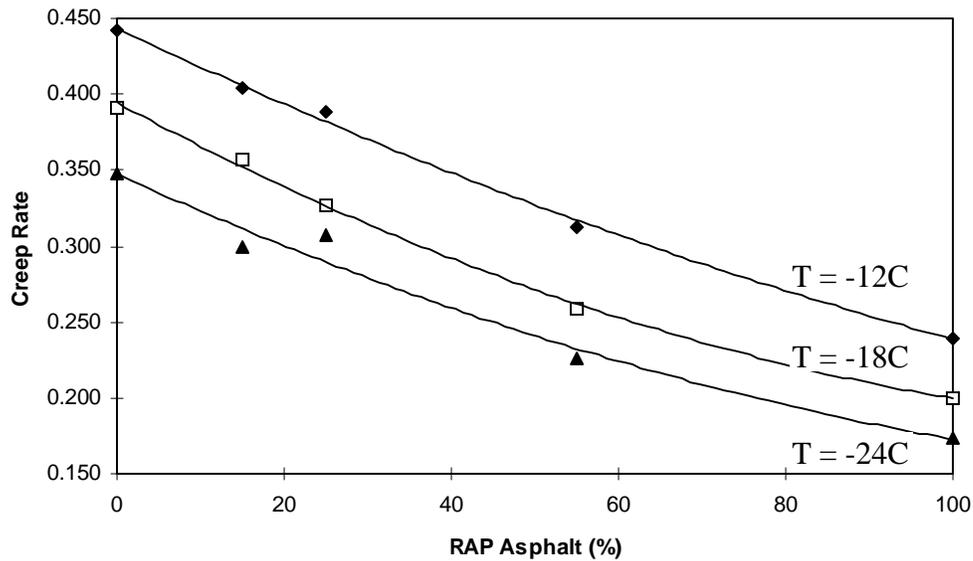
Figure 3.10 Creep rate trend for RTFOT and PAV-aged AF blend
