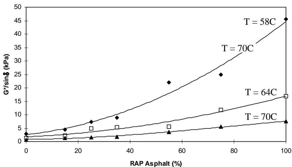
Figure 3.2  $G^*/\sin\delta$  trend for unaged MF blend
