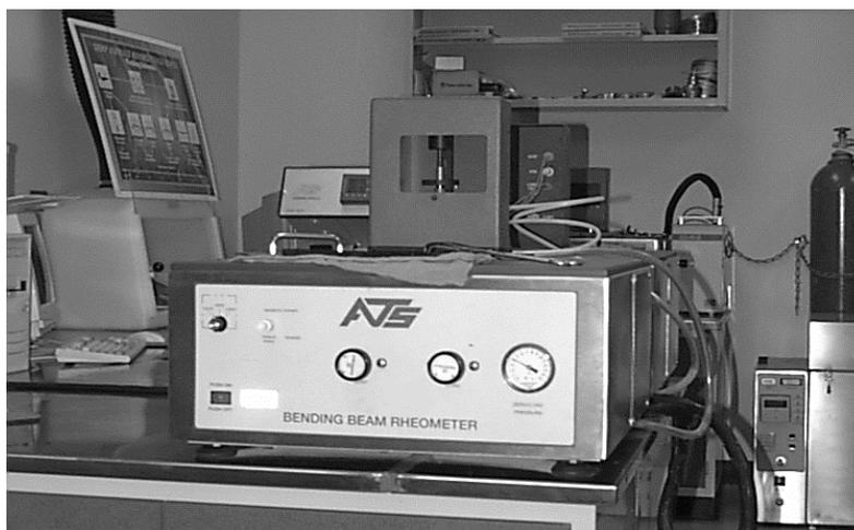
*Figure 2.5 Bending beam rheometer*
