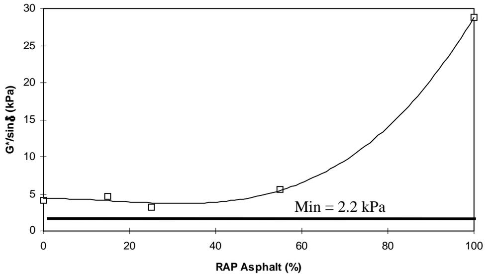
Figure 4.2  $G^*/\sin\delta$  trend for RTFOT-aged DG blend at 64°C
