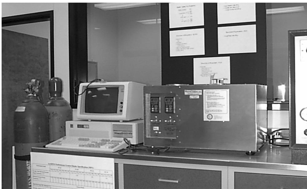
*Figure 2.2 Pressure Aging vessel*
