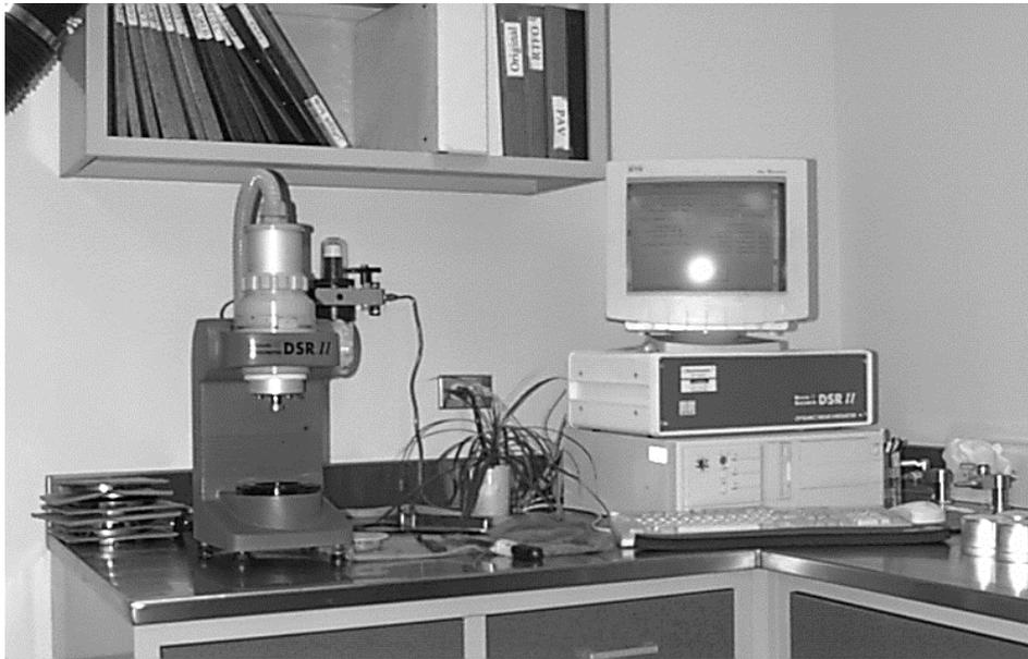
*Figure 2.3 Dynamic shear rheometer*
