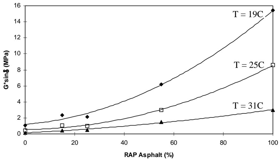
Figure 3.6  $G^* \sin \delta$  trend for RTFOT and PAV-aged AF blend
