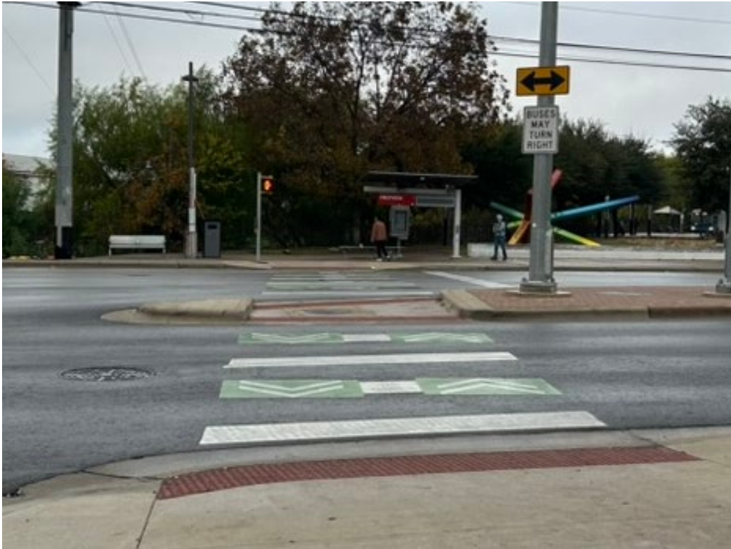
Figure 28. An example of a pedestrian refuge island at an intersection in Austin, Texas (taken: N Lamar Blvd & Airport Blvd, December 2024).
