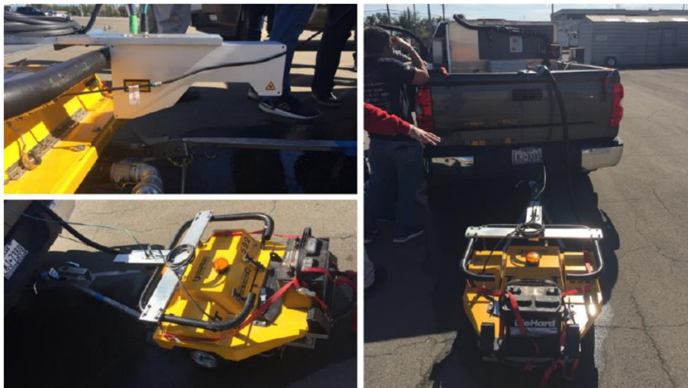
Figure 48: Original data collection prototype to measure pavement surface profiles at high speed and predict pavement surface.
