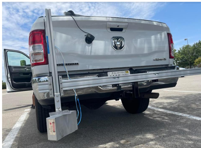
Figure 49: New data collection prototype to measure pavement surface profiles at high speed and predict pavement surface.
