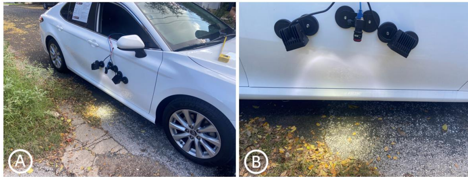
Figure 60: Part (A), camera and lighting system magnetically mounted to the passenger side of the vehicle. Part (B), close-up of the camera in the middle and two spot-lights focusing the light at the center area of where the images are being captured.
