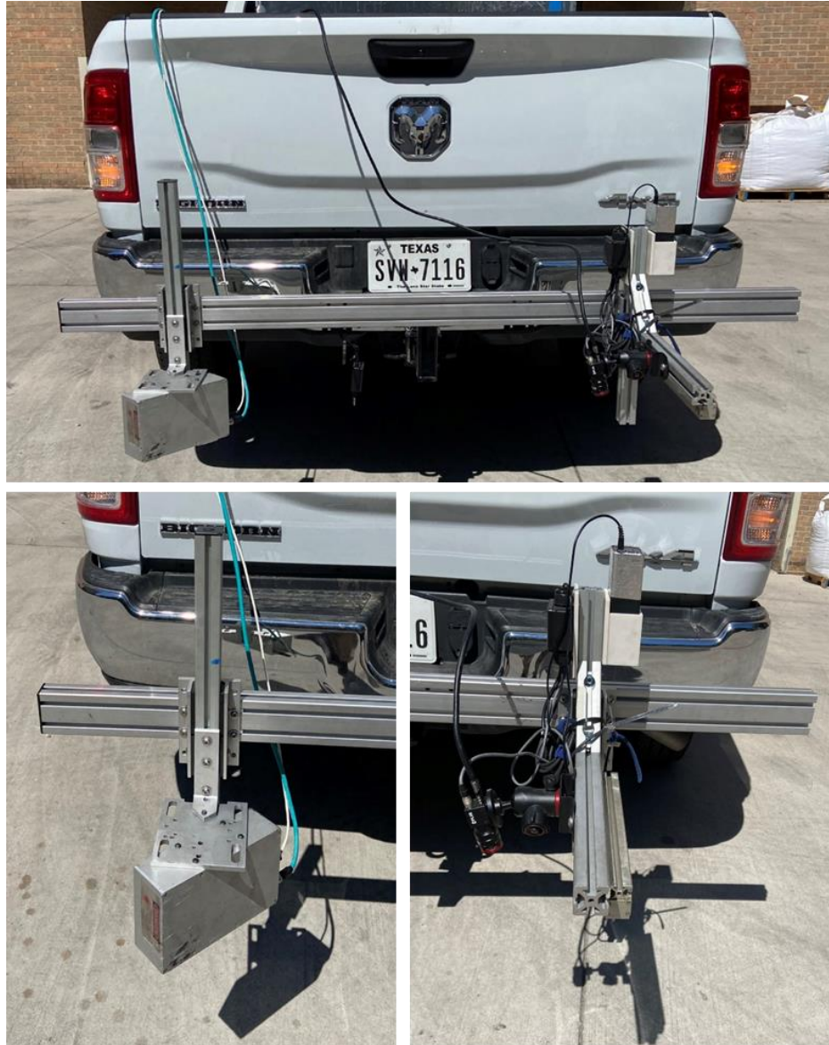
Figure 63: System mounted onto vehicle shown on the top; line laser sensor shown on the bottom-right; and camera and light system (perpendicular to the main beam), shown on the bottom left.
