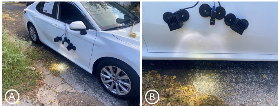
Figure 50: (A) Prototype magnetically mounted to the passenger side of the vehicle. (B) Close-up of the camera in the middle and two spot-lights focusing the light at the center area of where the images are being captured.
