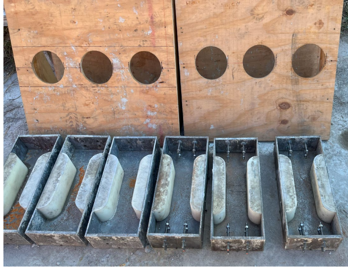
Figure 4-5 Metal molds for dog-bone specimens
