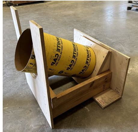
(b) Wood stand for 12×24-in. cylinder
