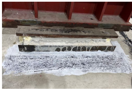
(a) Speckle pattern on the testing region
