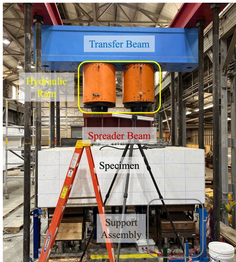
Figure 6-15 Test setup for drilled-shaft footing cap specimen
