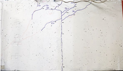
(a) Specimen photo at 50 kips
