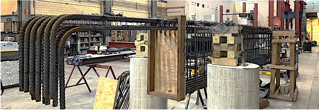
Figure 5-15 Steel cage of III-1.85-00-V and III-1.85-00-V-R with wooden stopper in between the interior and the exterior section
