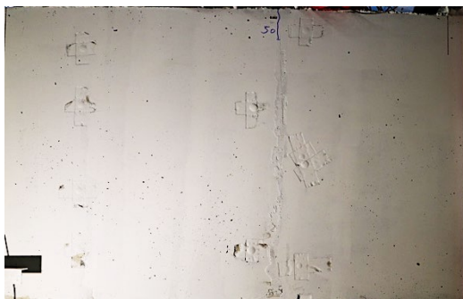
(a) Specimen photo at 50 kips
