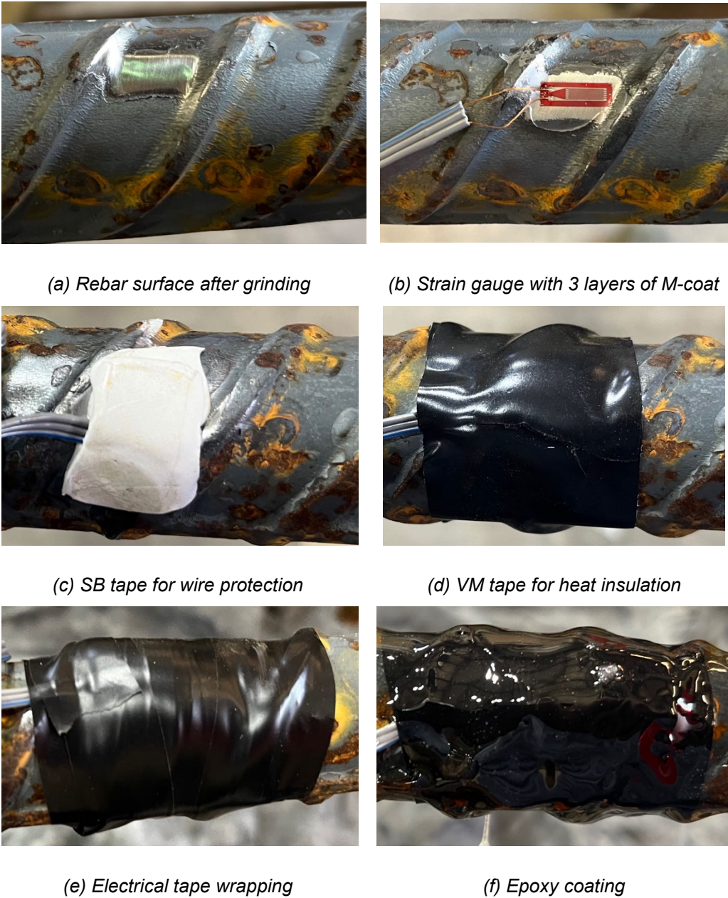
Figure 5-13 Strain gauge installation
