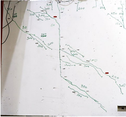
(b) Specimen photo at 350 kips
