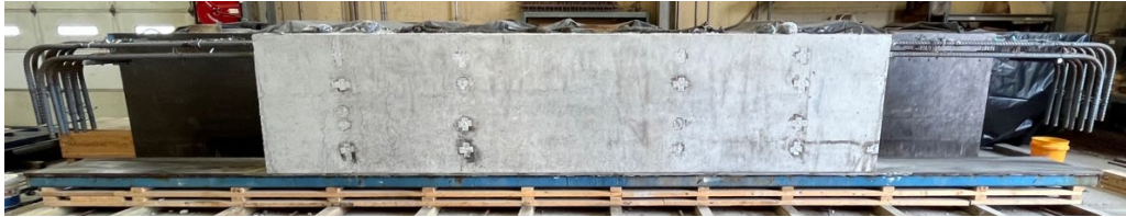
(b) Concrete cast in the interior section
