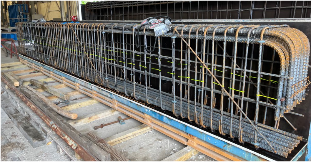
Figure 5-14 Steel cage of I-1.85-03-H and I-1.4-03-H
