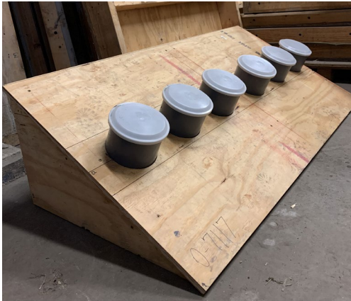
(a) Wood stand for 6×12-in. cylinders
