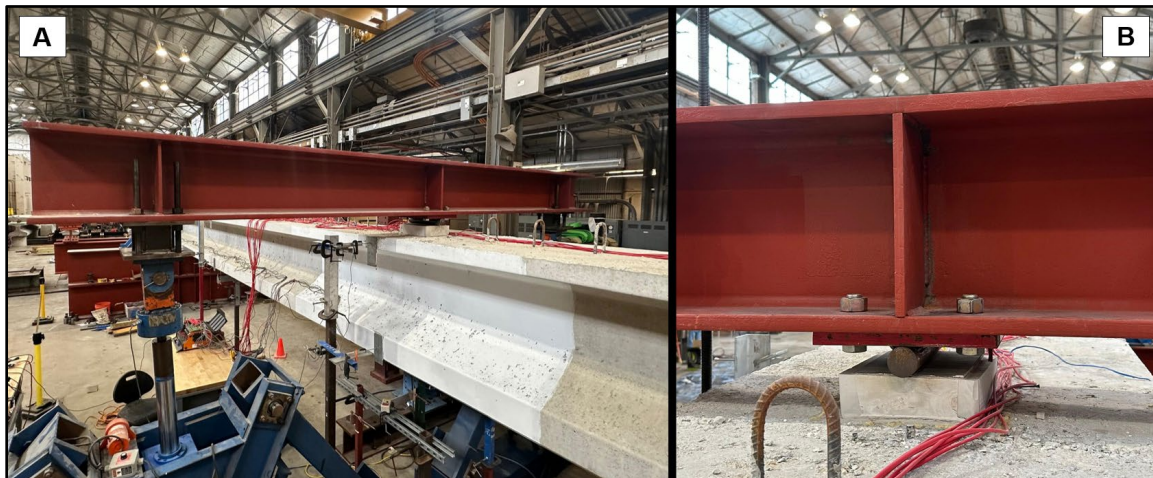
Figure 3.50. (A) Concentric loading setup at midspan (B) Load application via round bar on steel plate embedded in hydrostone
