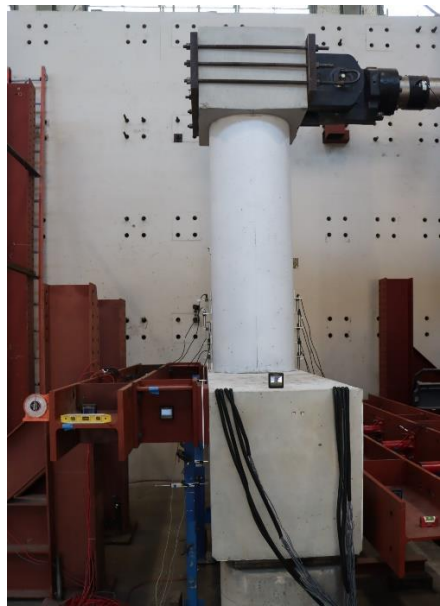
(b) HD-O-CIP in the test frame
