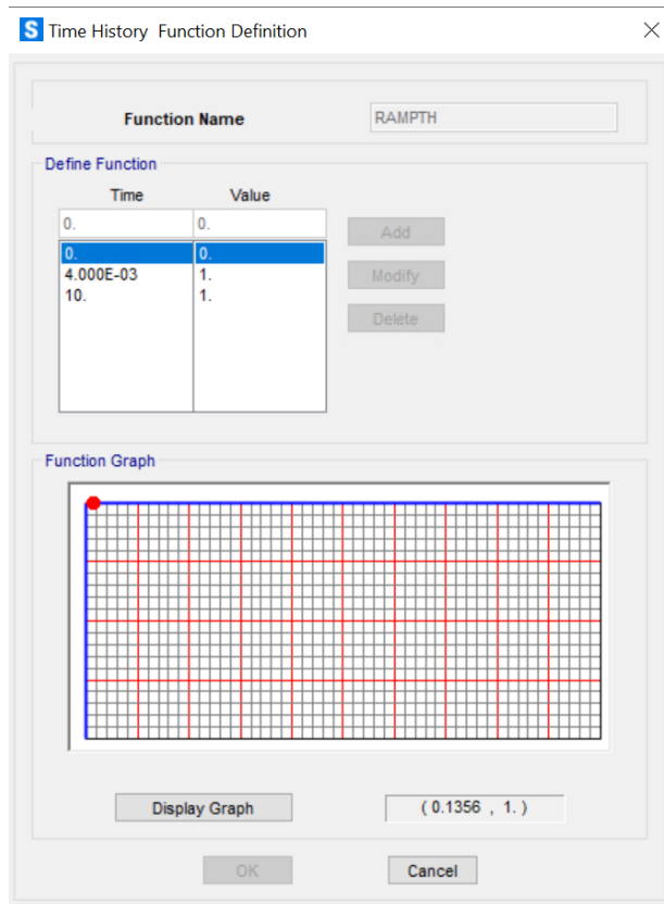
Figure 3-38. Definition of ramping function
