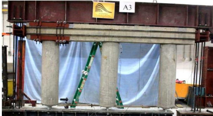
Figure 2-28. Retrofitted specimen with external prestressing along the cap and transverse prestressing at one external joint by Vasseghi et al. (2015)
