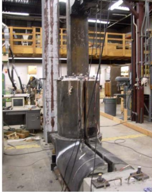
Figure 2-25. A specimen with elbow-shaped steel jacketing around the beam and joint (McLean and Shattarat (2005))
