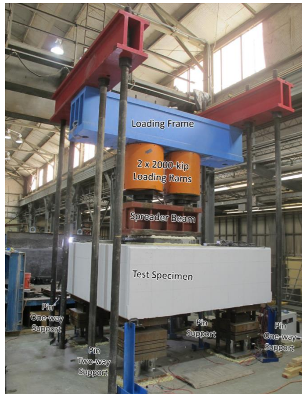
Figure 3-80. Test setup for drilled shaft footing specimens
