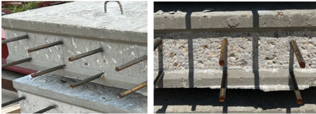
Figure 4.9 & Figure 4.10 Shear Key Surface Profiles Before (Left) and After (Right) Surface Roughening
