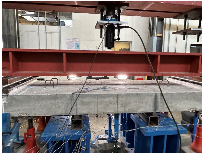
Figure 4.16 Monolithic Control Specimen in Flexure Test Setup
