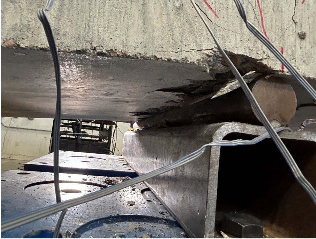
Figure 4.43 Non-proprietary Specimen Crushing
