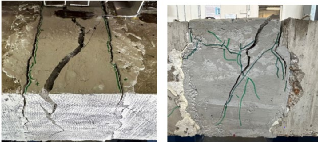
Figure 4.27 & 4.28 Proprietary mix closure joint at failure (left) & non-proprietary closure joint at failure (right)
