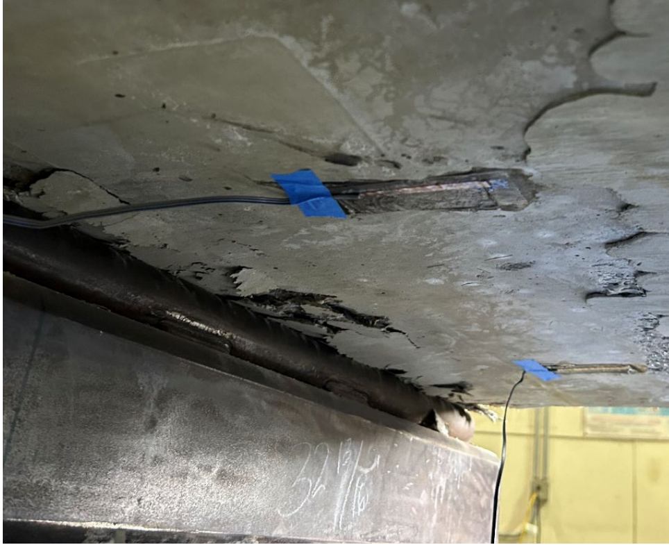
Figure 4.29 Proprietary Mix Crushing
