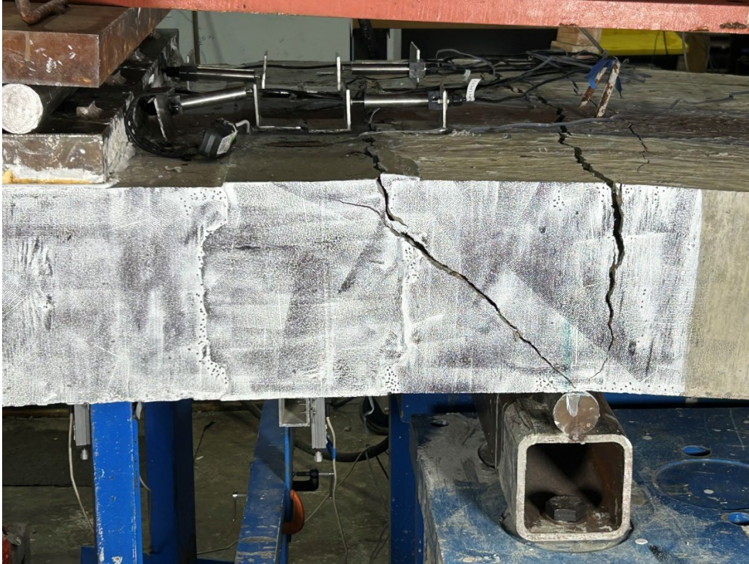
Figure 4.42 Non-proprietary Specimen at Failure
