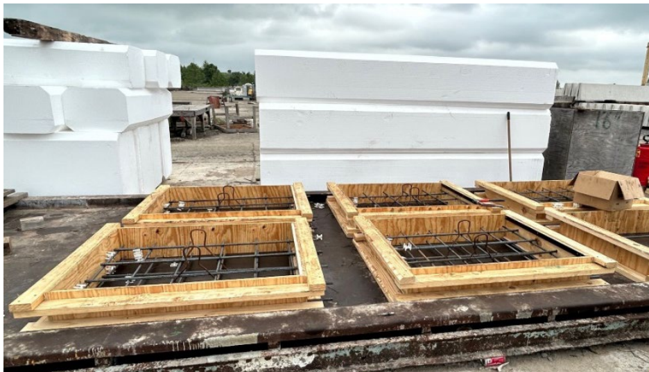
Figure 4.6 Closure Joint Deck Specimens Prior to Cast
