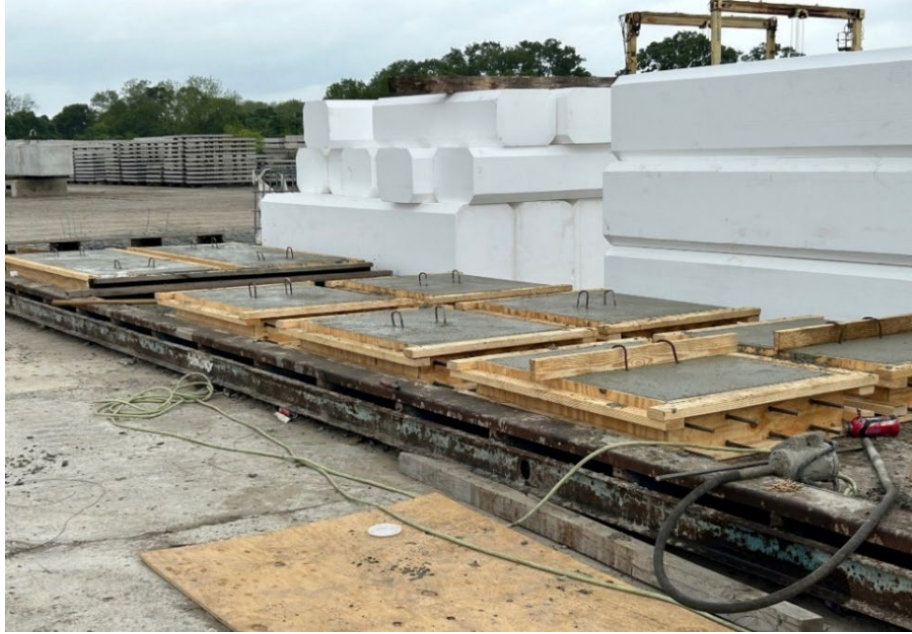
Figure 4.7 Closure Joint and Control Specimens Post Cast
