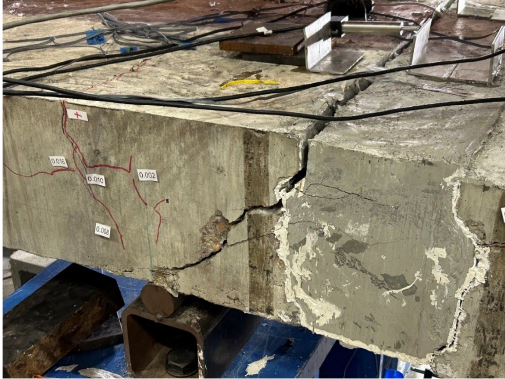
Figure 4.37 Nonproprietary Specimen at Failure
