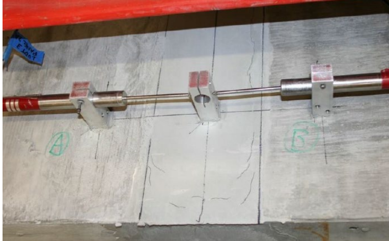
Figure 2.11 Shrinkage Cracking in UHPC Specimen (Haber & Graybeal, 2018)
