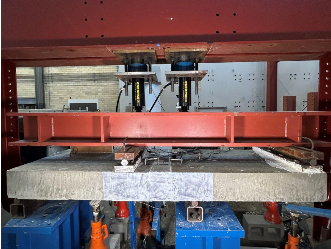
Figure 4.18 UHPC Closure Joint Specimen in Shear Test Setup
