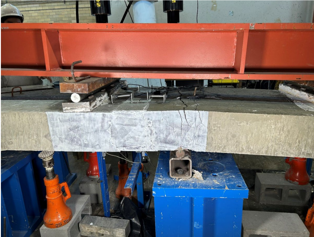
Figure 4.36 Proprietary Specimen at Failure
