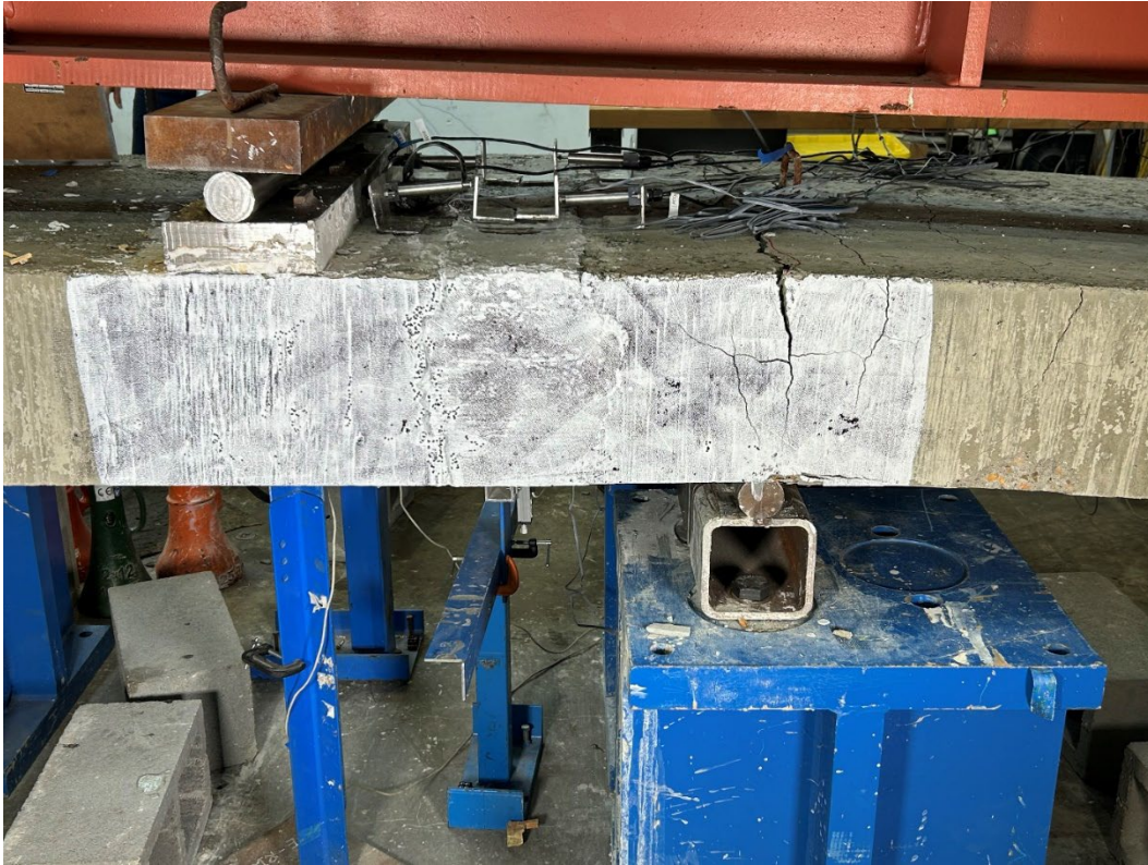
Figure 4.40 Proprietary Specimen at Failure
