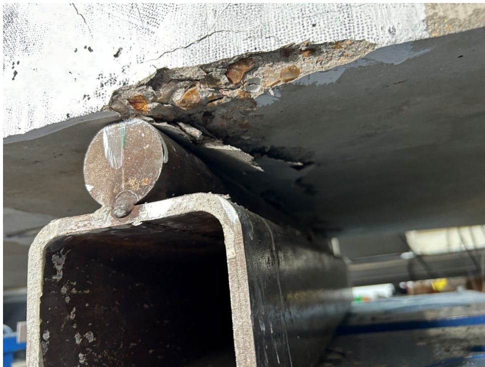
Figure 4.41 Proprietary Specimen Crushing
