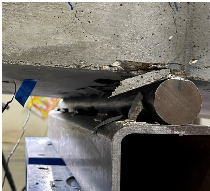
Figure 4.26 Control Specimen Crushing
