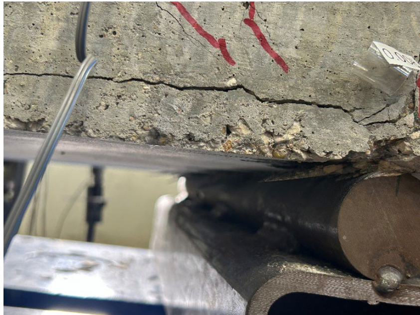
Figure 4.34 Control Specimen Crushing
