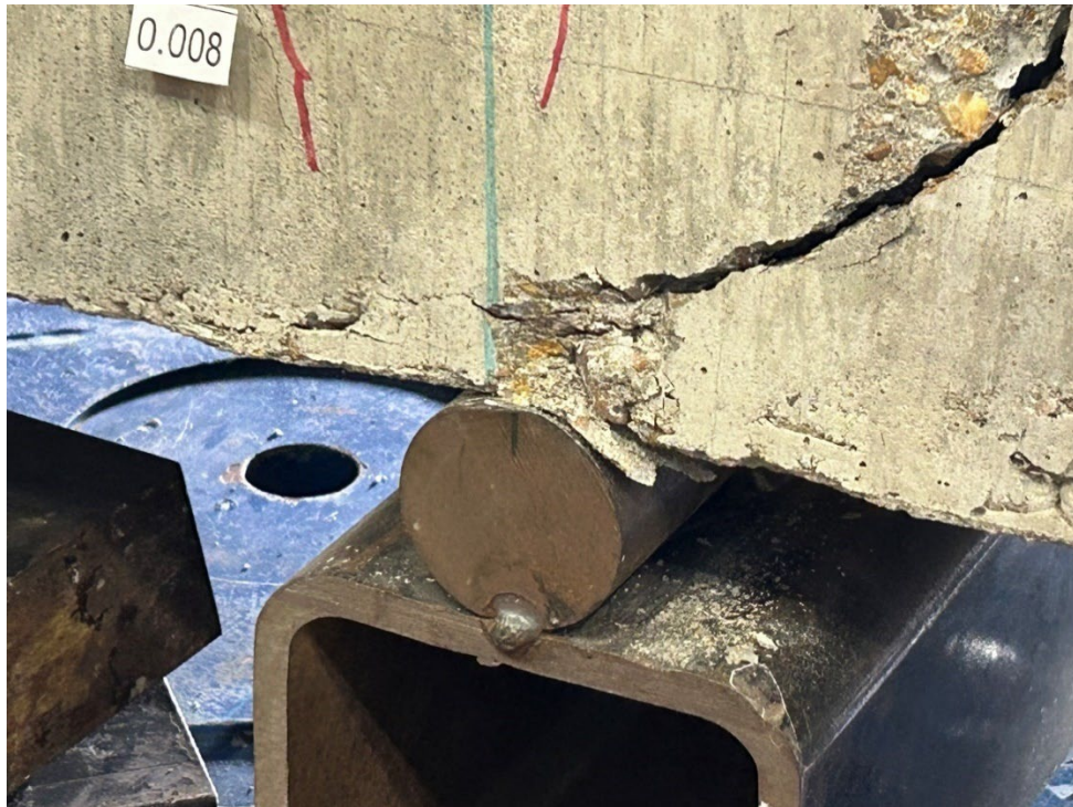
Figure 4.38 Support of Nonproprietary Specimen at Failure
