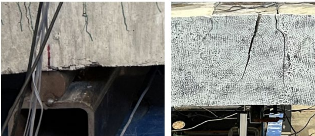
Figure 4.30 & 4.31 Non-Proprietary mix closure joint at failure (left) & (right)
