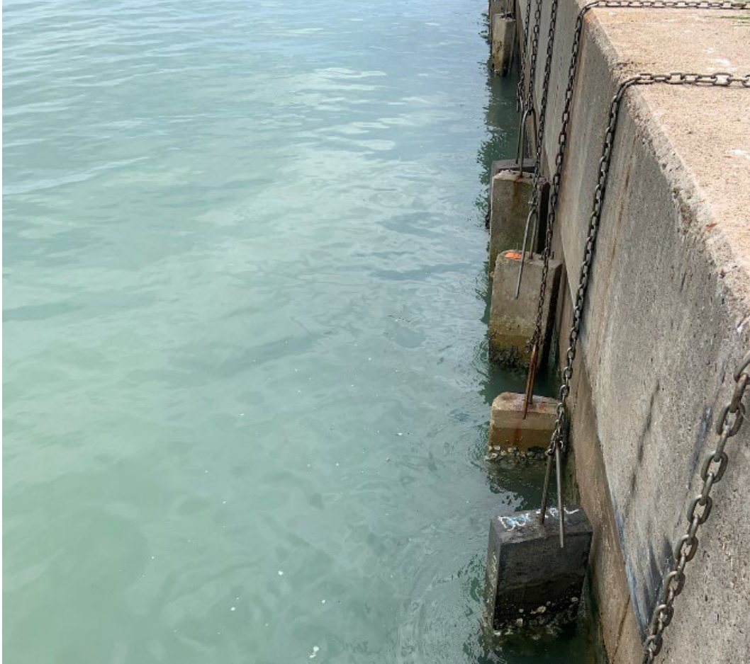
Figure 3.16 Marine Exposure Blocks for Chloride Induced Corrosion Testing
