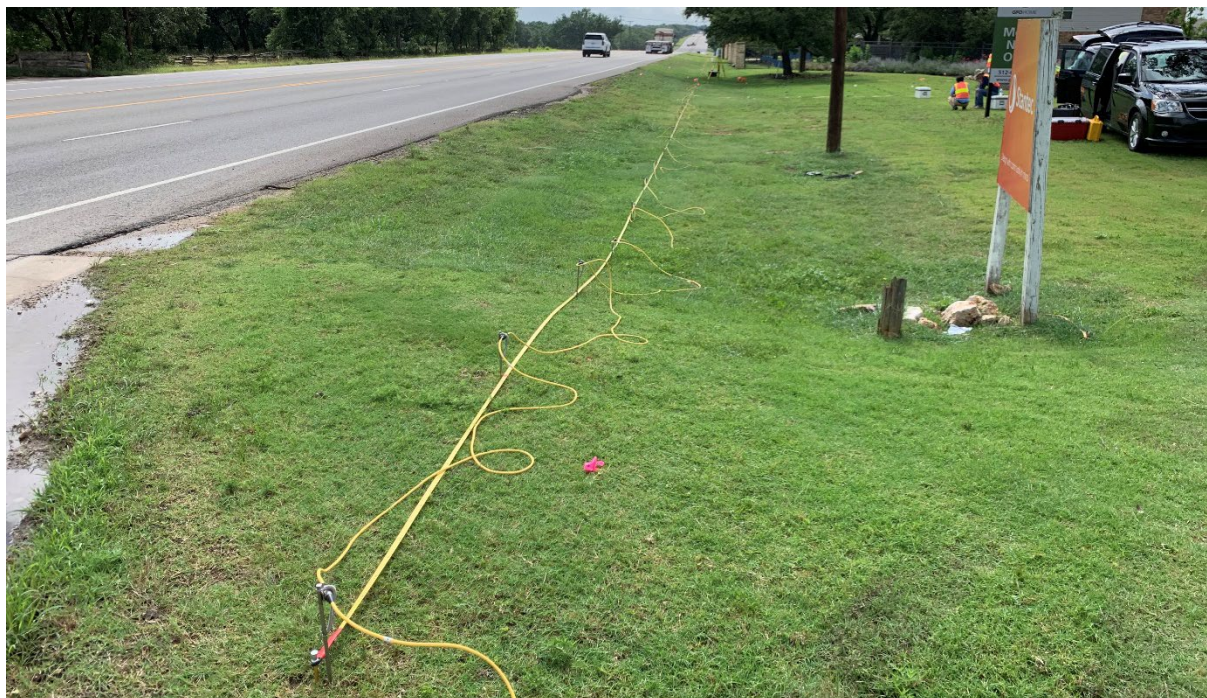
Figure 4.4: Typical ERT line showing electrodes and their connectivity (line X).
