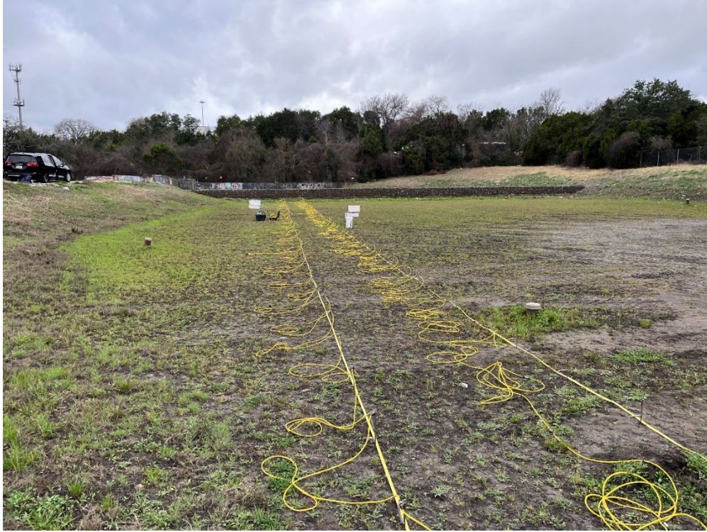
Figure 4.42: Picture of ERT equipment used for each Line.
