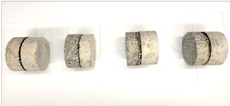
Figure 6.19. Side view from SAT IH35 cores after shear test
