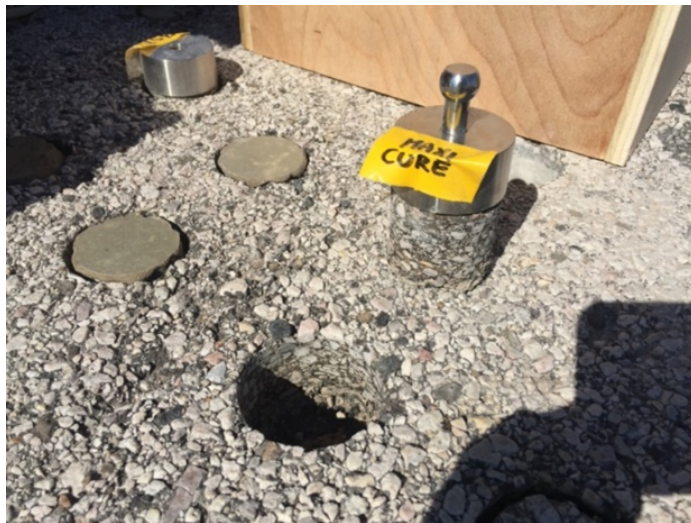
Figure 3.15. The pull-off test after completion; the figure also shows the epoxy system that was successful
