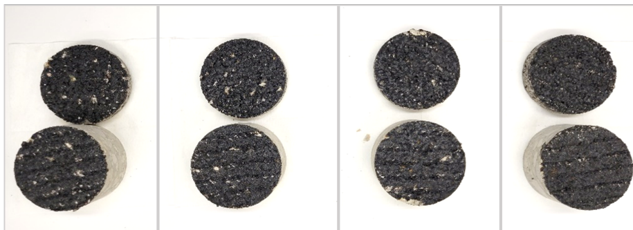
Figure 6.14. Top view from Hou IH69 cores after shear test
