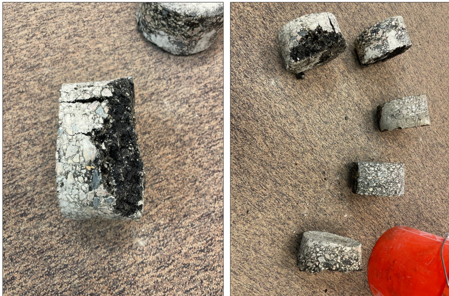
Figure 6.3. Cores from BMT US87 Beaumont district where the HMA debonded from PCC during coring
