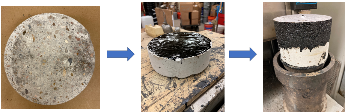
Figure 5.4. Procedure for preparation of a composite PCC-HMA sample for shear testing
