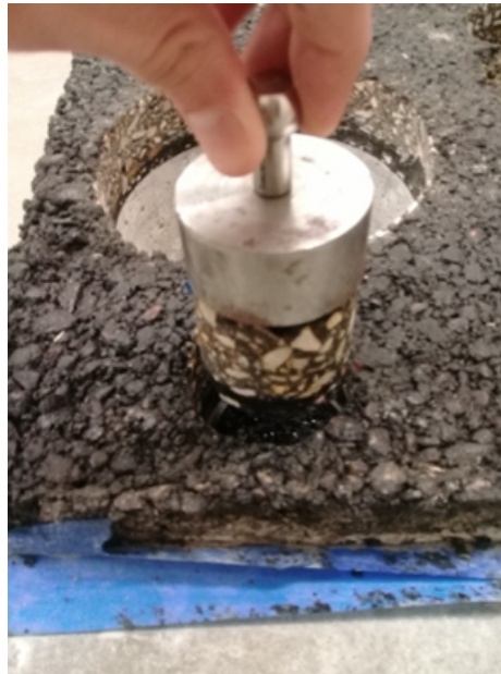
Figure 3.7. A metal plate glued to the HMA surface
