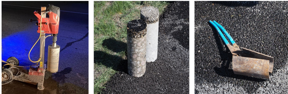
Figure 6.4. Procedure for obtaining 6-inch cores for the laboratory shear test
