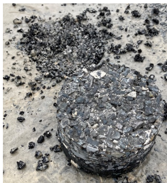
Figure 6.1. Cores from HOU SH225 with failure at the interface during coring
