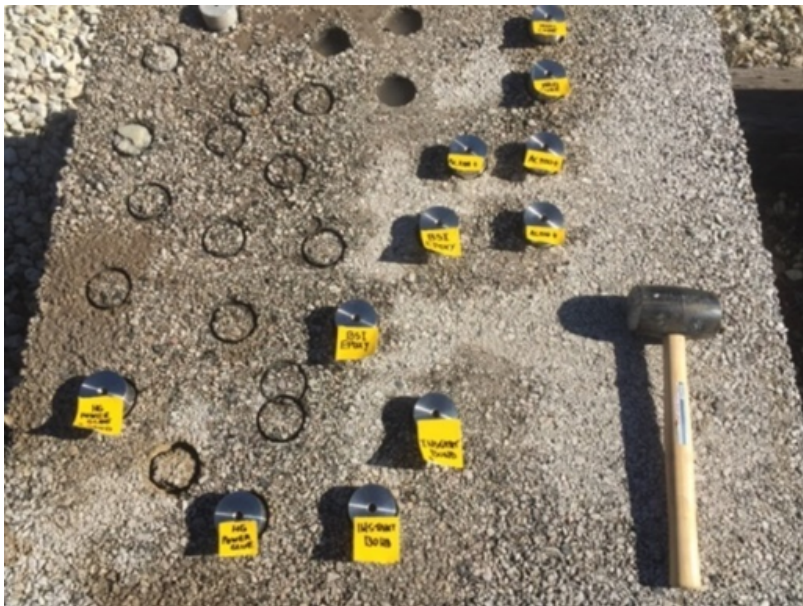
Figure 3.13. Tests conducted using multiple adhesives to determine the best adhesive for this application
