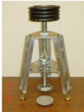
Figure 3.5. Tack coat pull-off test (TxDOT designation: Tex-243-F)
