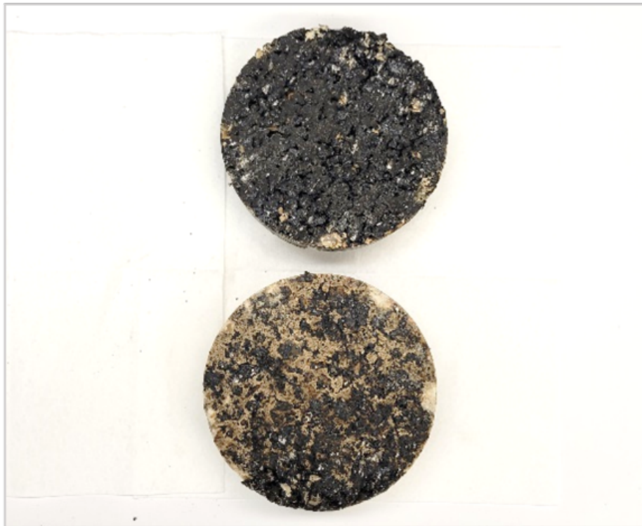
Figure 6.16. Top view from Hou SH225 core after shear test
