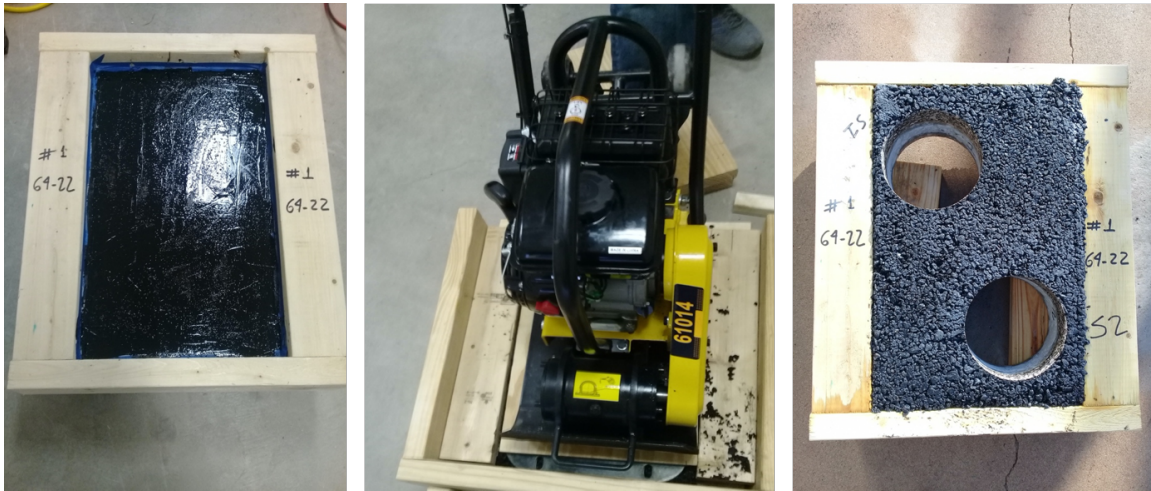
Figure 3.1. Specimen fabrication in the laboratory using a vibratory compactor
