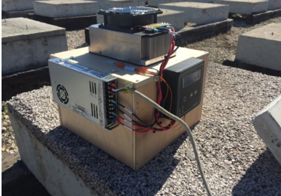
Figure 3.10. Thermoelectric temperature control system that can be used in the field
