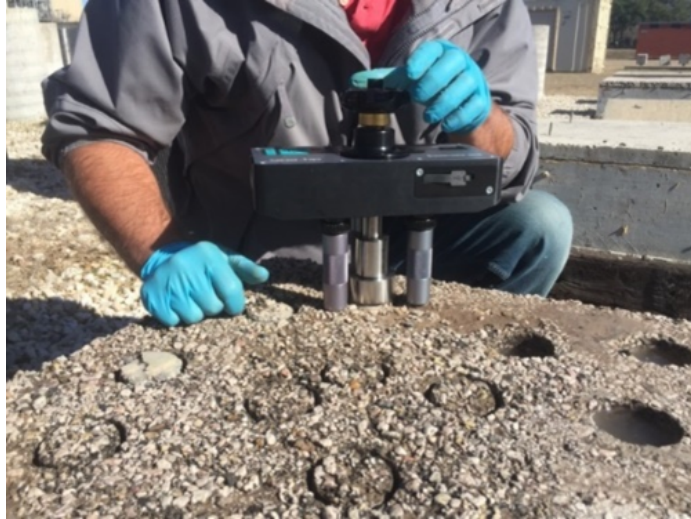
Figure 3.14. The pull-off device being locked on to the sample and the test being conducted using a force-controlled mode at a rate of 1 N/sec
