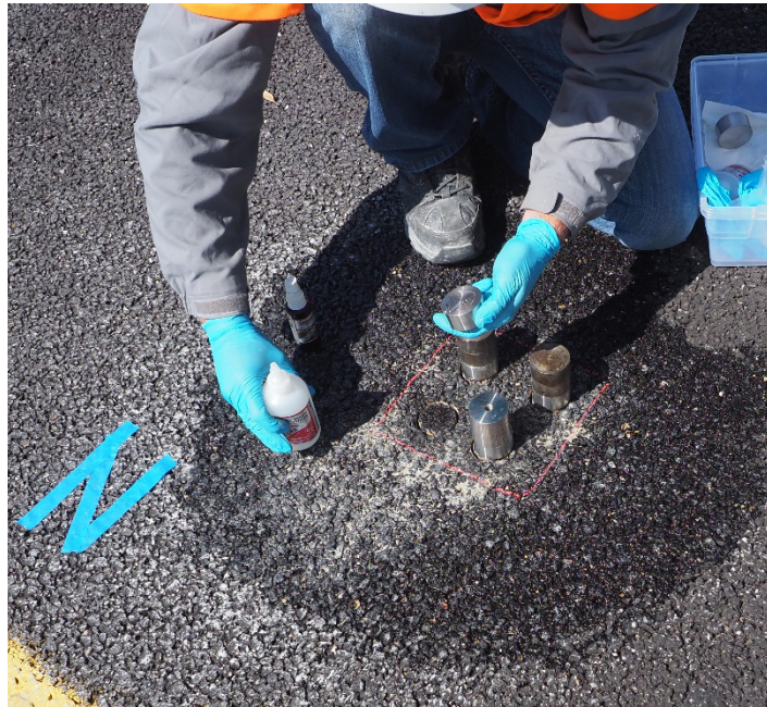
Figure 6. Applying adhesive, test stubs, and weights.
