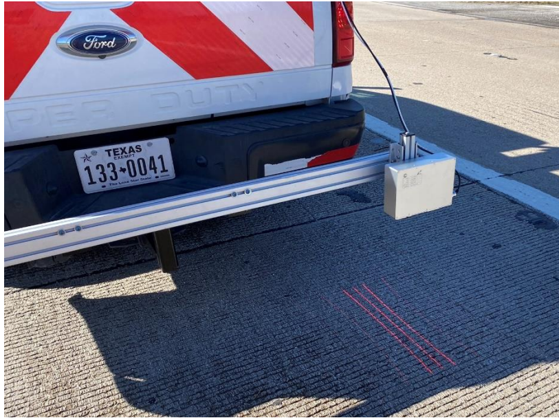
Figure 4.10 3-Line laser installed on TxDOT's profiler vehicle
