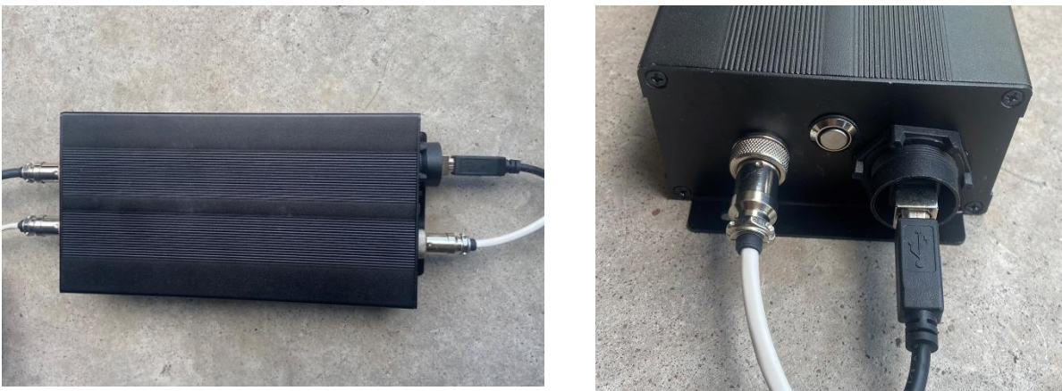
Figure 4.9 Encoder interfacing box, housing encoder counter
