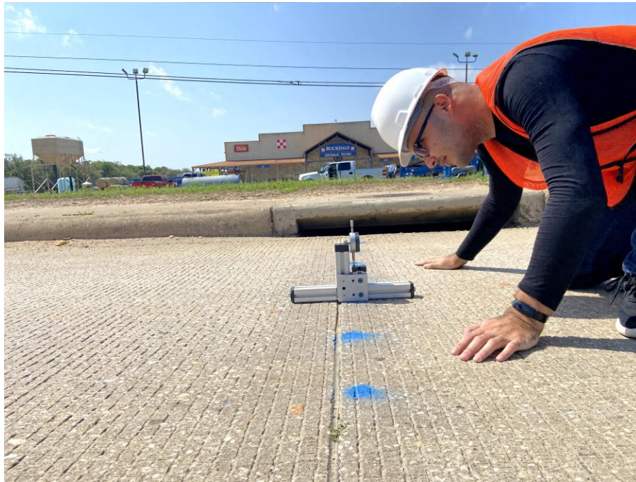
Figure 3.3 Operating the Faultmeter in Field Data Collection
