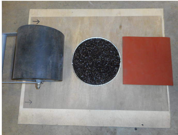
Figure 5.1. Specimen fabrication for the Sweep test.
