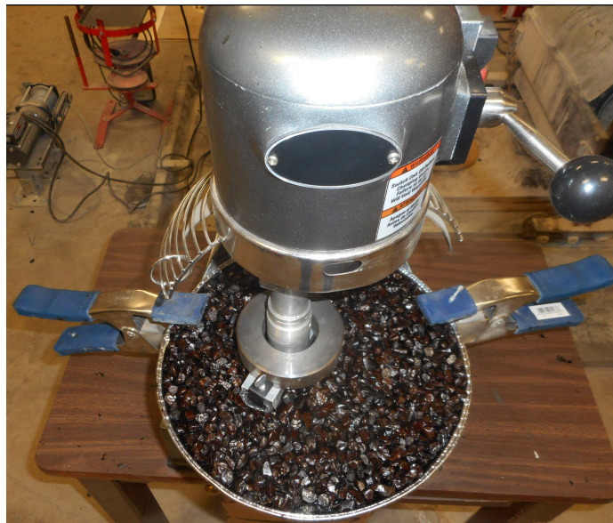
Figure 5.2. Specimen in the testing setup for the Sweep test.
