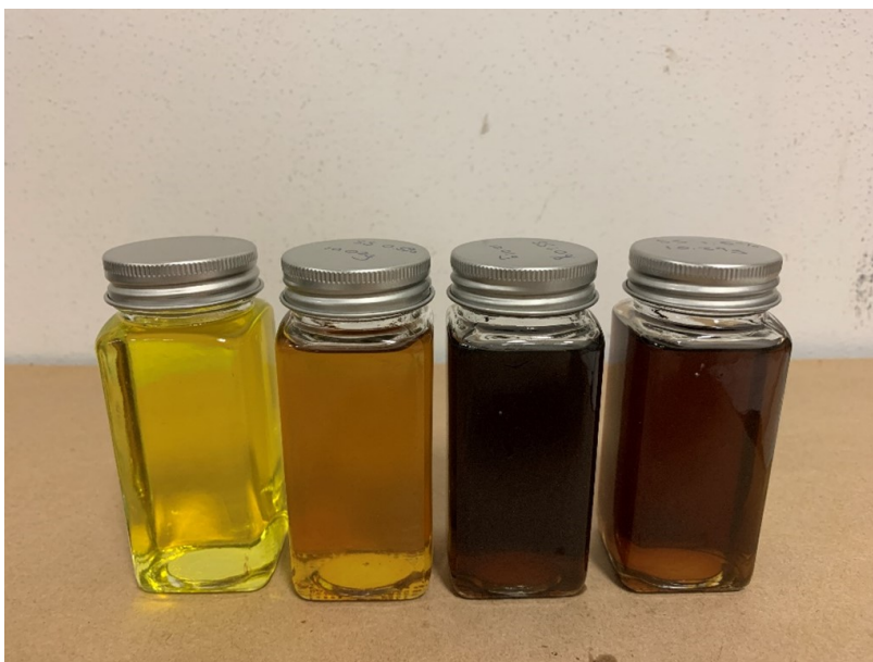
Figure 3.18. Difference in color between samples contain different percentages of binder dissolved in diesel
