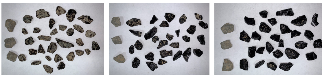
Figure 3.2. Sandstone aggregates coated with controlled amount of binder (left to right: 0.5%, 1.0%, 1.5%)
