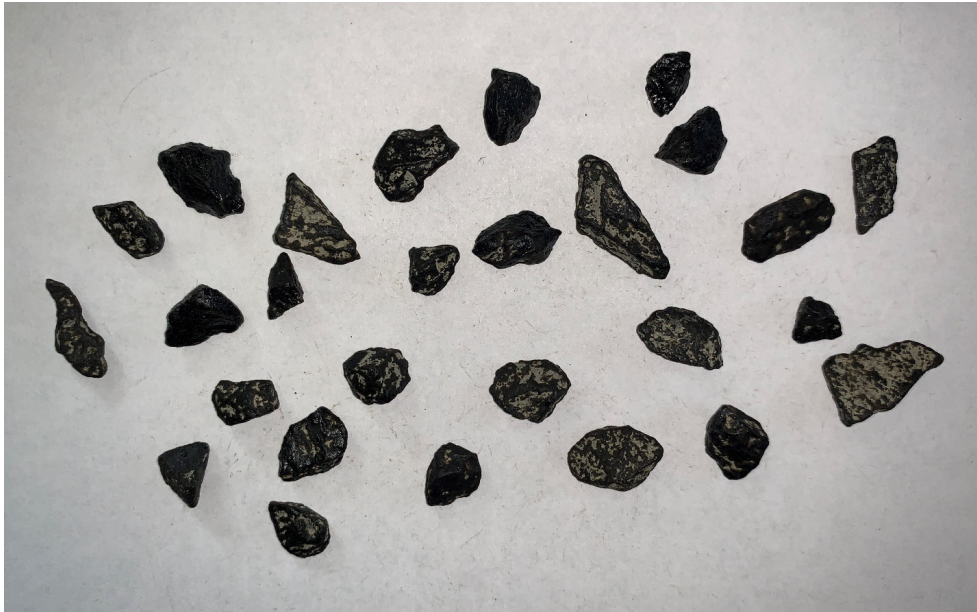
Figure 4.17. Rhyolite aggregate at 85.5% precoat (0.2% binder by weight)
