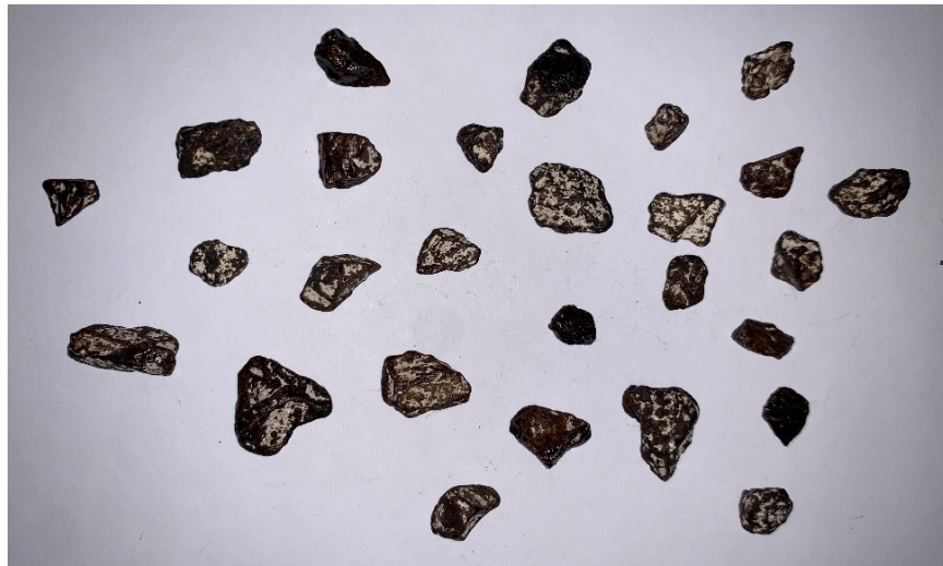
Figure 3.24. Limestone aggregate precoated in 0.4% binder by weight.
