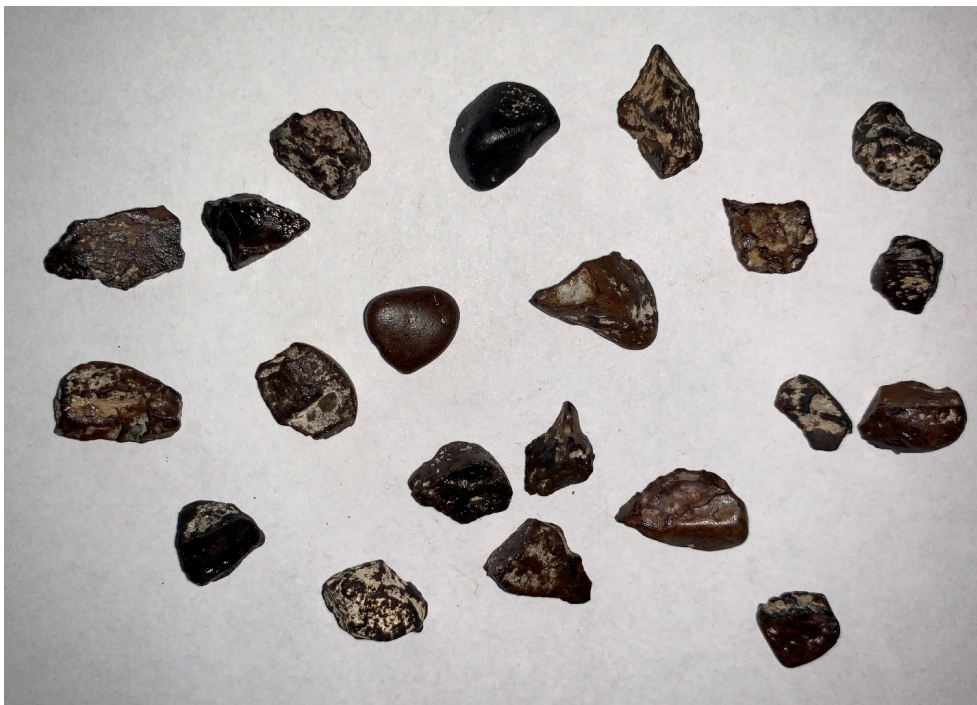
Figure 4.18. Gravel aggregate at 85.1% precoat (0.2% binder by weight)
