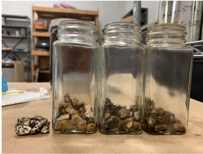
Figure 3.22. Precoated aggregates after dissolving in solvent (Diesel/Kerosene); notice that a small amount of binder did not completely dissolve.
