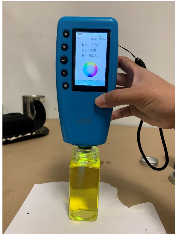
Figure 3.16. Image of a colorimeter pointed towards a diesel sample to measure color measurements
