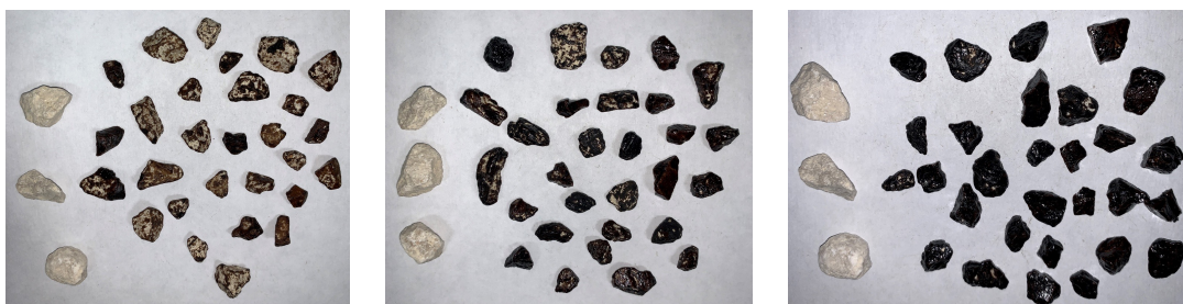
Figure 3.1. Limestone aggregates coated with controlled amount of binder (left to right: 0.5%, 1.0%, 1.5%)
