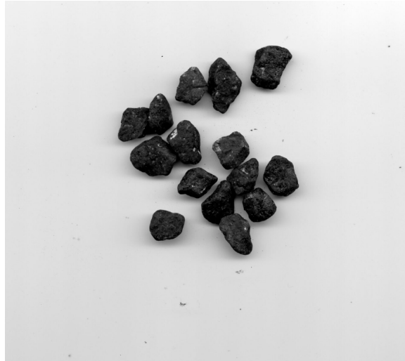
Figure 3.7. Image of pre-coated aggregate on the bed of a scanner
