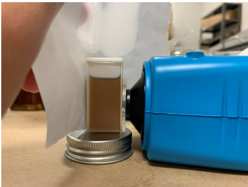
Figure 3.17. PG 64-22 mixed with diesel in cuvette; the colorimeter is used from the side and a white sheet of paper was used to reflect light back into the colorimeter sensor.
