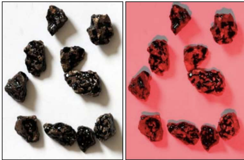
Figure 2.2. Aggregate surface before and after being examined for scatter under laser (Mulsow, 2012)
