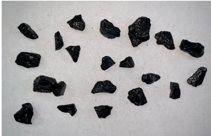
Figure 3.25. Rhyolite aggregate precoated in 0.4% binder by weight.
