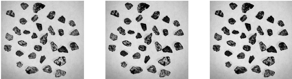
Figure 3.10. Image from Figure 3.9 split into three channels, left to right: red, green, and blue channel
