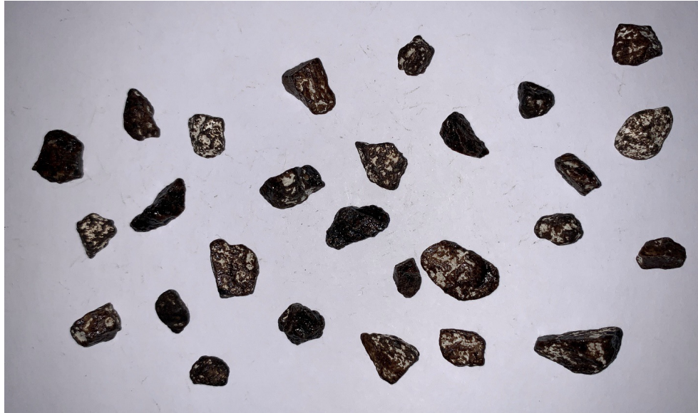
Figure 4.15. Limestone aggregate at 85.6% precoat (0.6% binder by weight)
