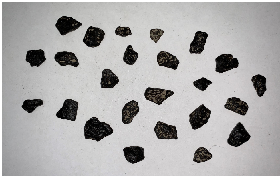
Figure 4.16. Sandstone aggregate at 85.3% precoat (0.6% binder by weight)
