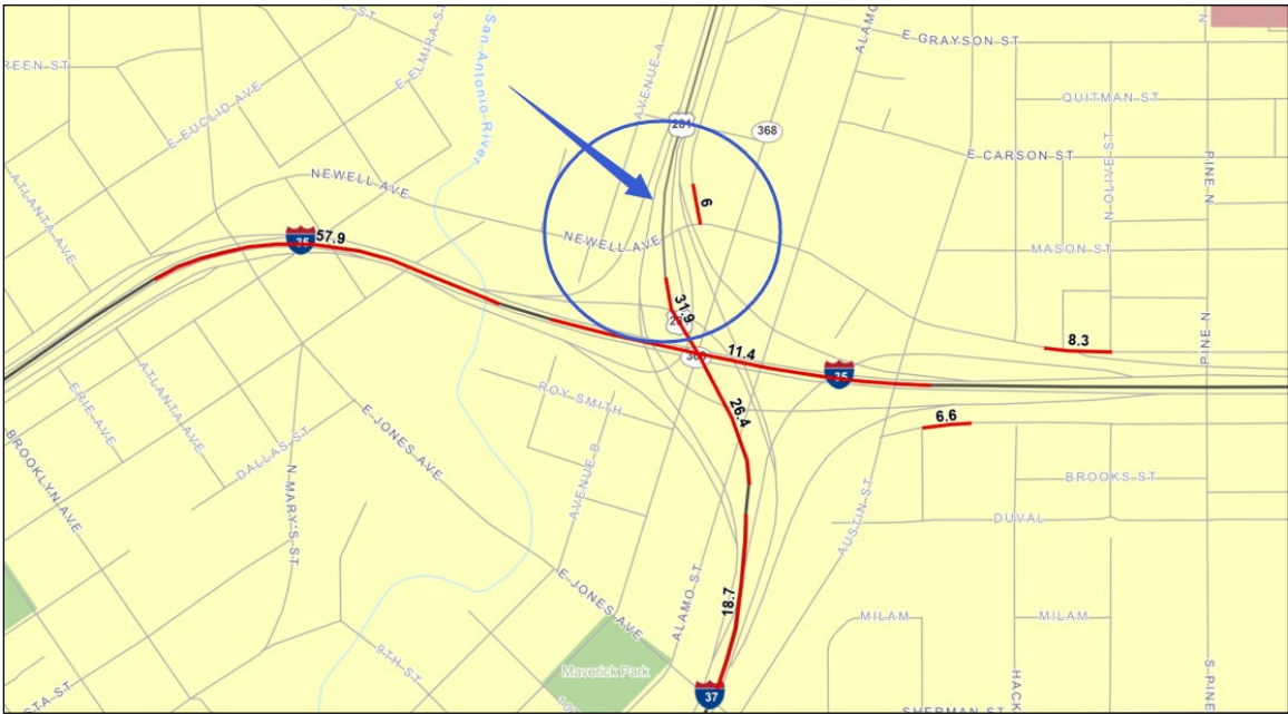
Figure 3-11. Incomplete Curves in Highway Curves GIS Layer
